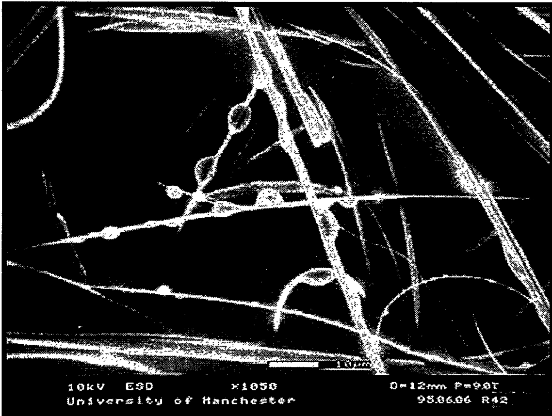
Figure 6. Water droplet formation on coalescer fibres after soaking in a clay-treated Jet A-1 fuel. Note the wide variation in droplet contact angle
