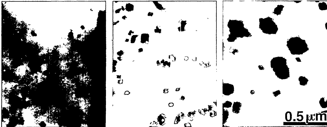
Fig. 1. TEM micrographs of oxide particles resulting from: a) 900°C extrusion, 900°C 1 hour anneal; b) 900°C extrusion, 1300°C 1 hour anneal; and c) 1100°C extrusion, 1300°C 1 hour anneal.
