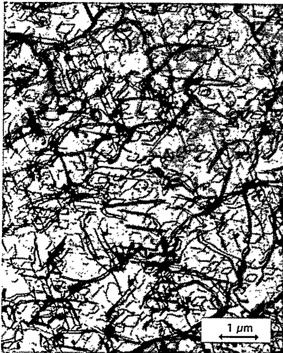
Fig. 5. TEM micrograph of FA-180 oil-quenched from a heat treatment at 1150°C and creep tested at 593°C for 6480 h.
