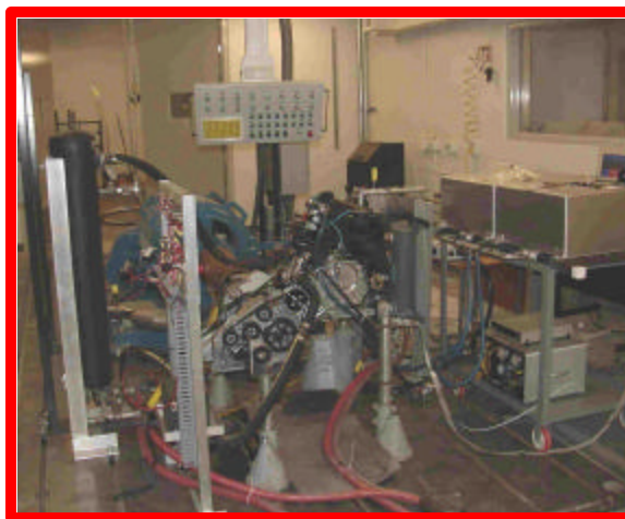
One of five typical engine research cells, this one houses a small direct-injection diesel engine with full-pass control over major engine calibration parameters
