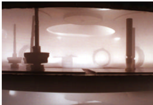
Argonne-developed near-frictionless carbon coating is produced in a high-vacuum chamber.
