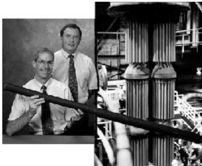
Fig. 3.1. Ceramic composite hot gas candle filters can be used to remove particulates from gas streams in combined cycle fossil and biomass power facilities. The filter is made up of an oxide fiber structure into which silicon carbide is deposited by a chemical vapor infiltration process.
