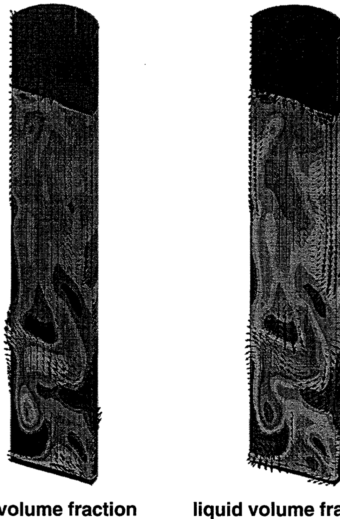
Figure 3. Los Alamos CFDLIB calculation of bubble-column flow (Kumar et al., 1995b).
