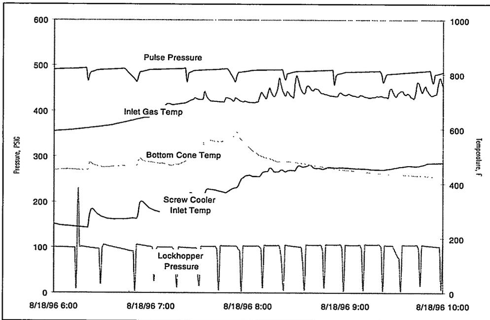
Figure 6.1.15-6 Bottom of PCD Cone Filled With Ash
