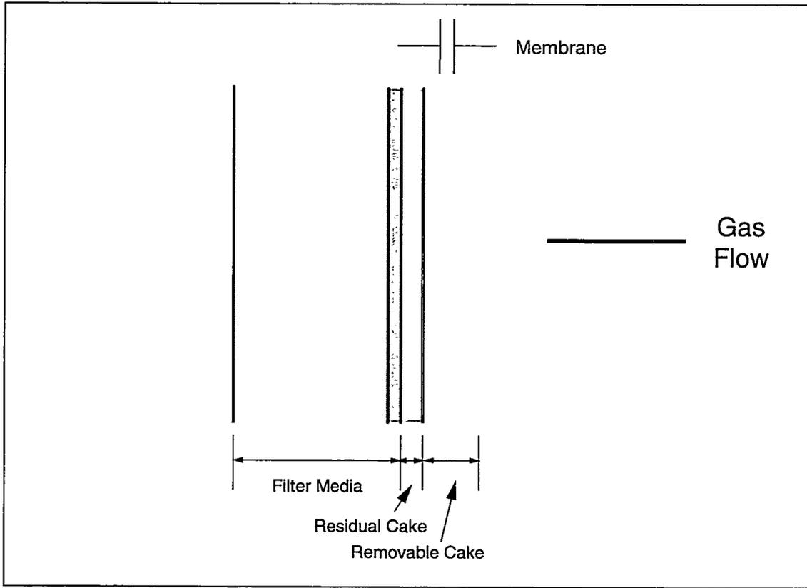
Figure 6.1.14-1 Resistances to Gas Flow
