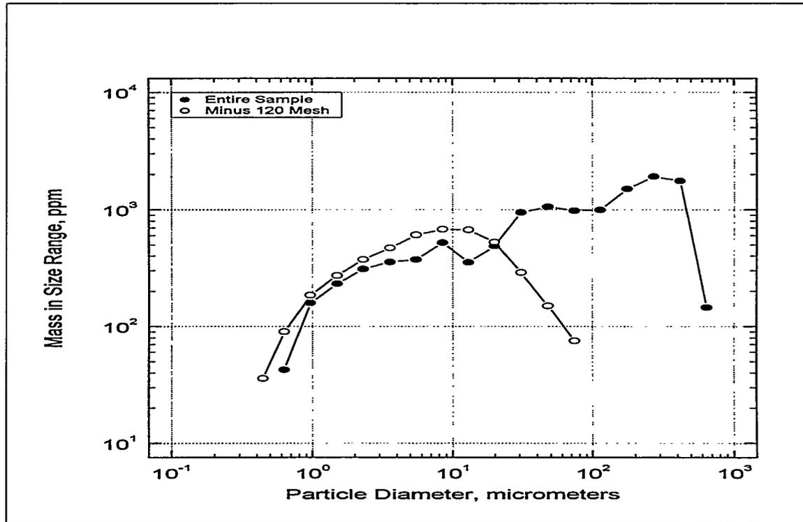
Figure 6.1.12-5 Comparison of Microtrac Measured Size Distributions for Complete Sample and Particles Smaller Than 120 Mesh
