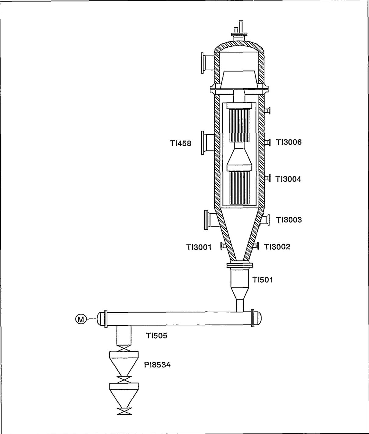
Figure 6.1.15-1 PCD/Ash Removal Instrumentation
