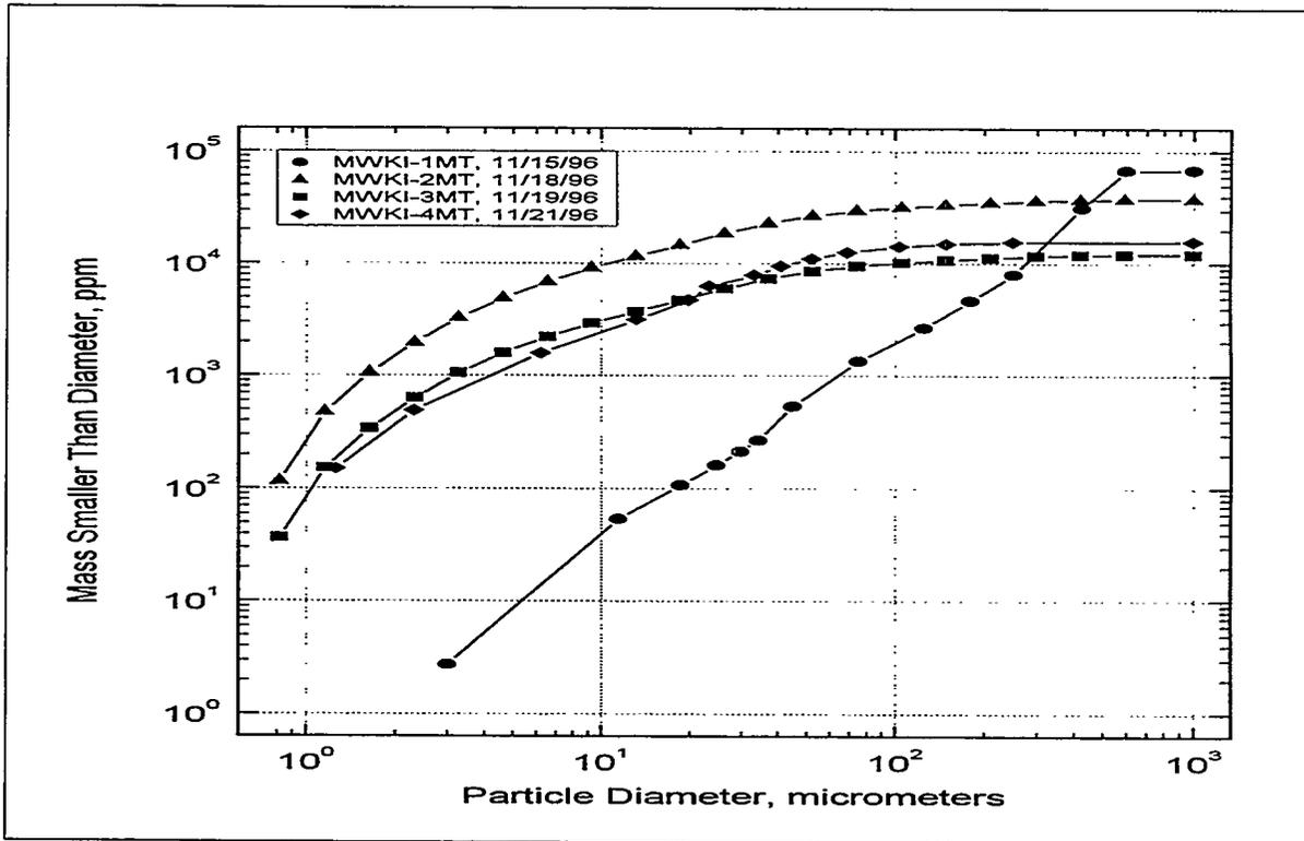
Figure 6.1.12-7 Comparison of Cumulative Mass Size Distribution For All Isokinetically Collected Samples
