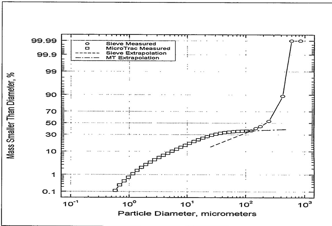
Figure 6.1.12-3 PCD Inlet Particle Size Distribution From Combined Sieve and Microtrac X-100 Measurements on In Situ Sample MWKIMT-3
