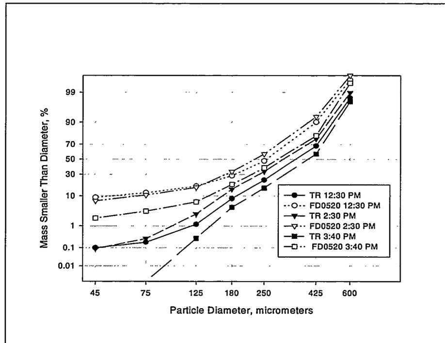
Figure 6.1.13-3 CCT3 Hopper Particle Size Distribution - December 1996 (Reactor Solid Separation Efficiency Tests 1, 2, and 3)
