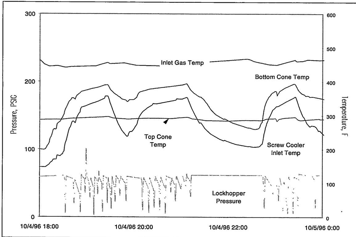
Figure 6.1.15-3 Excessive Carryover to PCD
