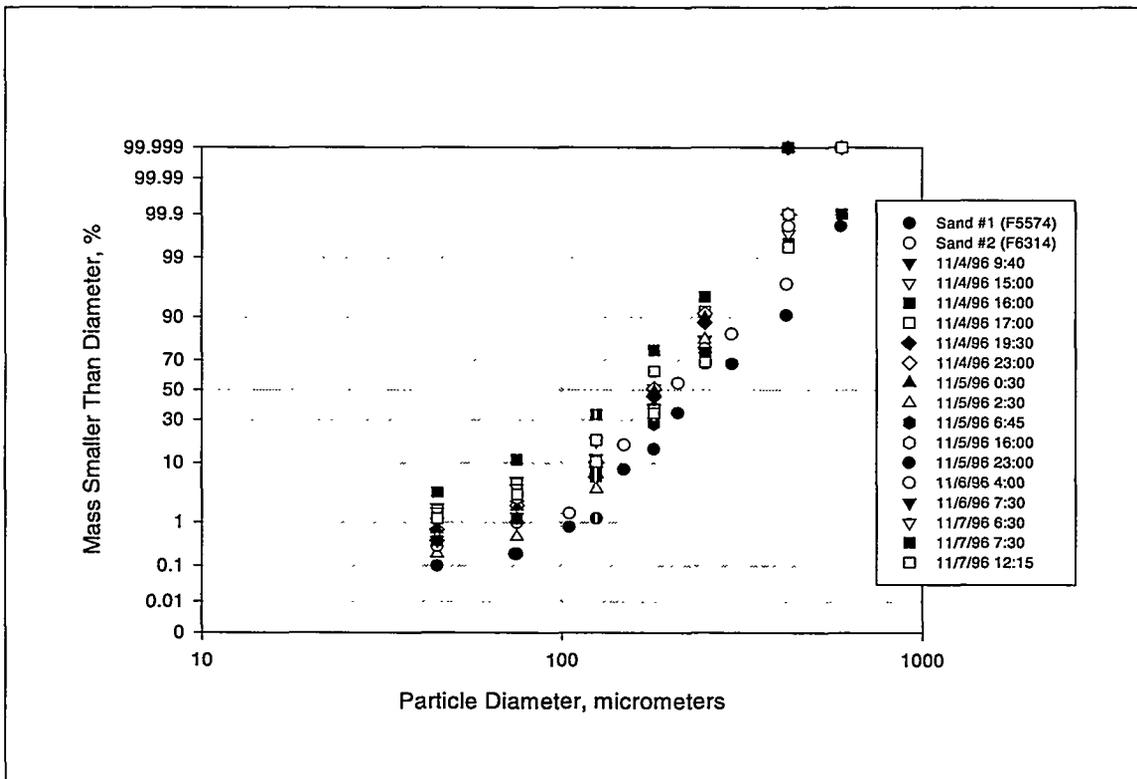
Figure 6.1.11-4 CCT2B Hopper Particle Size Distribution
