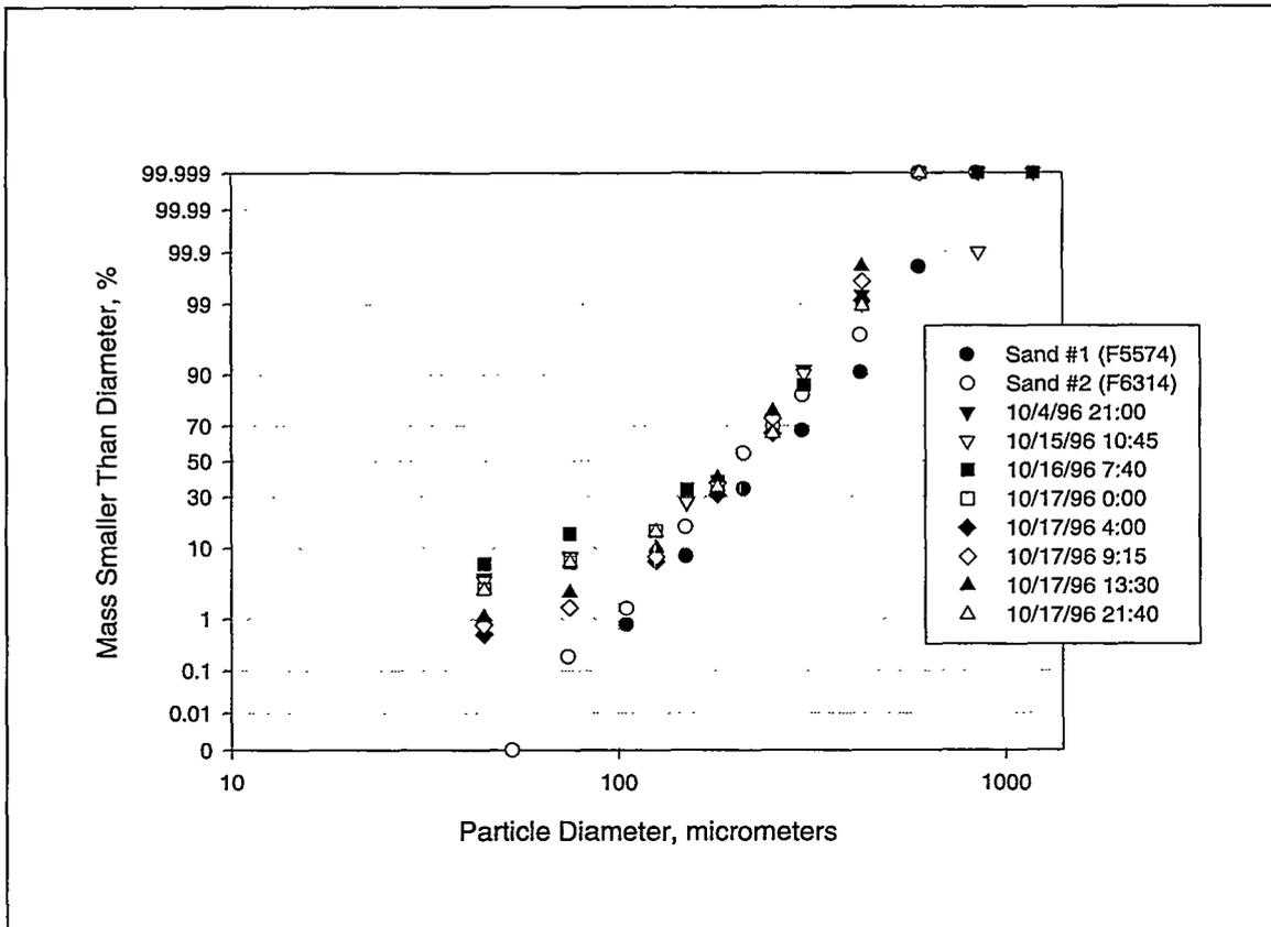
Figure 6.1.10-7 CCT2A PCD Hopper Particle Size Distribution
