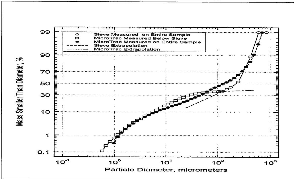
Figure 6.1.12-4 Microtrac Alone and Combined Sieve and Microtrac Measurements
