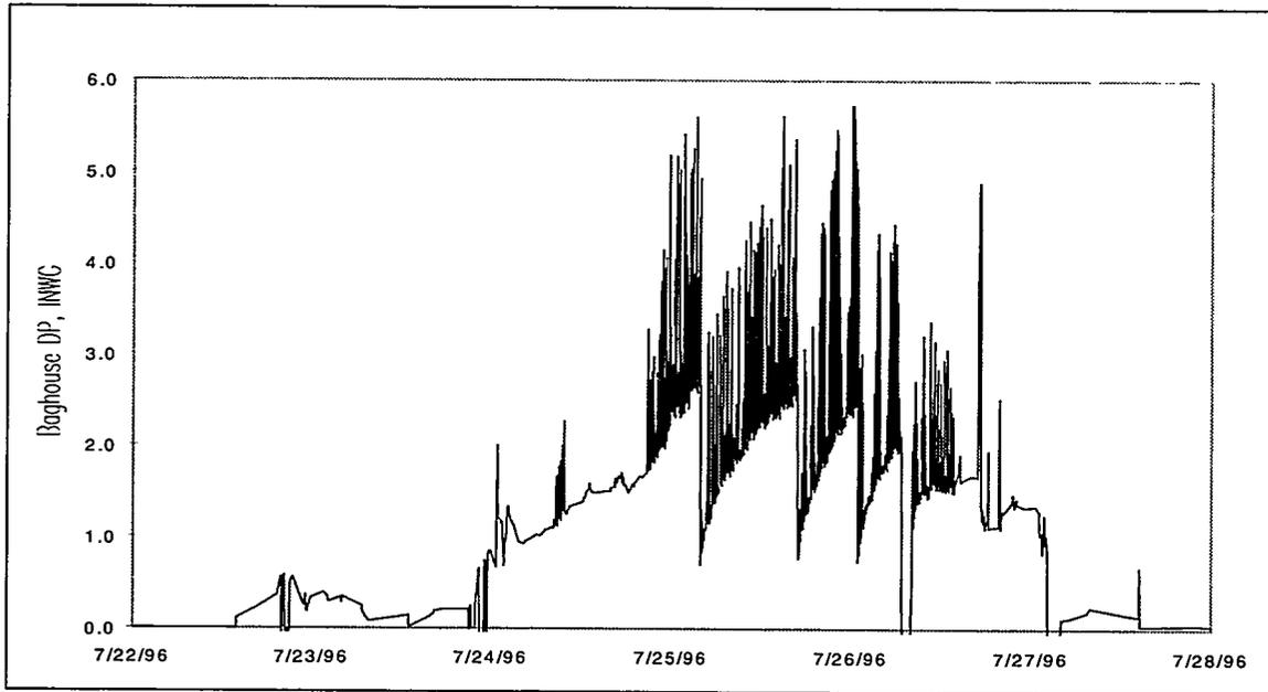
Figure 6.1.6-5 CCT1A Baghouse Differential Pressure
