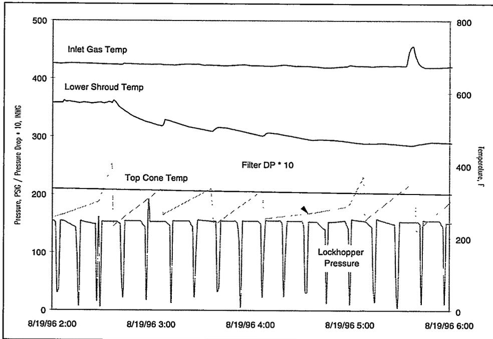
Figure 6.1.15-8 Lower Shroud Filled With Ash
