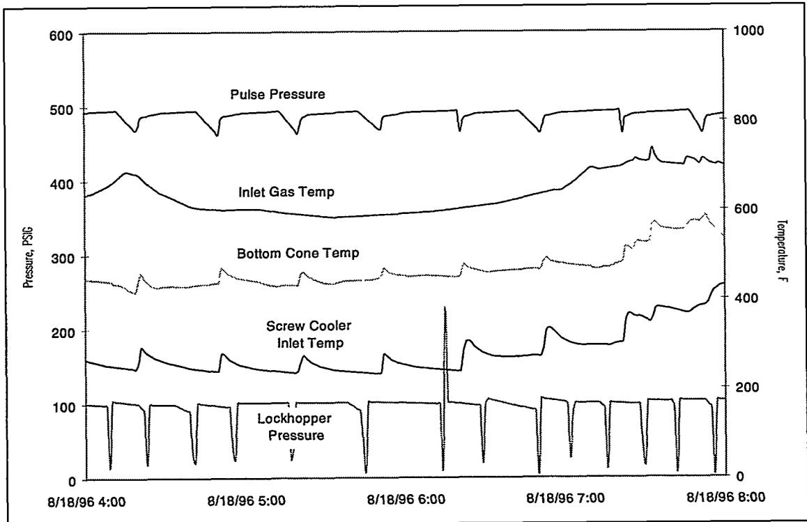
Figure 6.1.15-5 "Normal" Operation of PCD Prior to Filling
