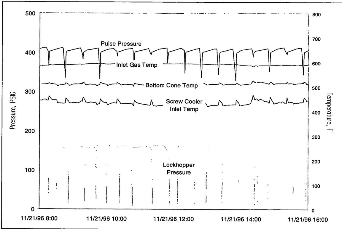
Figure 6.1.15-2 Normal PCD Operation
