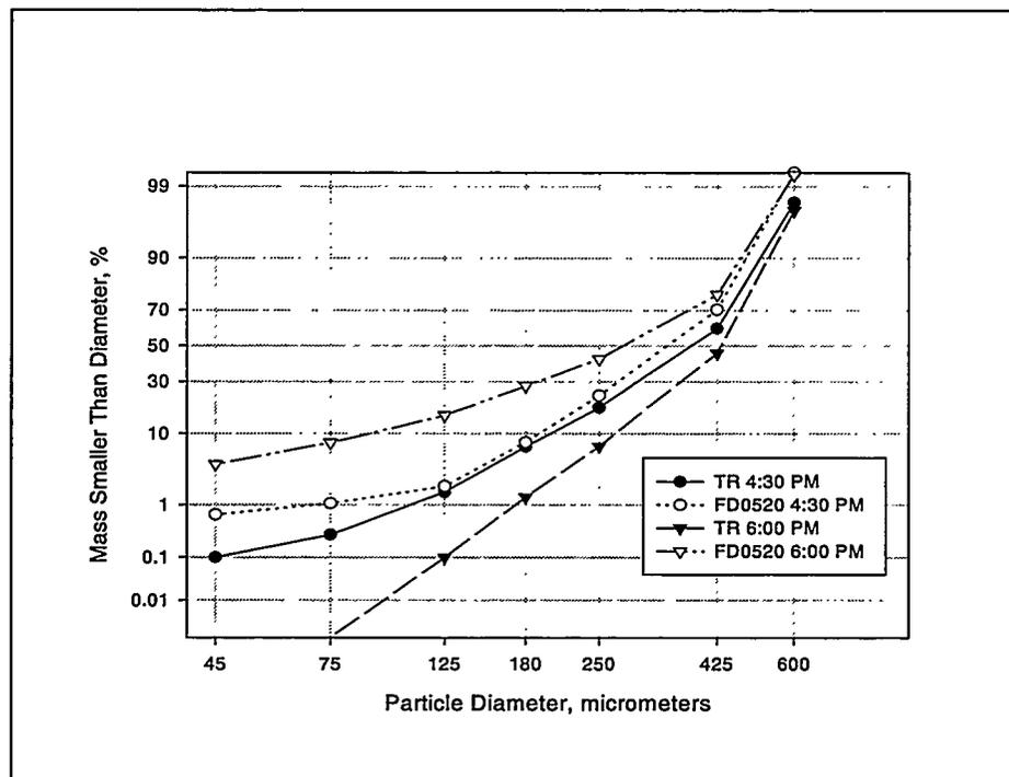
Figure 6.1.13-4 CCT3 Hopper Particle Size Distribution - December 1996 (Reactor Solid Separation Efficiency Tests 4 and 5)
