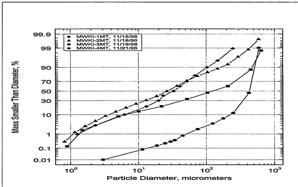
Figure 6.1.12-6 Comparison of Cumulative Percent Particle Size Distributions for All Isokinetically Collected Samples
