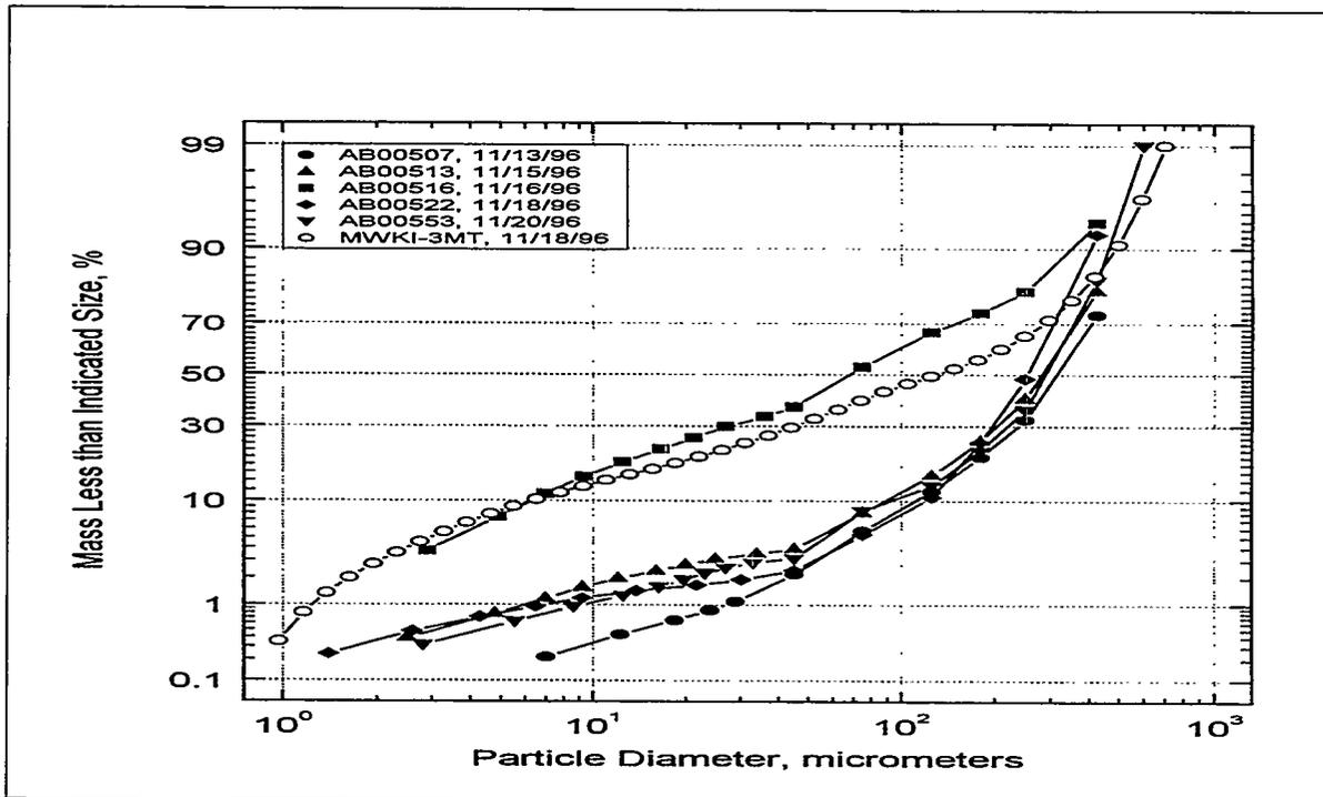
Figure 6.1.12-8 Comparison of Size Distributions From PCD Inlet In Situ Sample and PCD Cone Samples
