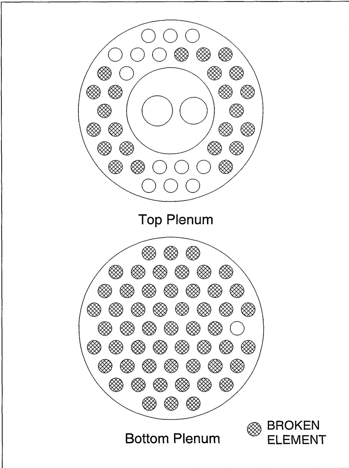
Figure 6.1.8-14 Broken Elements After CCT1C (Top of Page Is North)
