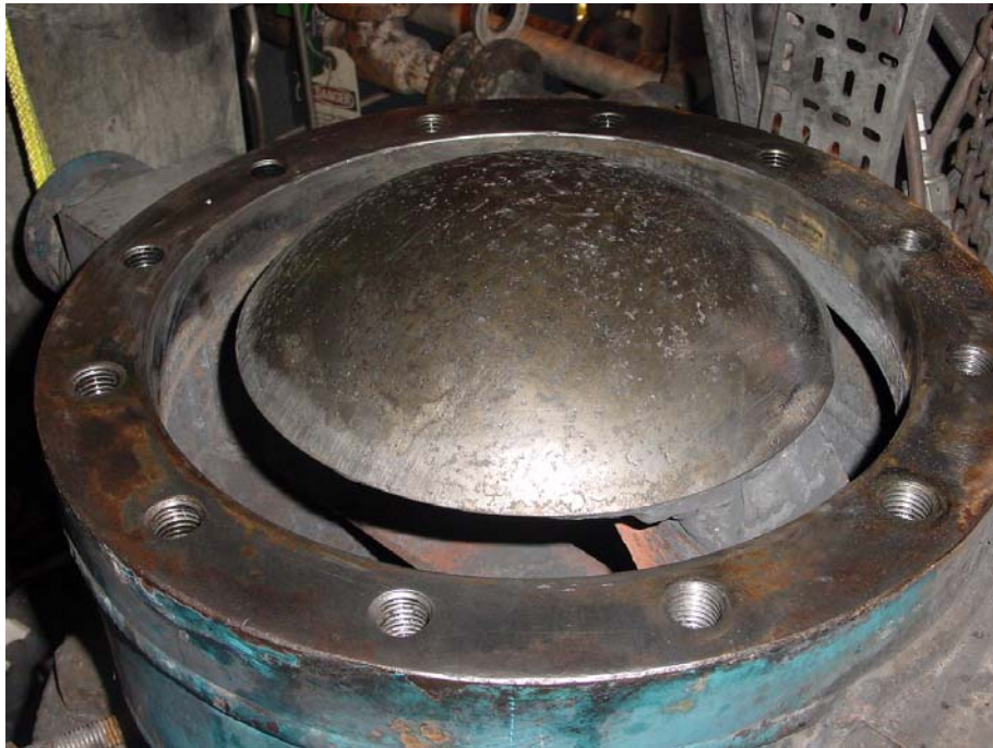
Figure 3.3-33 Upper Spheri Valve After Cleaning
