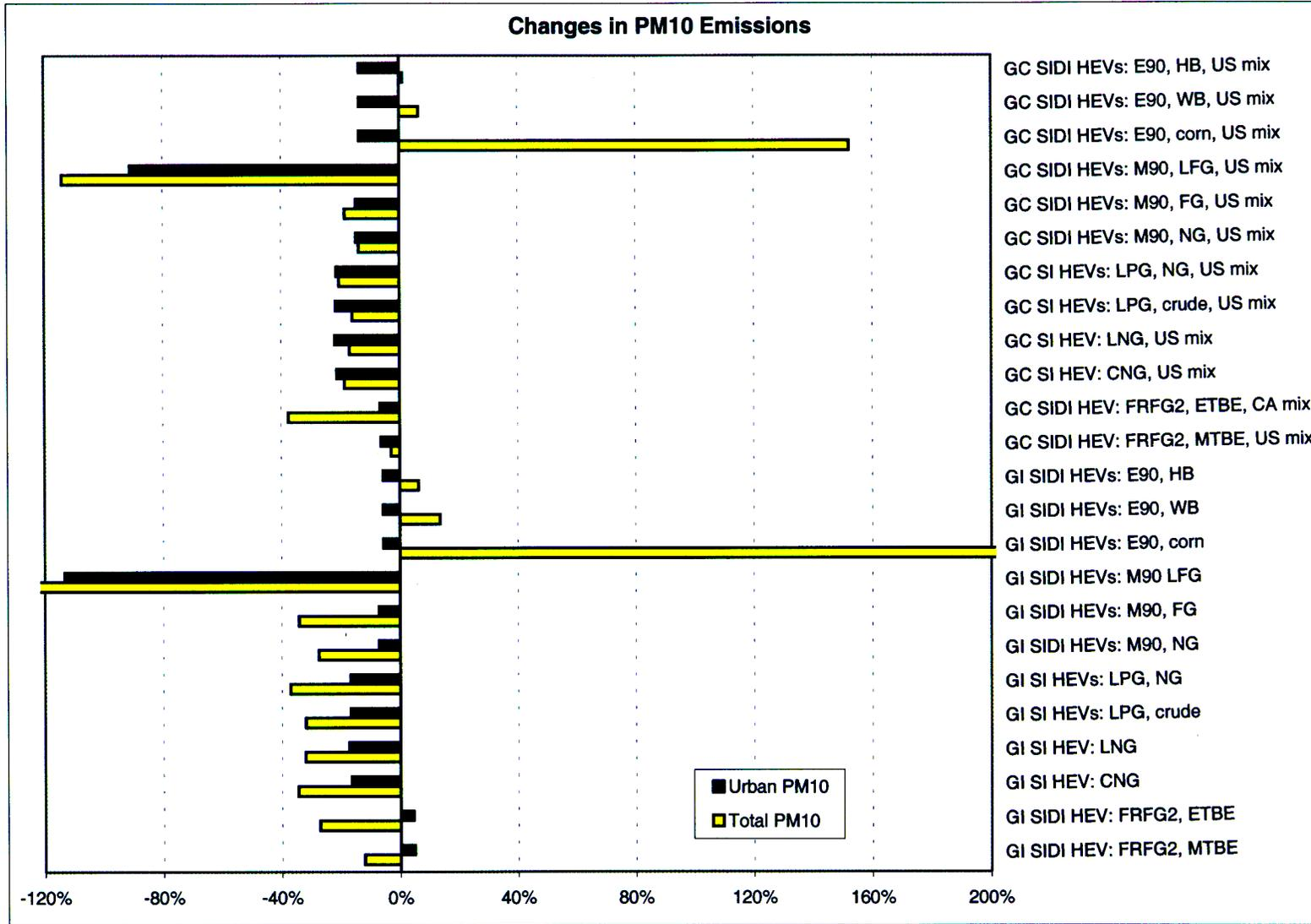
Figure 6.60 Changes in Fuel-Cycle Total and Urban PM<sub>10</sub> Emissions Relative to GVs Fueled with RFG: Long-Term SI and SIDI HEVs
