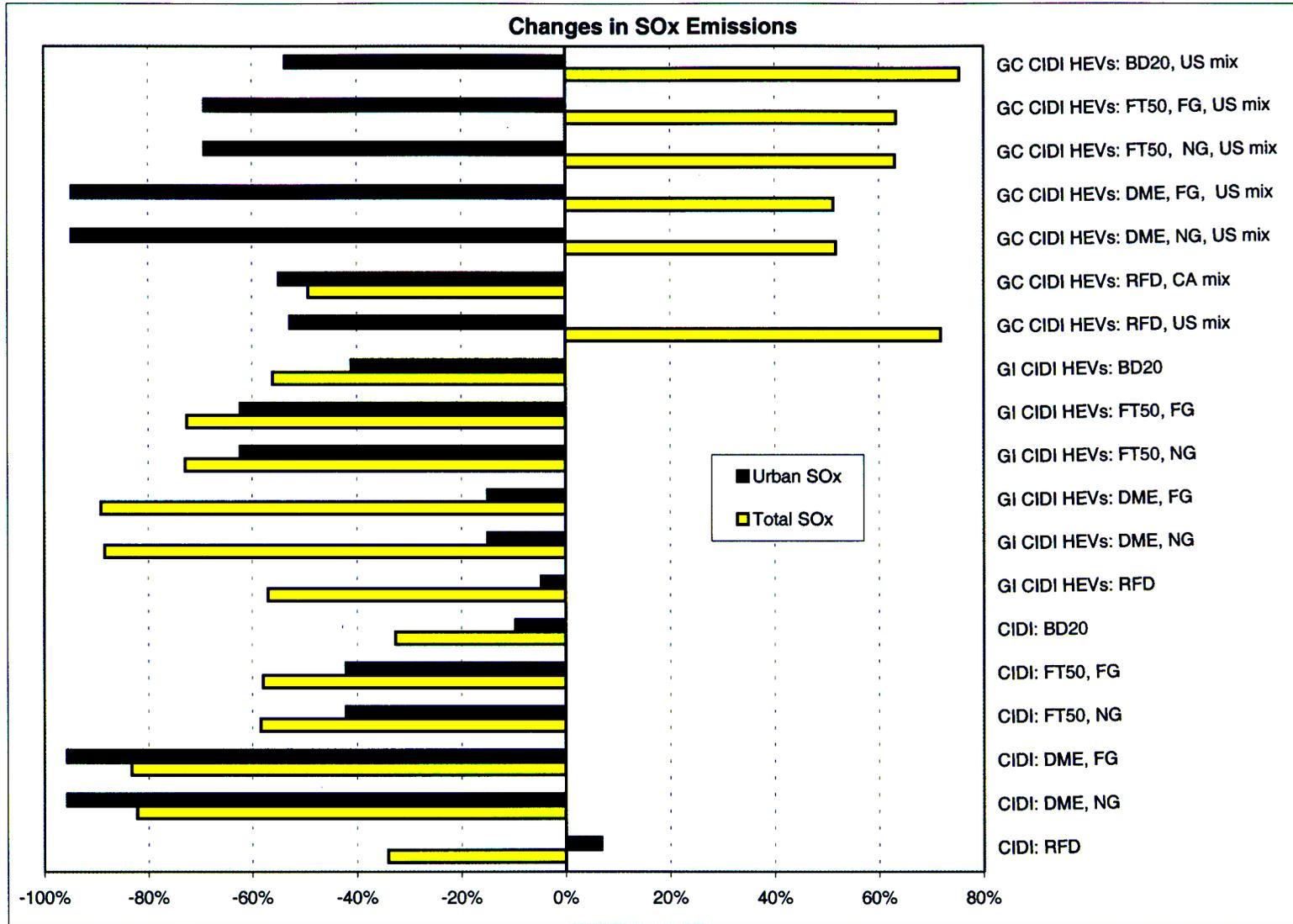
**Figure 6.65 Changes in Fuel-Cycle Total and Urban SO<sub>x</sub> Emissions Relative to GVs Fueled with RFG: Long-Term CIDI Vehicles and CIDI HEVs**
