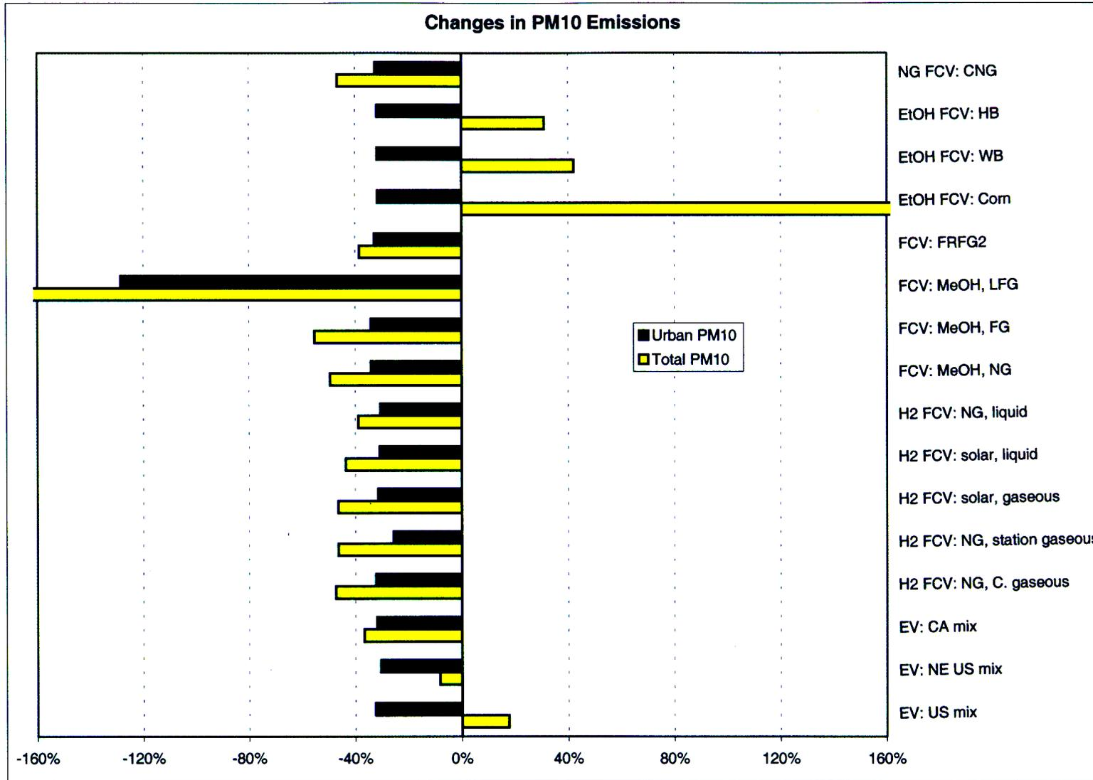
**Figure 6.62 Changes in Fuel-Cycle Total and Urban PM<sub>10</sub> Emissions Relative to GV's Fueled with RFG: Long-Term EVs and FCVs**
