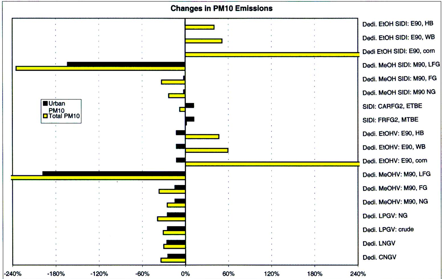
**Figure 6.59 Changes in Fuel-Cycle Total and Urban PM<sub>10</sub> Emissions Relative to GVs Fueled with RFG: Long-Term SI and SIDI Vehicles**
