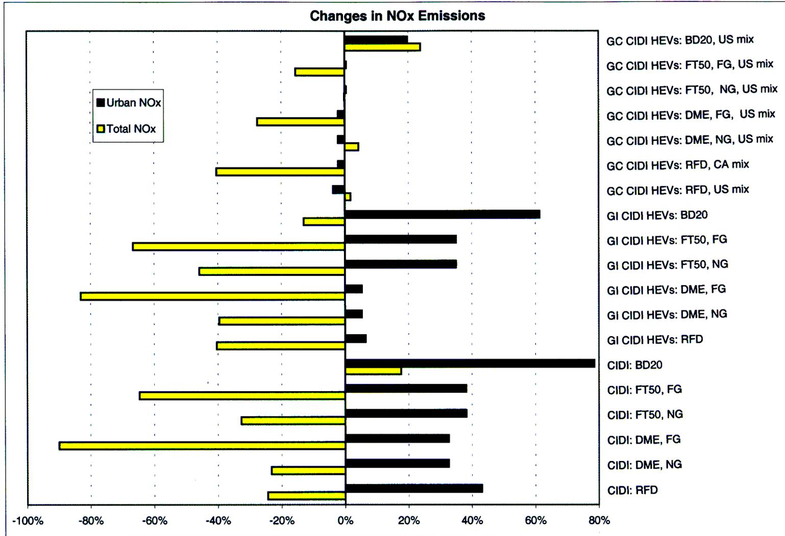
**Figure 6.57 Changes in Fuel-Cycle Total and Urban NO<sub>x</sub> Emissions Relative to GVs Fueled with RFG: Long-Term CIDI Vehicles and CIDI HEVs**
