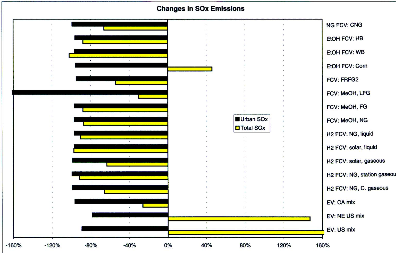
**Figure 6.66 Changes in Fuel-Cycle Total and Urban SO<sub>x</sub> Emissions Relative to GV<sub>s</sub> Fueled with RFG: Long-Term EV<sub>s</sub> and FCV<sub>s</sub>**
