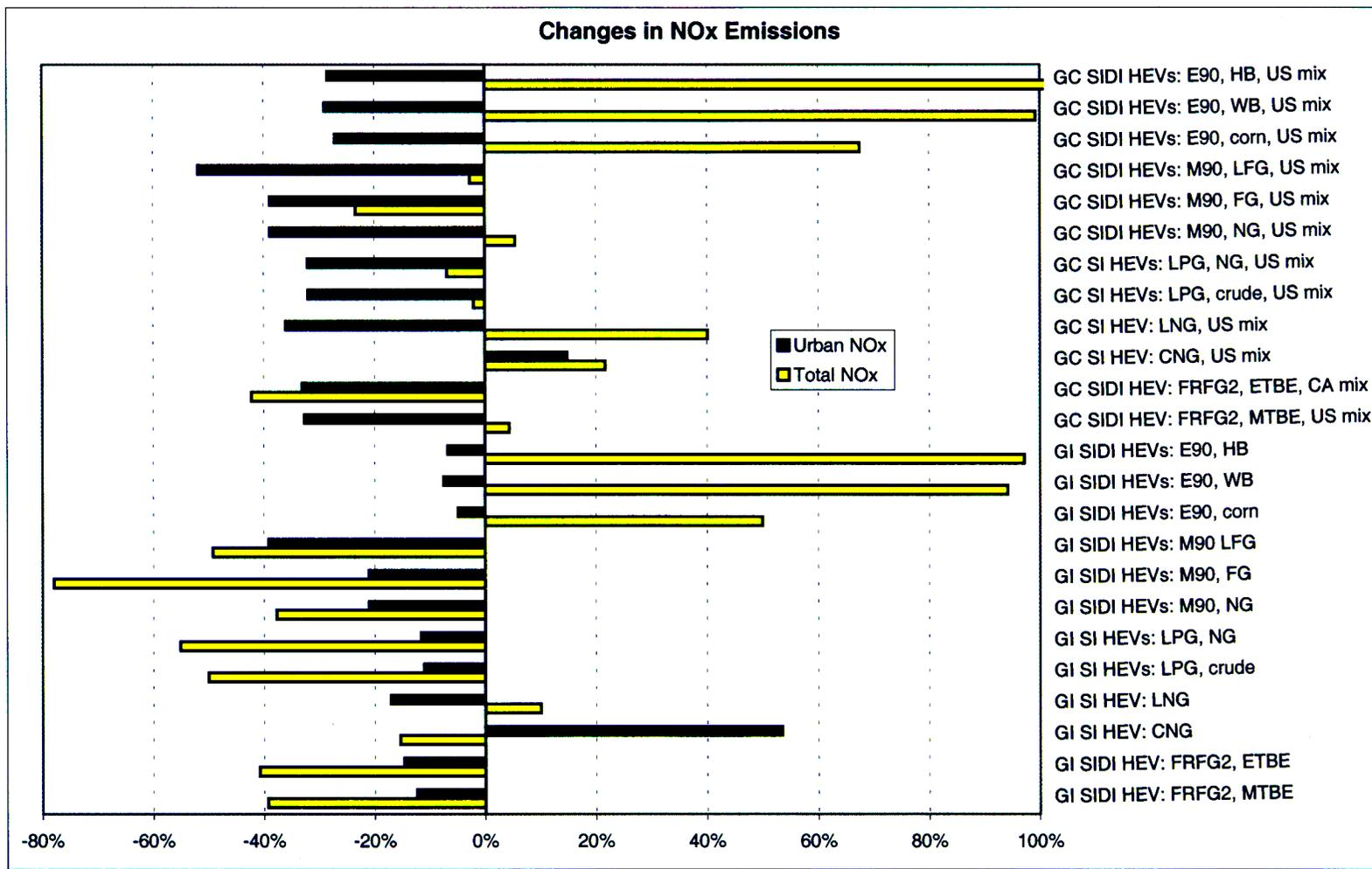
**Figure 6.56 Changes in Fuel-Cycle Total and Urban NO<sub>x</sub> Emissions Relative to GVs Fueled with RFG: Long-Term SI and SIDI HEVs**
