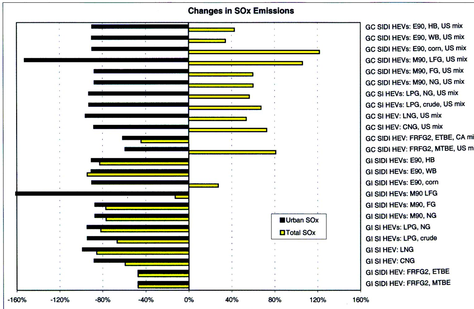
**Figure 6.64 Changes in Fuel-Cycle Total and Urban SO<sub>x</sub> Emissions Relative to GVs Fueled with RFG: Long-Term SI and SIDI HEVs**
