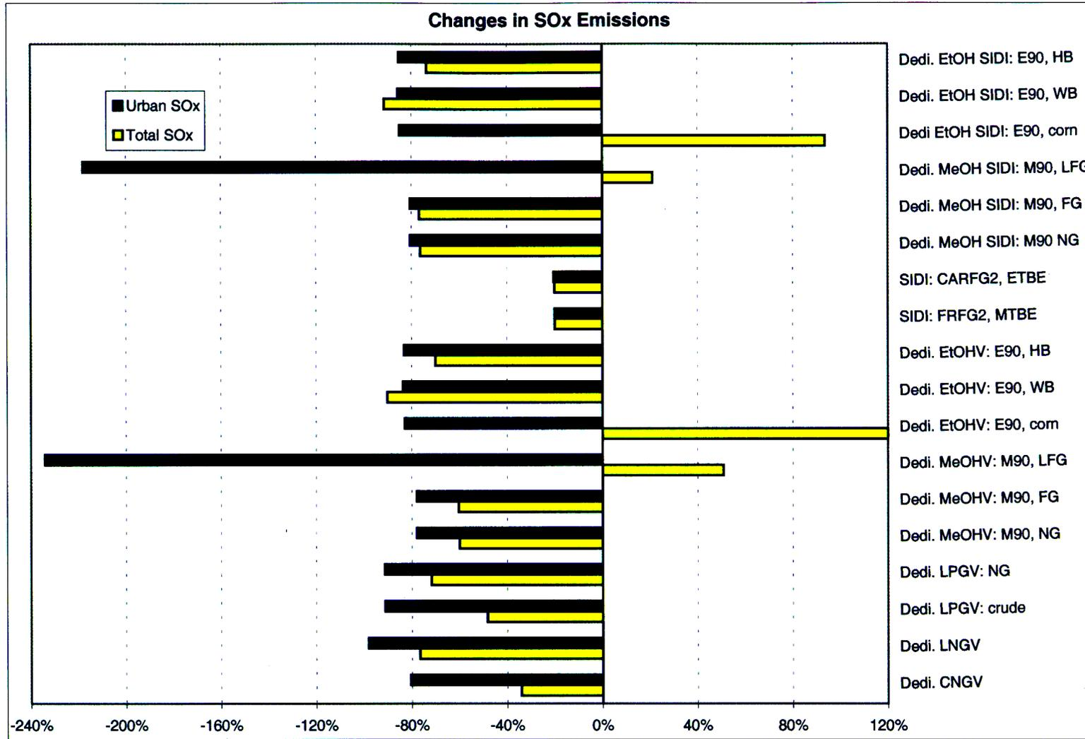
**Figure 6.63 Changes in Fuel-Cycle Total and Urban SO<sub>x</sub> Emissions Relative to GVs Fueled with RFG: Long-Term SI and SIDI Vehicles**
