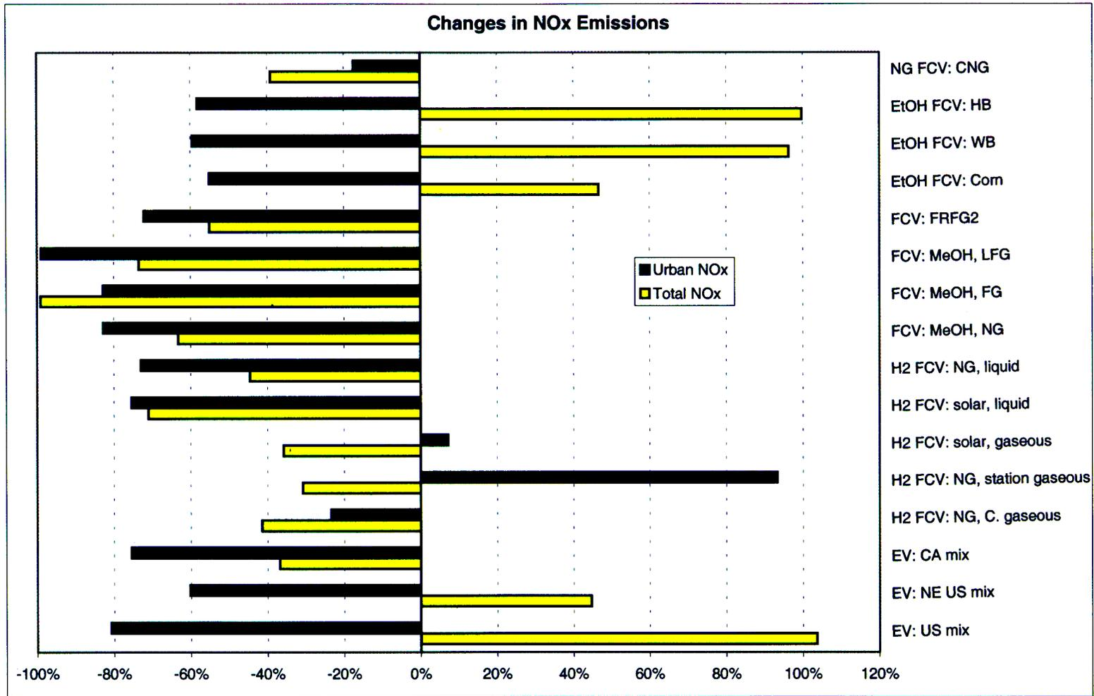
**Figure 6.58 Changes in Fuel-Cycle Total and Urban NO<sub>x</sub> Emissions Relative to GVs Fueled with RFG: Long-Term EVs and FCVs**
