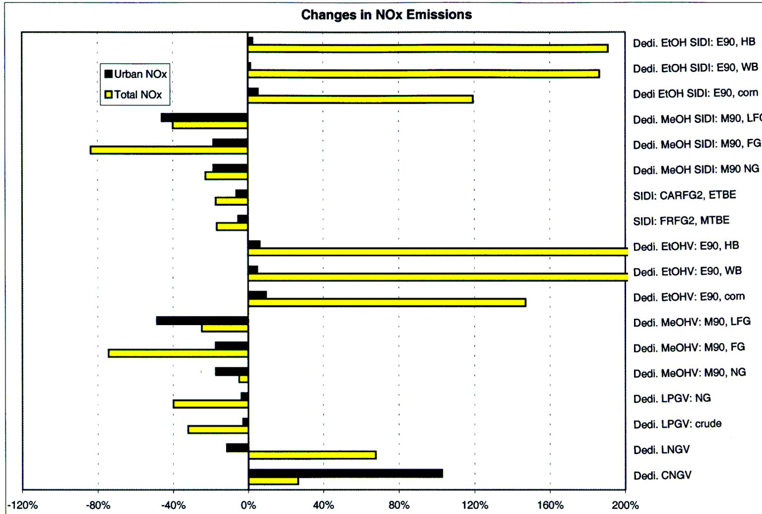
**Figure 6.55 Changes in Fuel-Cycle Total and Urban NO<sub>x</sub> Emissions Relative to GVs Fueled with RFG: Long-Term SI and SIDI Vehicles**
