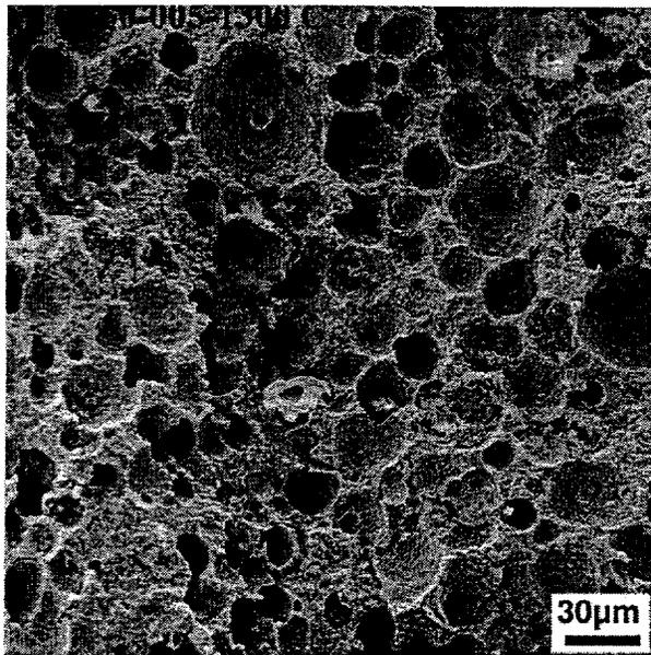
Figure 5: CS-50, + 50 vol% starch, sintered at 1300°C.
