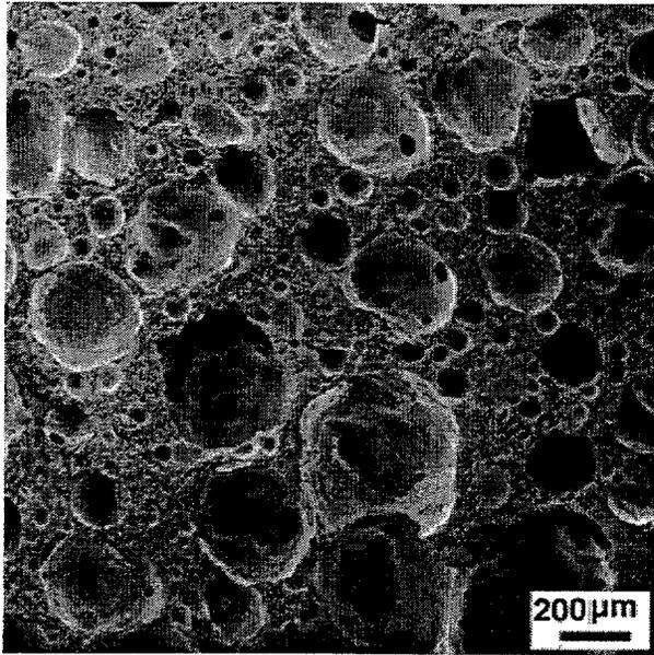
Figure 4: SEM picture of CS-50 gelcast foam
