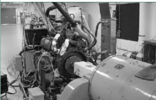
The Navistar T444E engine was installed on a GE-2000 DC dynamometer at WVU's test facility.
