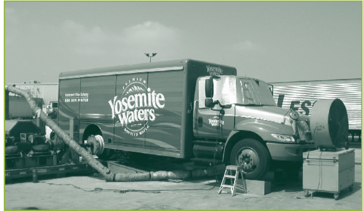
Figure 11. Yosemite Waters vehicle on WVU chassis dynamometer
