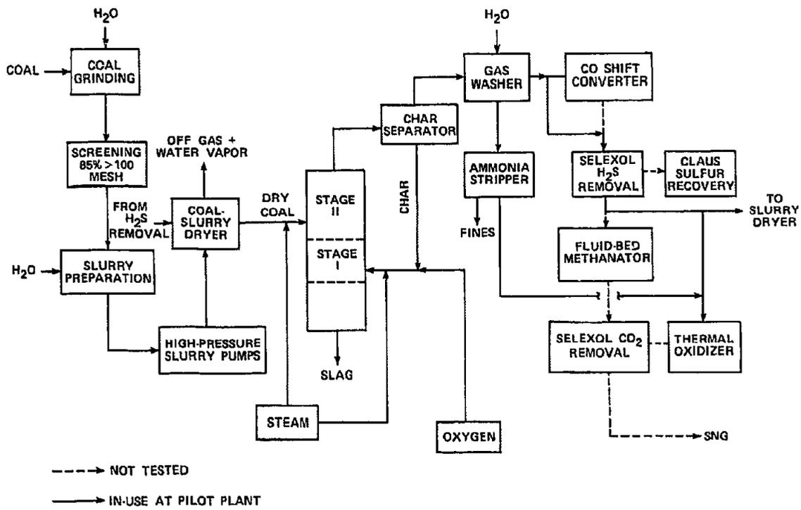
Figure 3-1. Bi-Gas Block Flow Diagram
