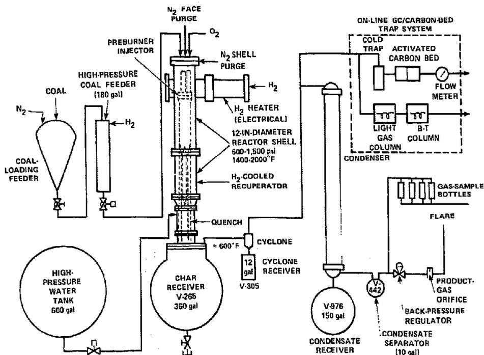
**Figure 5-2. Simplified Flow Diagram of CS/RI 3/4-tph Reactor System**
