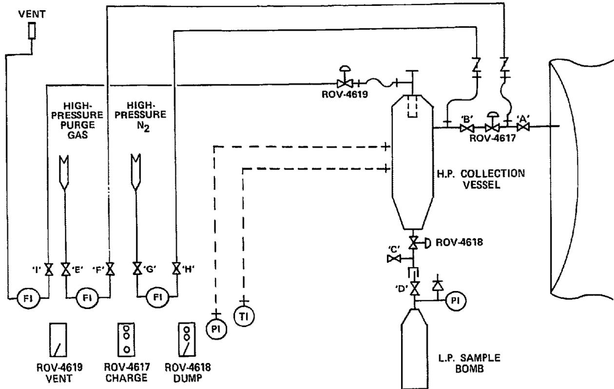
Figure 6-4. Char-Feed Vessel-Sample System
