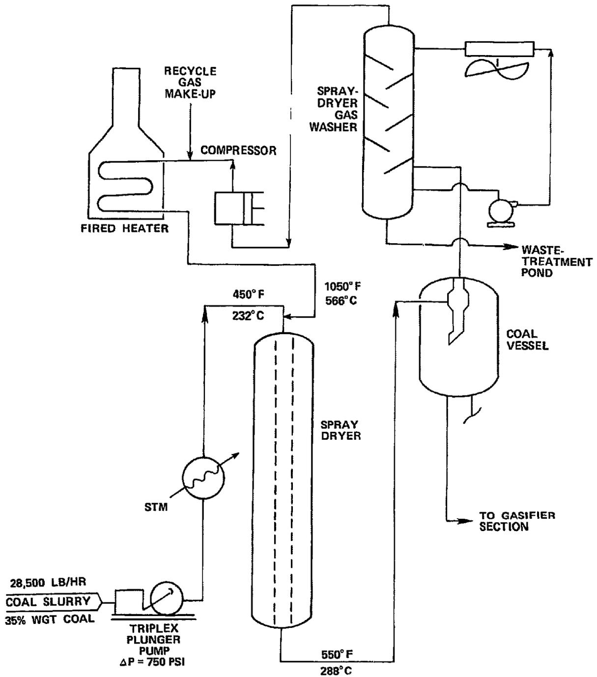
Figure 6-1. Bi-Gas Coal-Slurry Spray-Drying Section
