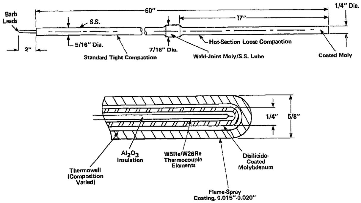
Figure 6-3. Bi-Gas Stage I Thermocouple and Thermowell
