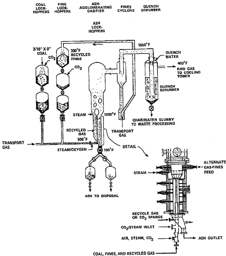
Figure 4-2. Westinghouse PDU Process Schematic
