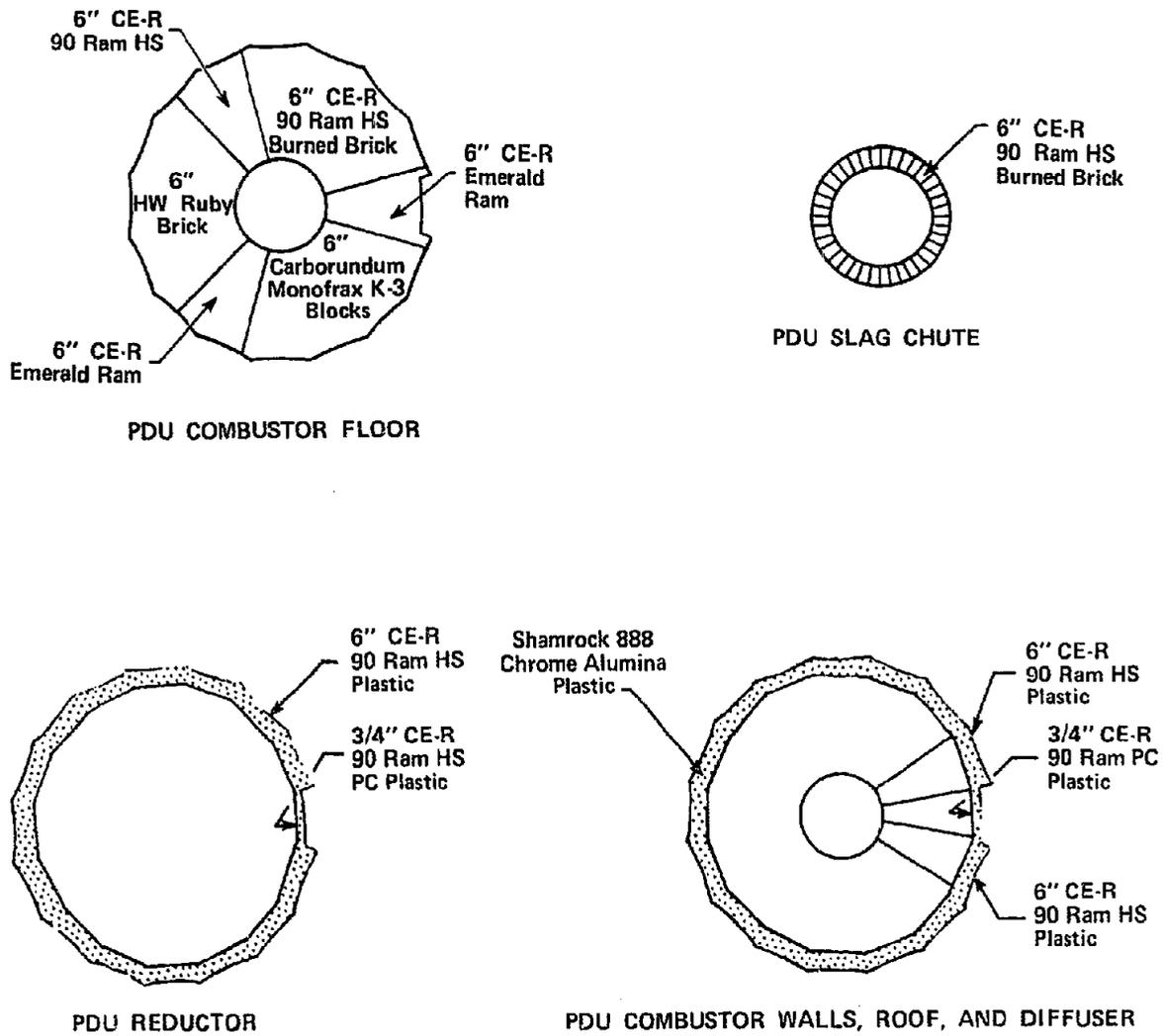
Figure 6-5. C-E PDU Gasifier Refractory-Lining Materials
