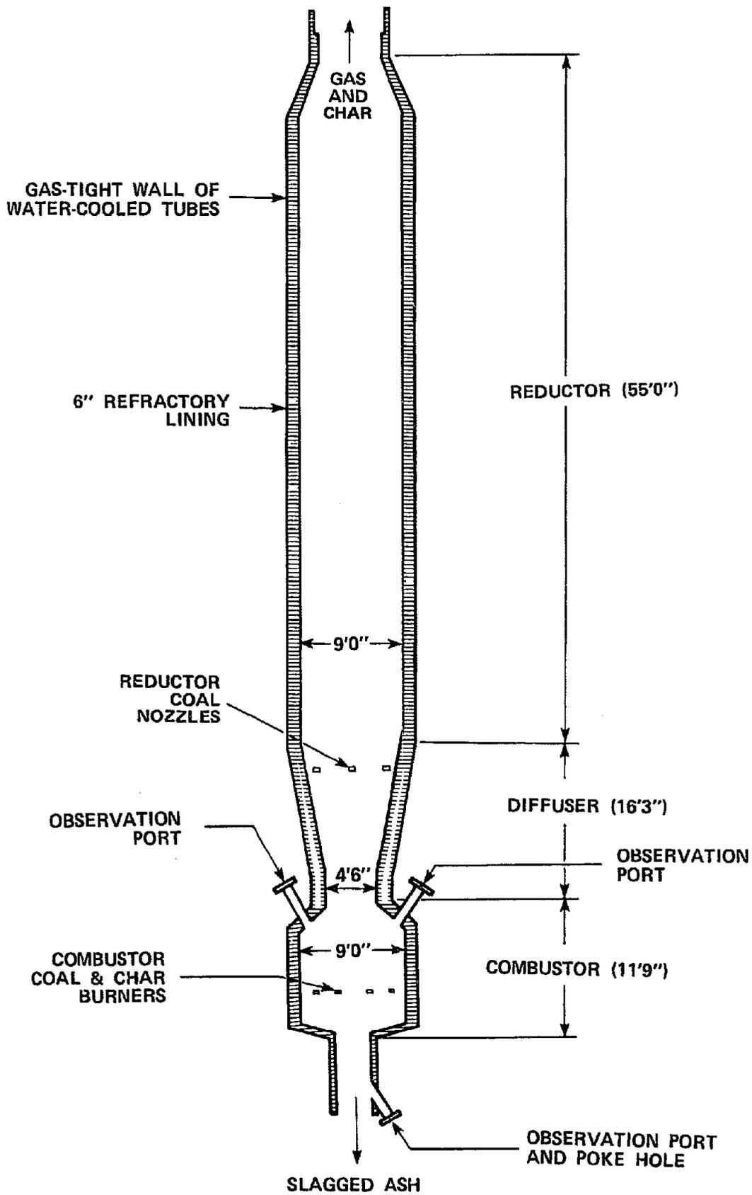
Figure 2-1. Combustion Engineering PDU Gasifier Schematic
