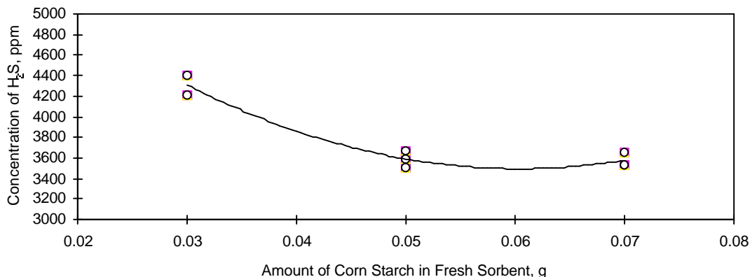
Figure 5. Effects of corn starch amount on reactivity of sorbents with initial 7400 ppm dry H 2 S for 120 seconds at 550°C.
