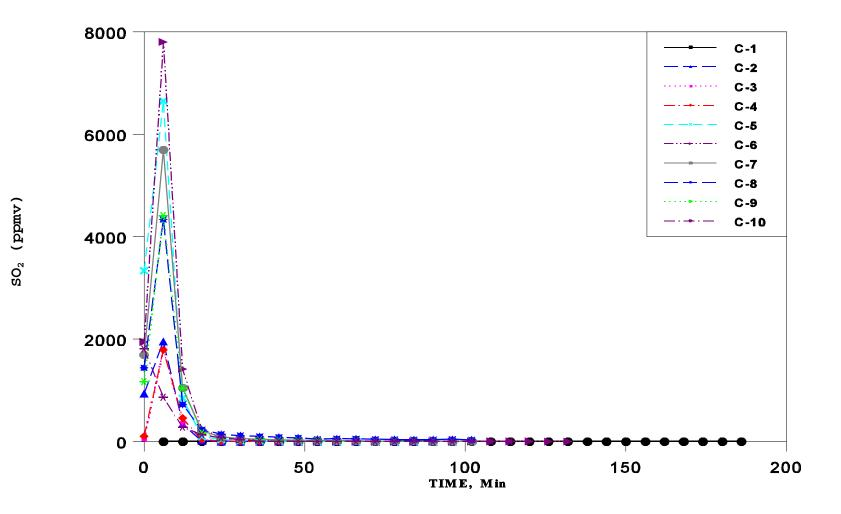
Figure 2.  $SO_2$  Evolution During Sulfidation Due to sulfation
