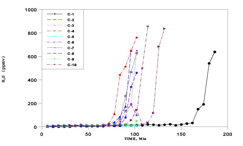
Figure 1. Breakthrough Behavior of MCRH-61
