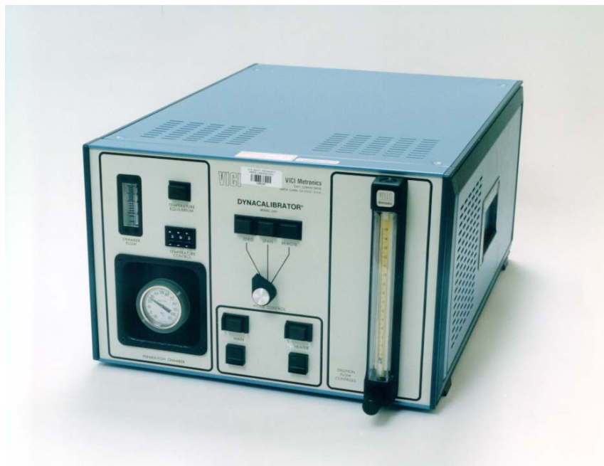
Figure 36. VICI Metronics Model 340 Dynacalibrator.
