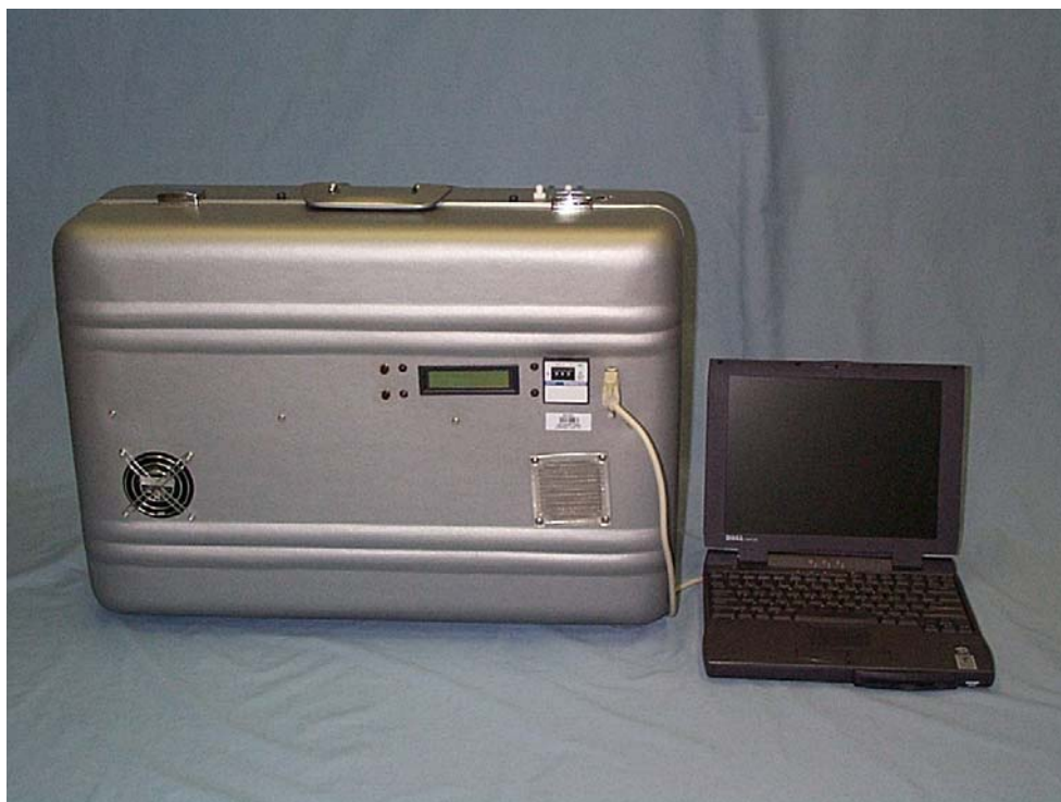
Figure 18. Mercury Analyzer Employing a D 2 Background Correction System.
