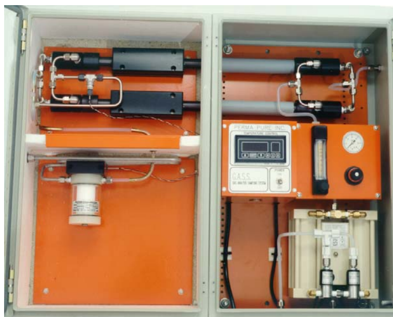
Figure 3. Gas Drying System from Perma Pure.
