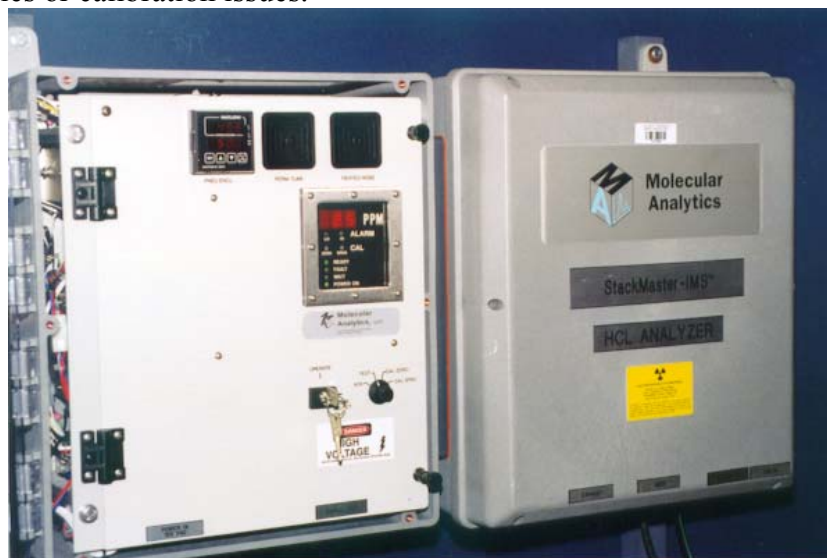
Figure 32. Ion Mobility Spectrometer for Monitoring HCl.
