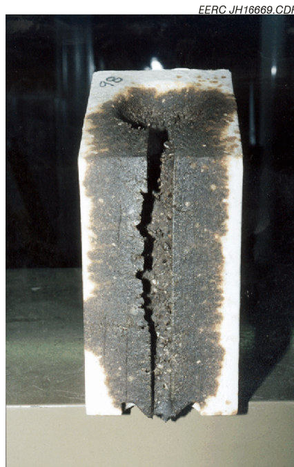
Figure 3-63. Photograph of uncoated Plicast 98 material that was pre-fired and tested at 2732°F (1500°C) for 54 hours using Illinois No. 6 slag.
