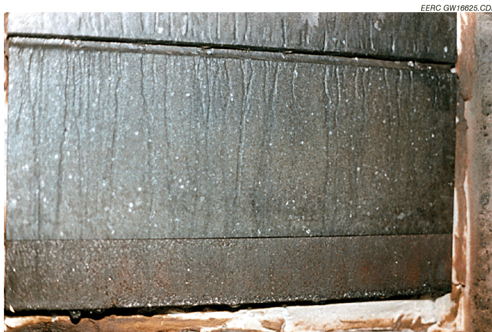
Figure 3-43. Photograph of the RAH lower support brick, small lower tile, and the lower edge of the large lower tile following the February test.
