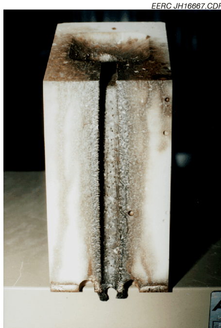
Figure 3-61. Photograph of the Monofrax after 100 hours of slag feed at 2732°F (1500°C) using Illinois No.6 slag.
