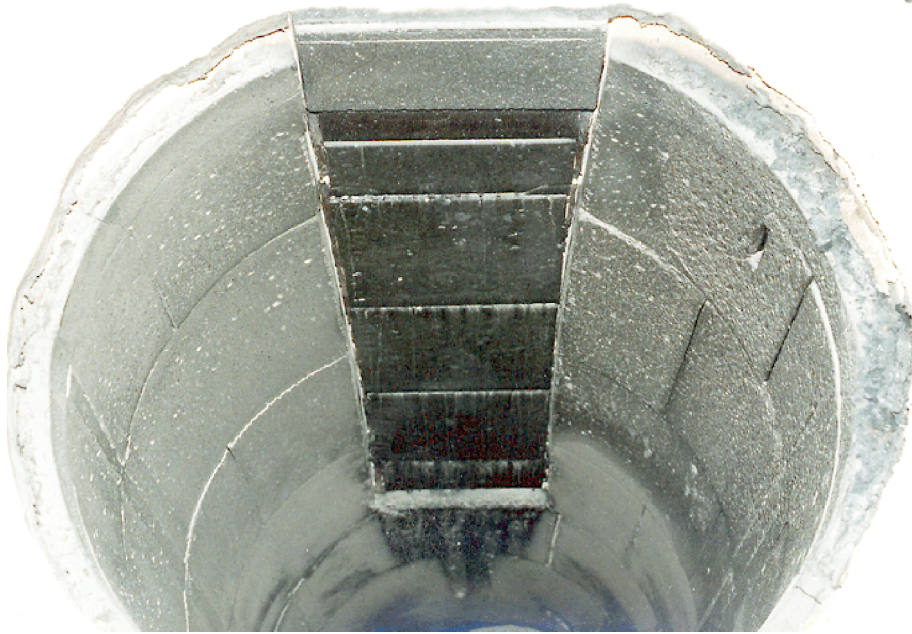
Figure 3-40. Photograph of the RAH panel inside of the slagging furnace following the April test.
