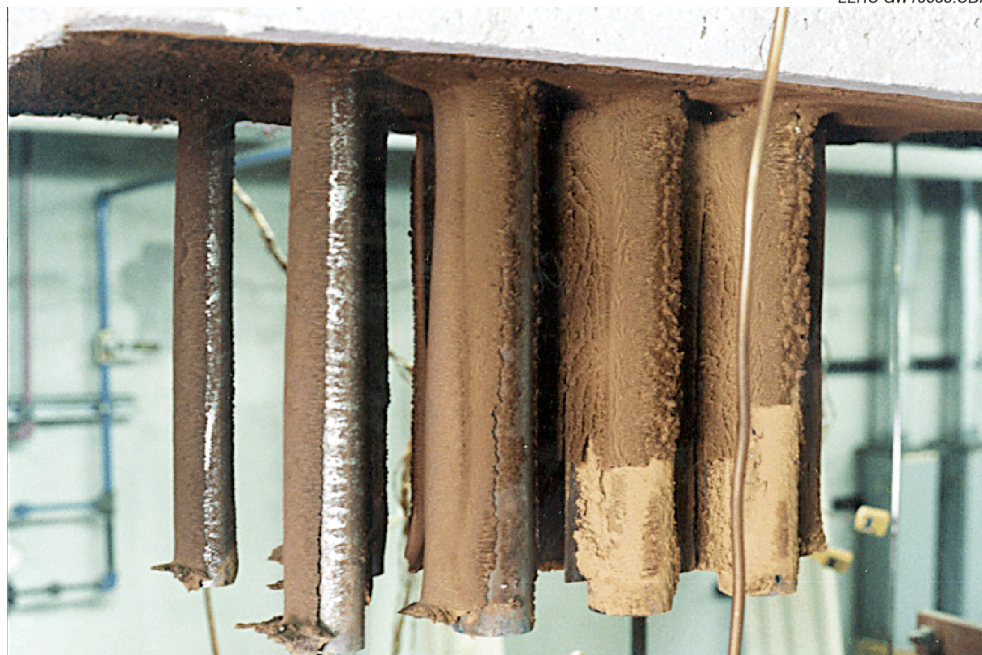
Figure 3-27. Photograph of ash deposits on the CAH tubes following the January test firing Illinois No. 6 bituminous coal.
