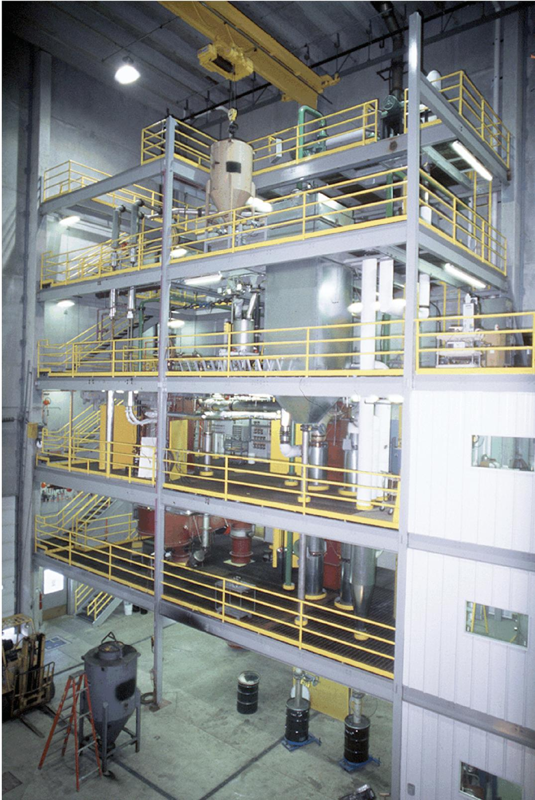
Figure 2-1. Photograph of the pilot-scale slagging furnace system.
