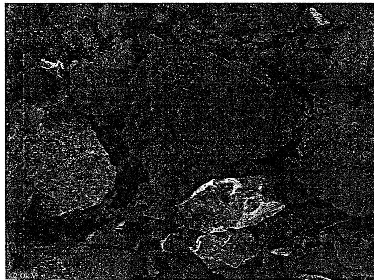
Figures 7.11 & 7.12 SEM micrographs of gasified char samples (reactor-aged) of the L.NK-coal mixture
