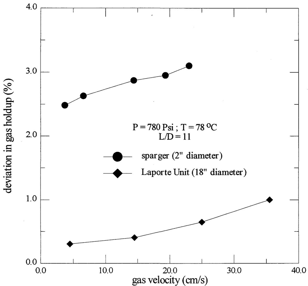
Figure 2. Comparison of deviation in gas holdup between two-inch column and LaPorte Unit.
