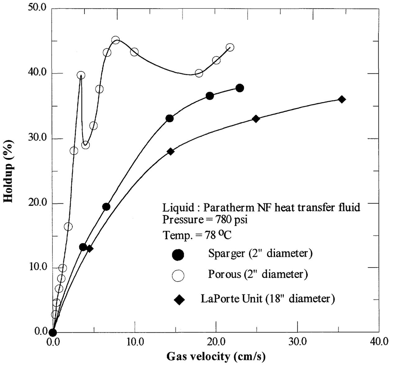
Figure 1. Comparison of gas holdup between two-inch column and LaPorte unit
