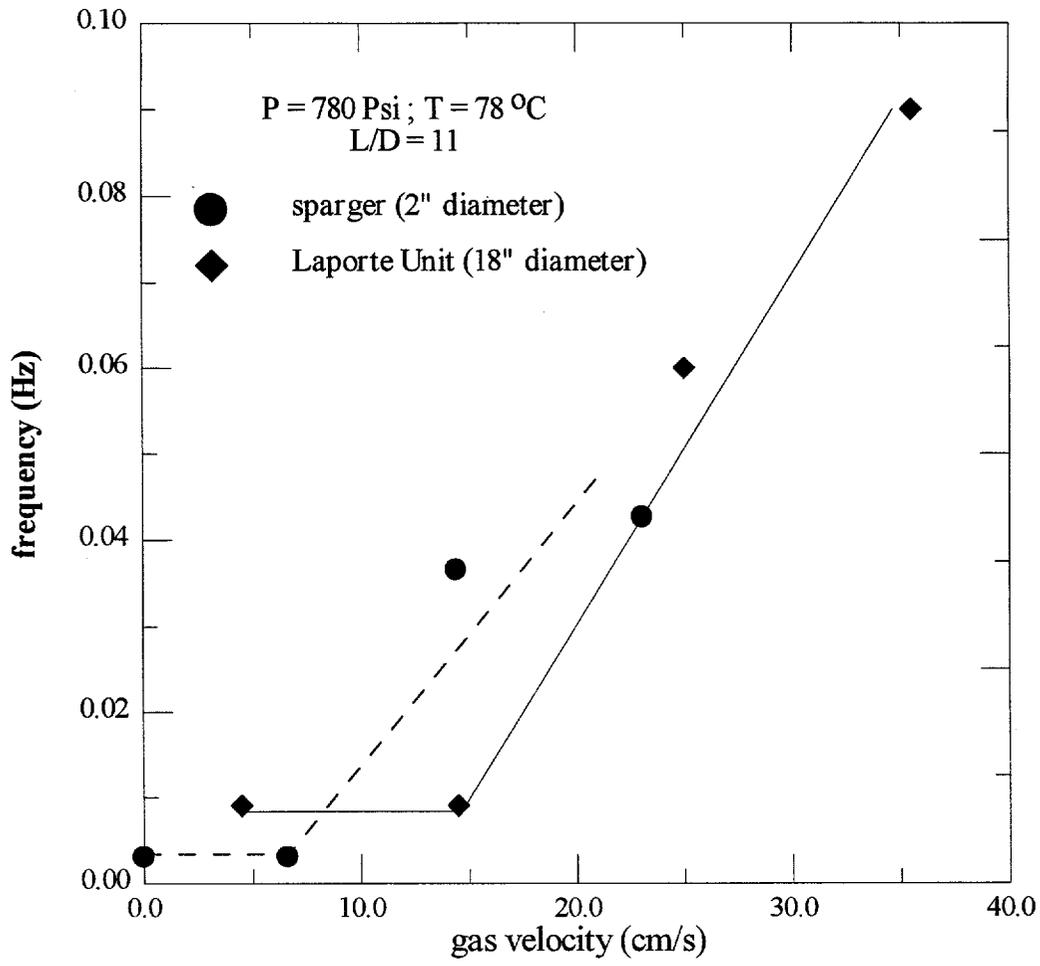
Figure 3. Power spectrum analysis of differential pressure fluctuation for two-inch column and LaPorte unit
