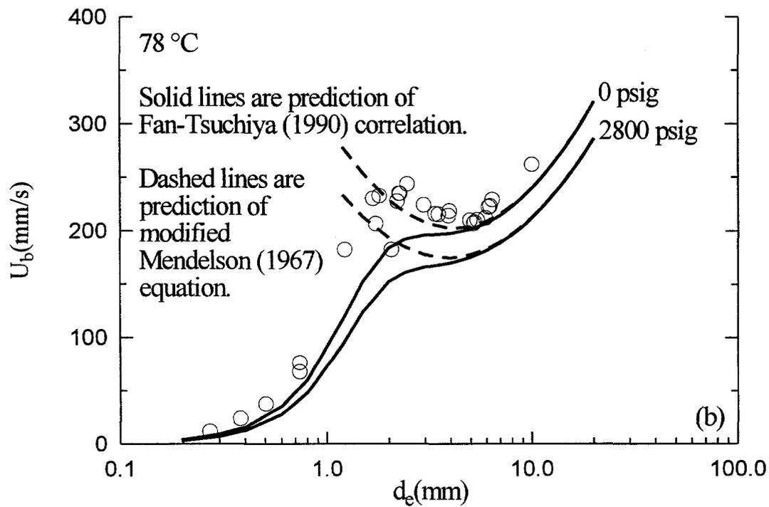
Figure 4. Effect of pressure on terminal rise velocity of single bubbles in Parather NF heat transfer fluid and its prediction at (a)  $27\text{ }^\circ\text{C}$  and (b)  $78\text{ }^\circ\text{C}$ .
