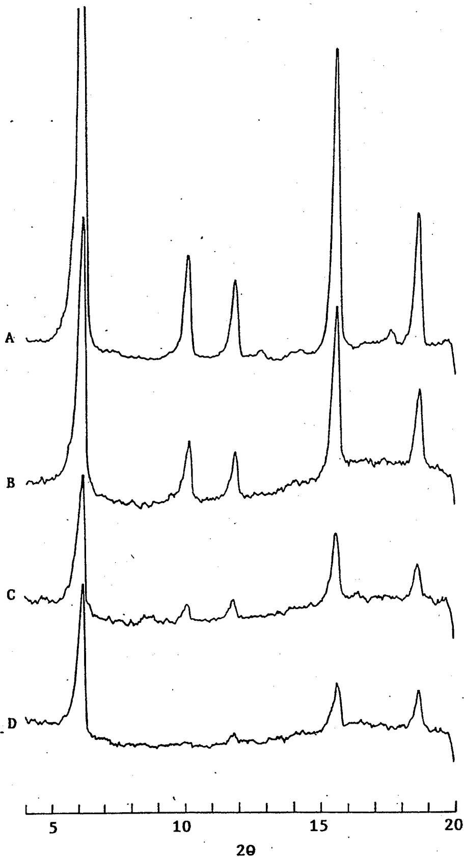
Figure 11. XRD spectra of \gamma -zeolite and supported samples reduced at 700^{\circ}\text{C} : A, \gamma -zeolite; B, 5 wt% Ni/Y; C, 5-5 Ni-Ce/Y; D, 5-10 Ni-Ce/Y.
