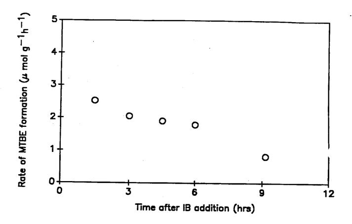
Figure 2.6 Rate of MTBE formation over Li6/Pd/S1 + ZSM-5 (physical mixture) using a syngas + isobutylene feed.
