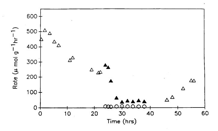
Figure 2.5 Rate of methanol and MTBE formation over Li1/Pd/S1 + ZSM-5. Open and closed triangles represent methanol rates in the absence and presence of isobutylene, respectively. Open circles represent rate of MTBE formation x 10.
