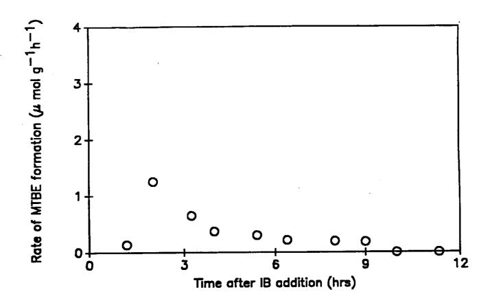
Figure 2.7 Rate of MTBE formation over Li6/Pd/S1 + LZ210-12 (physical mixture) using a syngas + isobutylene feed.
