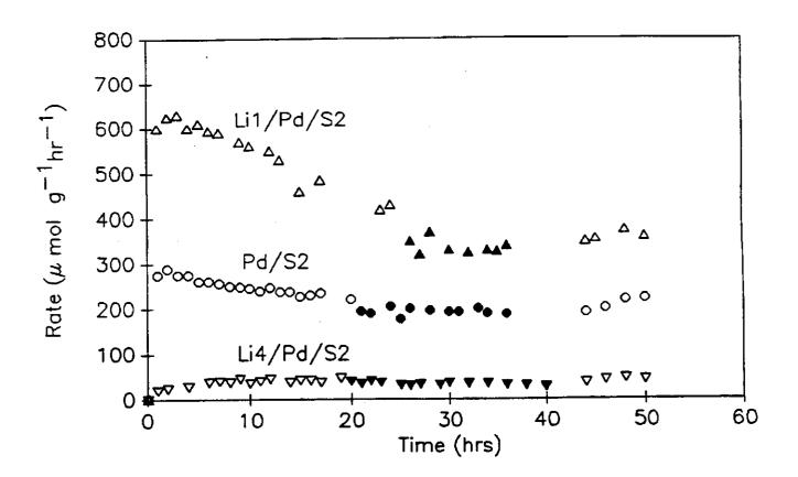
Figure 2.2 Rate of methanol formation over Pd and Li-Pd catalysts.
