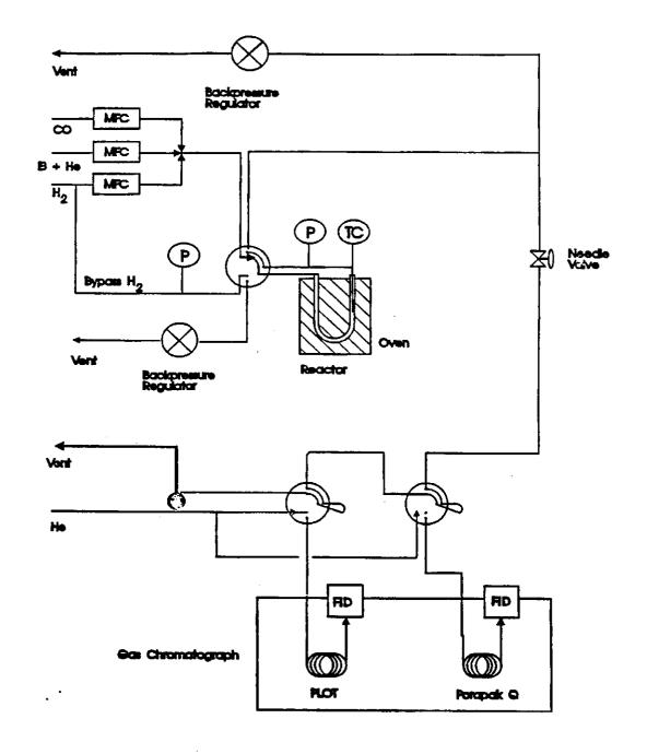
Figure 2.1 Schematic of reaction system used in syngas studies
