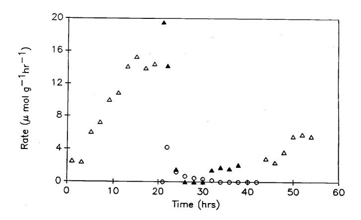
Figure 2.3 Rate of methanol and MTBE formation over Li4/Pd/S2 + ZSM-5. Open and closed triangles represent methanol rates in the absence and presence of isobutylene, respectively. Open circles represent rate of MTBE formation.
