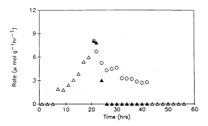
Figure 2.4 Rate of methanol and MTBE formation over Li4/Pd/S2 + LZ210-12. Open and closed triangles represent methanol rates in the absence and presence of isobutylene, respectively. Open circles represent rate of MTBE formation.
