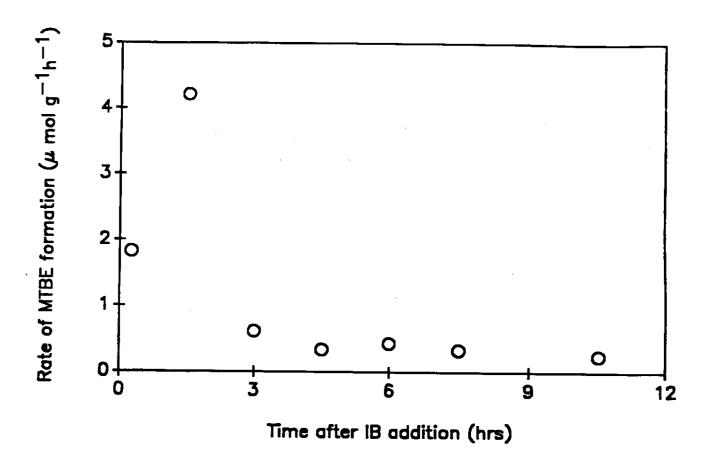
Figure 2.8 Rate of MTBE formation over Li6/Pd/S1 + ZSM-5 (dual bed) using a syngas + isobutylene feed.
