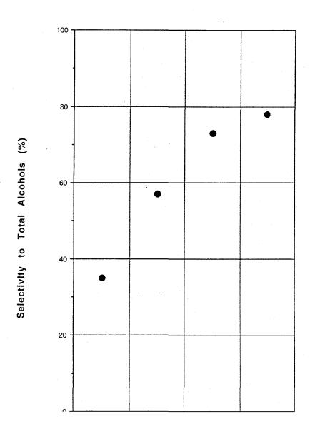
Figure 5. Rate to total alcohols vs. K loading for 6 wt% Pd on ZnCr spinel with excess Zn. Tested in a copper-lined tube at  $440^{\circ}$ C, 1500 psi with GHSV 12000 and  $H_2/CO = 1$
