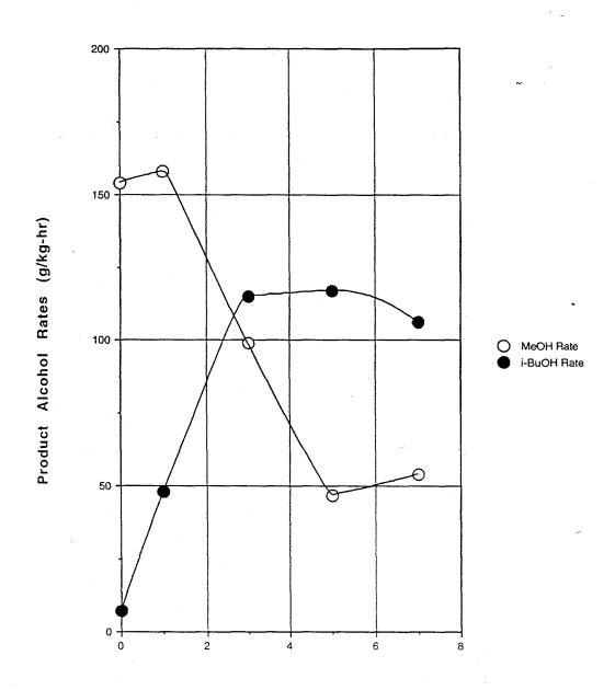
Figure 4. Selectivity to total alcohols vs. K loading for 6 wt% Pd on ZnCr spinel with excess Zn. Tested in a copper-lined tube at  $440^{\circ}$ C, 1500 psi with GHSV 12000 and  $H_2/CO = 1$
