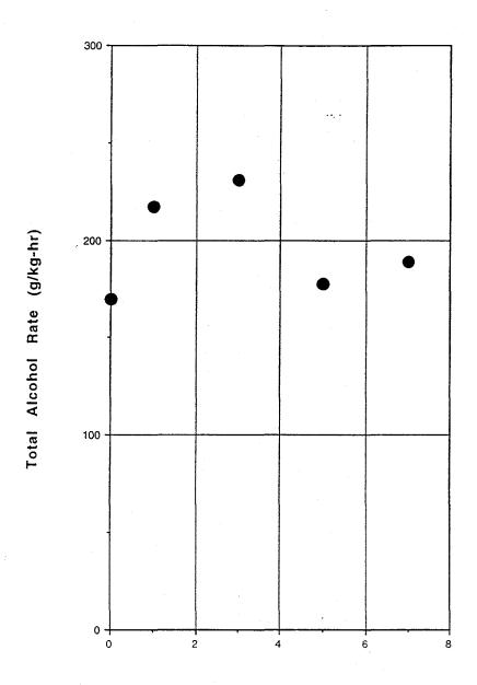
Figure 3. Rates to methanol and isobutanol vs. K loading on ZnCr spinel with excess Zn. Tested in a copper-lined tube at  $440^{\circ}$ C, 1500 psi with GHSV 12000 and  $H_2/CO = 1$
