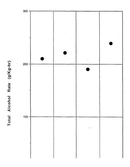
Figure 4. Selectivity to total alcohols vs. K loading for 6 wt% Pd on ZnCr spinel with excess Zn. Tested in a copper-lined tube at  $440^{\circ}$ C, 1500 psi with GHSV 12000 and  $H_2/CO = 1$
