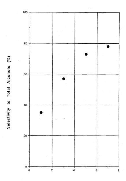
Figure 5. Rate to total alcohols vs. K loading for 6 wt% Pd on ZnCr spinel with excess Zn. Tested in a copper-lined tube at  $440^{\circ}$ C, 1500 psi with GHSV 12000 and H<sub>2</sub>/CO = 1
