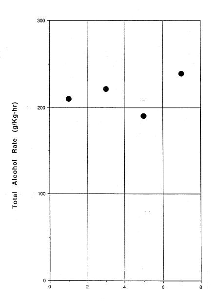
Figure 6. Rates to methanol and isobutanol vs. K loading for 6 wt% Pd on ZnCr spinel with excess Zn. Tested in a copper-lined tube at  $440^{\circ}$ C, 1500 psi with GHSV 12000 and  $H_2/CO = 1$
