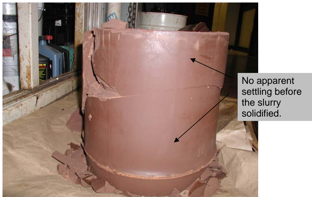
Figure 12. Photograph of "frozen" catalyst/wax slurry after 26 days of circulation.
