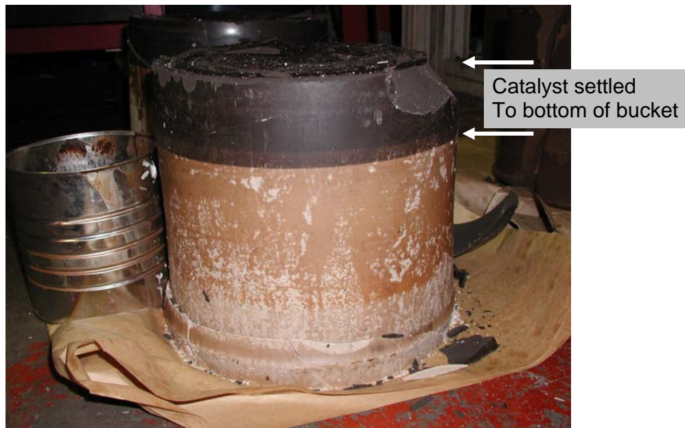
Figure 11. Photograph of "frozen" catalyst/wax mixture after 12 days of circulation.
