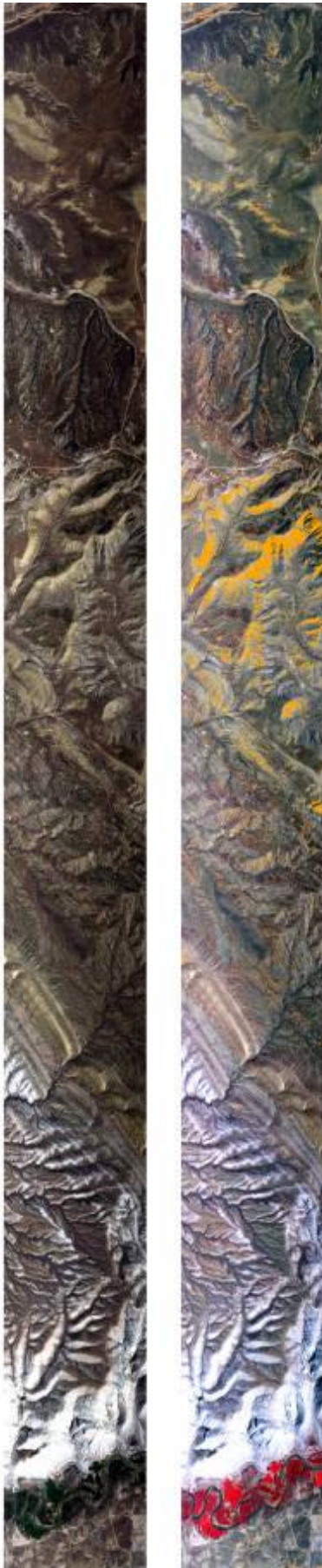
Figure 9 Flight line 3 hyperspectral image analyzed using ENVI to produce a “true color” image shown on the left. The area includes the Rangely Oil Field shown in the photo previous figure. On the right there is a composite image of a map of what appears to be a mixture of Montmorillonite and Kaolinite mineral soils overlaid on a color infrared RGB produced from the hyperspectral image. Wendy Cover using the commercial image analysis program ENVI did this analysis. Wendy is a first year PH. D. graduate student at UC Santa Cruz in our remote sensing program. The procedure she used is complex and is referred to in the literature as the ENVI “hourglass” in the literature. If anyone is interested in finding out more about the procedure contact Wendy Cover or Bill Pickles. In our previous experience, these maps are extremely accurate in arid regions, which this is. The Montmorillonite Kaolinite soil mixture is shown in orange. The red color at the bottom of the image is the lush vegetation along the White River banks. It is red because the underlying image is a pseudo “color infrared” made from the hyperspectral image using the bands 27, 16, and 7 as red, green, and blue respectively. The true color image on the left was similarly made using the bands 15, 9, and 2 as RGB.
