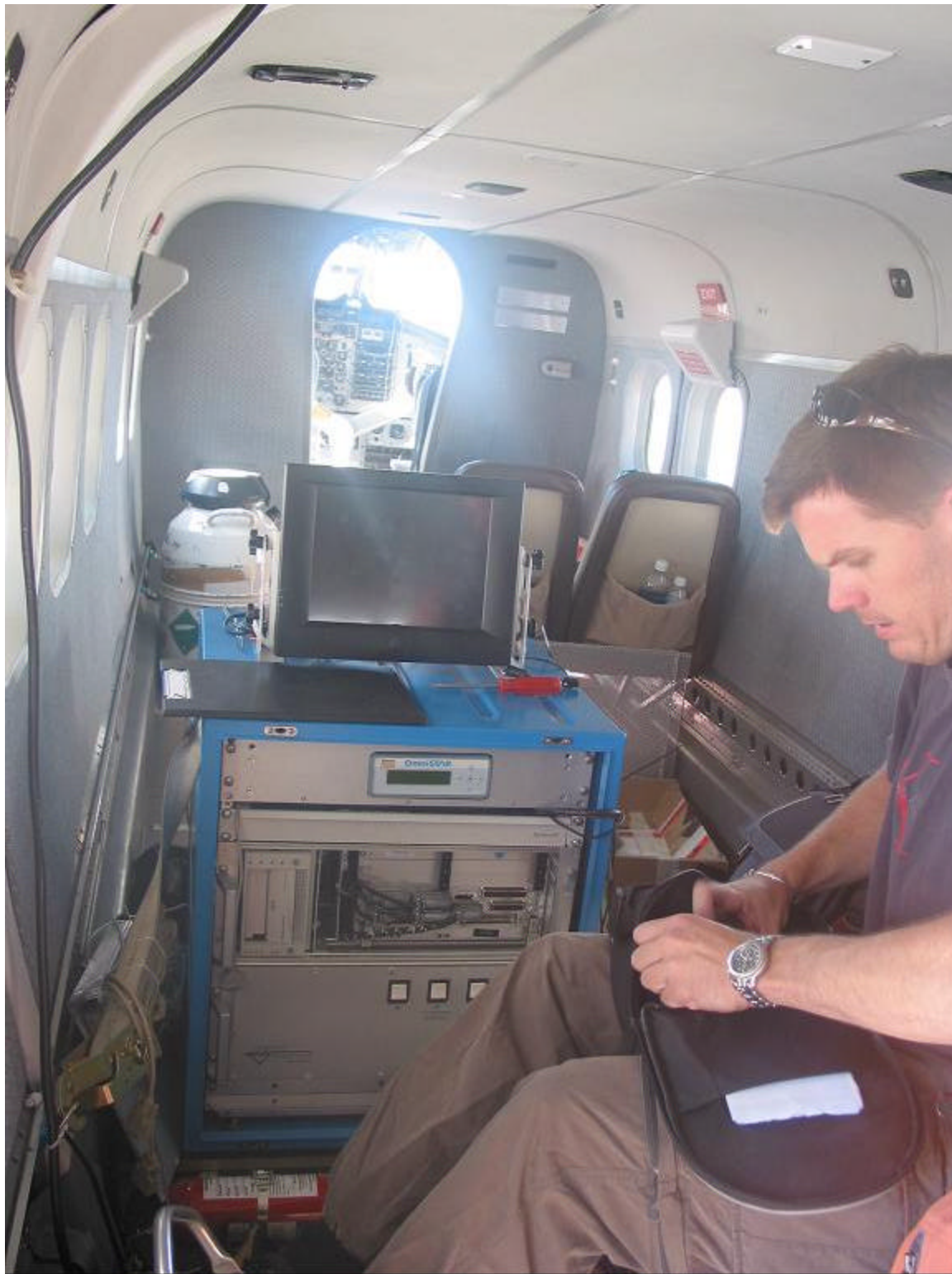
Figure 2 Ashley Hill is the acquisition contractor's sensor operator and flight commander. He is shown with the onboard computer system that controls the sensor systems and records the image, and the exact geolocation of each pixel in the image as it is acquired. The aircraft is the B300 Twin Otter.
