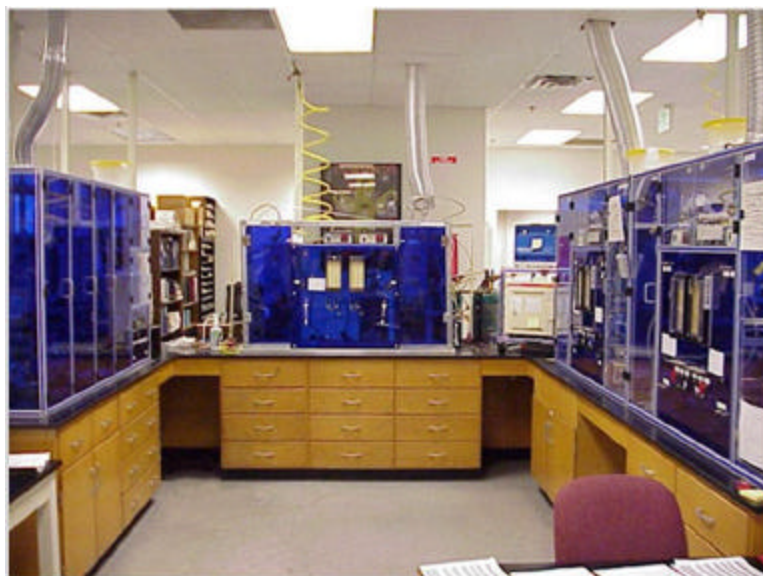
1.2.1.1.4.6 (3) Ambient pressure testing facility - Eltron Research Inc. Left: new reactors for testing membranes with water-gas shift catalyst. Right: reactors for screening membrane catalysts in steam and water-gas shift mixture. Center: reactors used for long-term tests.
