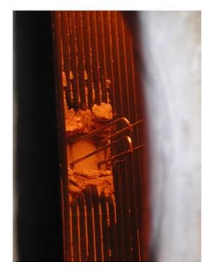
Figure 3. Air heater tube testing assembly installed in the upper
