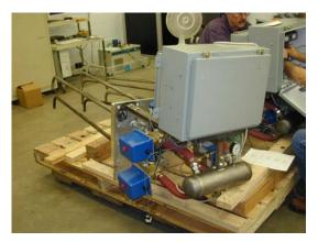
Figure 2. Furnace-side view of air heater tube testing assemblies
