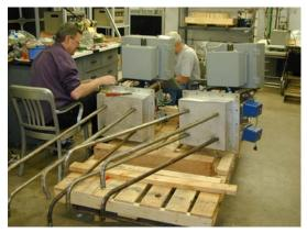
Figure 1. Air heater tube testing assemblies during final installation of instruments and controls
