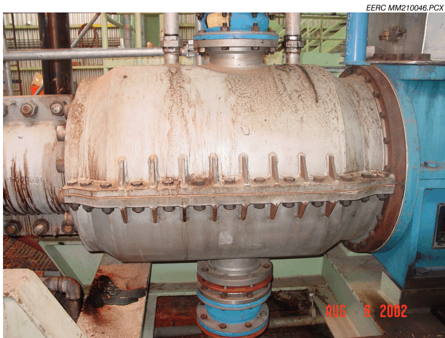
Figure 47. Throat section of plug-screw feeder.
