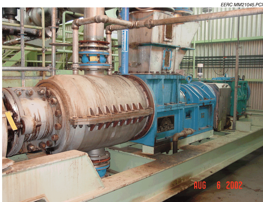
Figure 45. Plug-screw feeder system used in wood chip pulping process.
