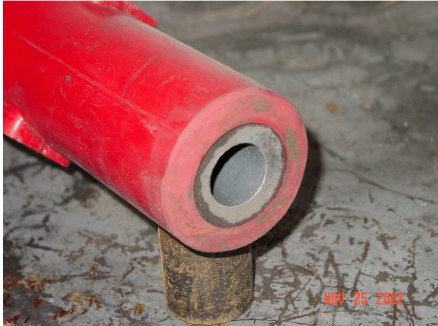
Figure 28. Plug inserted into tip of shotcrete nozzle.
