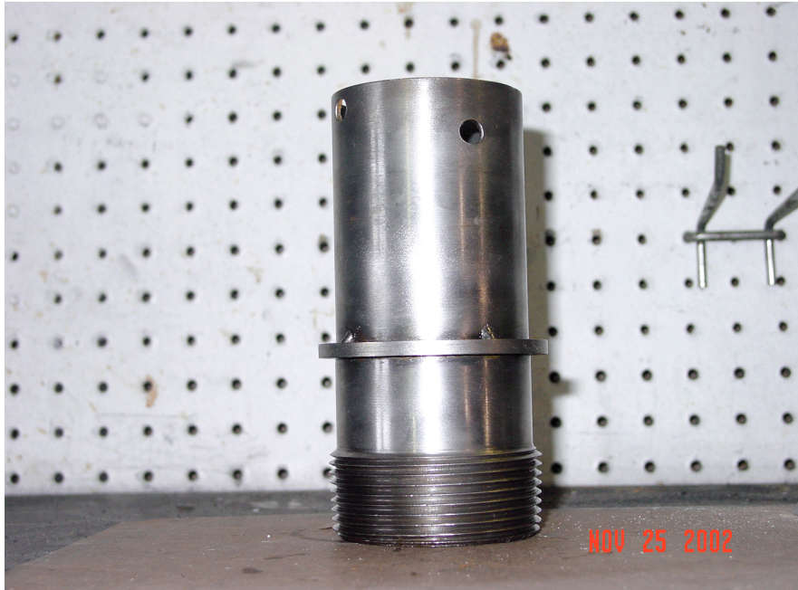
Figure 26. Mixing-Insert 1 for shotcrete nozzle body.
