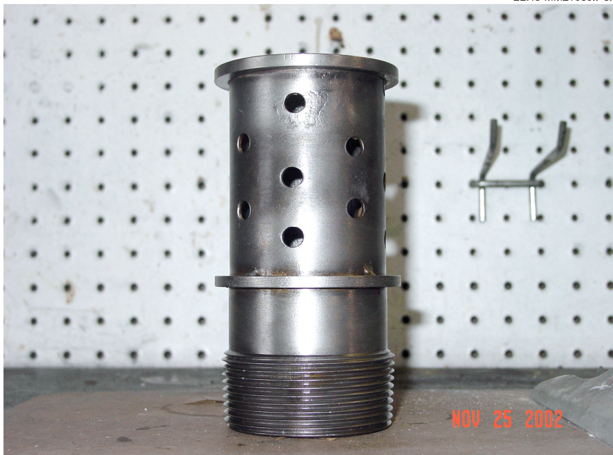
Figure 27. Mixing-Insert 2 for shotcrete nozzle body.
