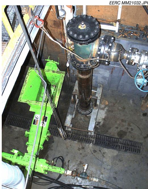
Figure 13. Pump system configured for pumping sludge into pressurized vessel – top view.
