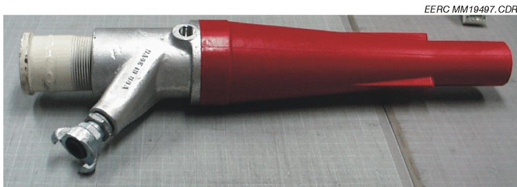
Figure 16. Shotcrete Technologies 2½-inch shotcrete nozzle.
