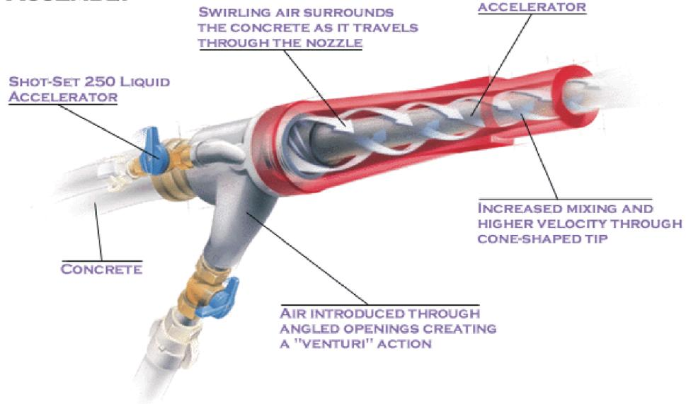
Figure 15. Cutaway diagram of Shotcrete Technologies shotcrete nozzle.
