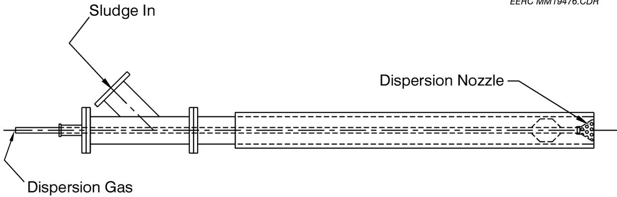
Figure 17. Sludge dispersion lance used in fluid-bed incinerator.
