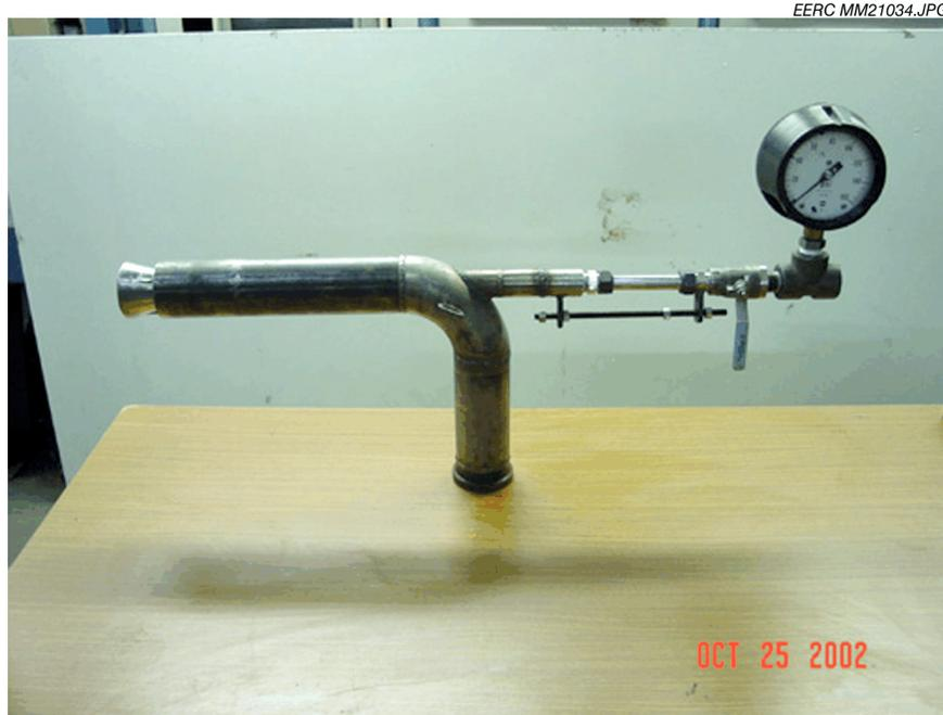
Figure 21. The EERC-2 sludge dispersion nozzle.
