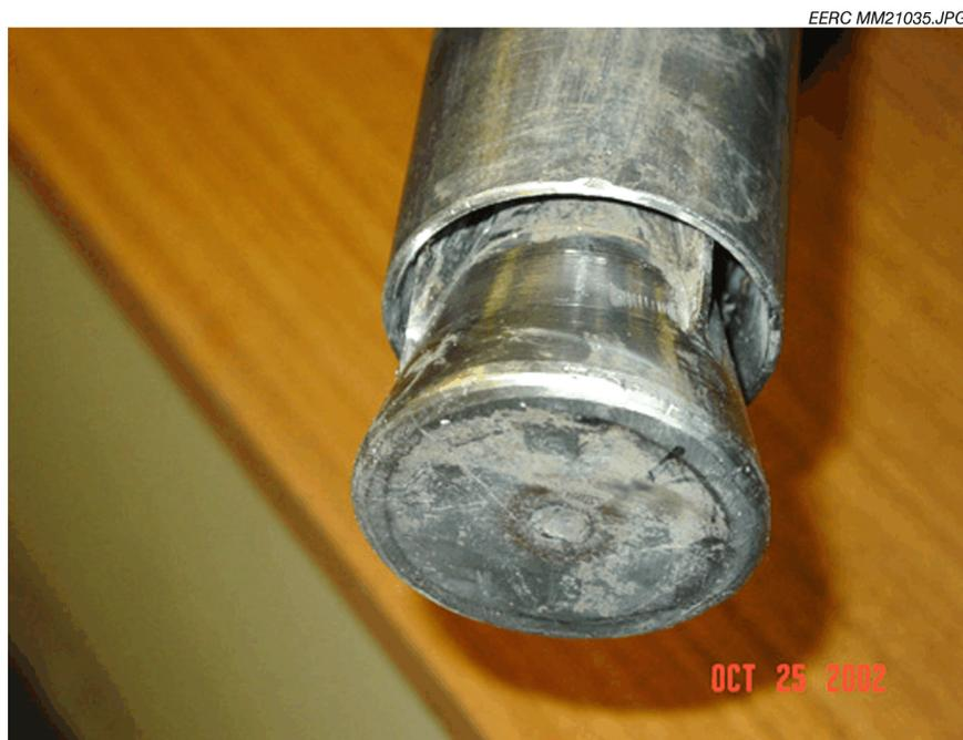
Figure 22. The EERC-2 sludge dispersion nozzle – end view.
