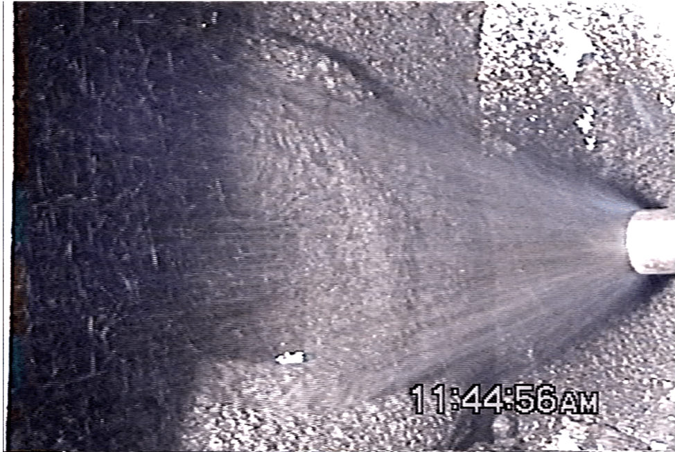
Figure B3. Sludge dispersion testing with EERC-2 nozzle.
