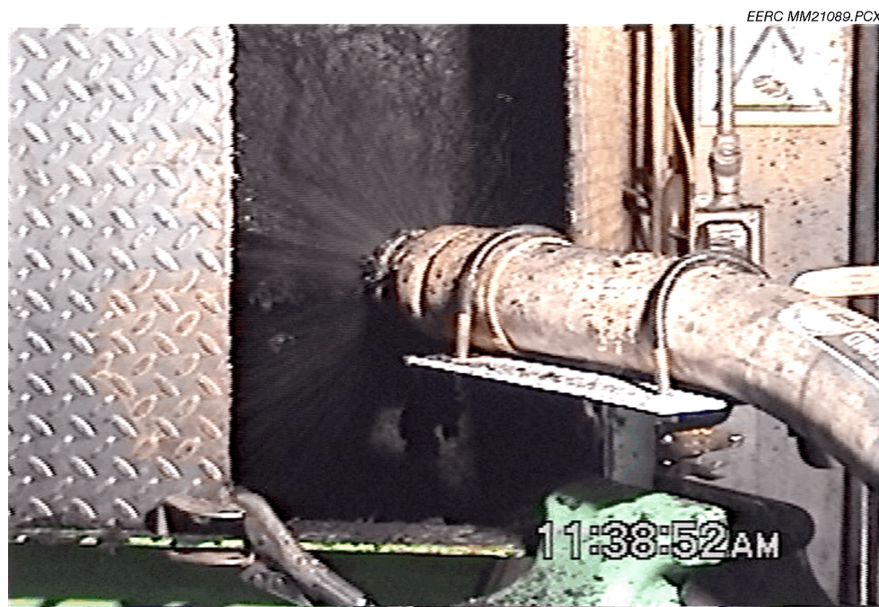
Figure B2. Sludge dispersion testing with EERC-1 nozzle.
