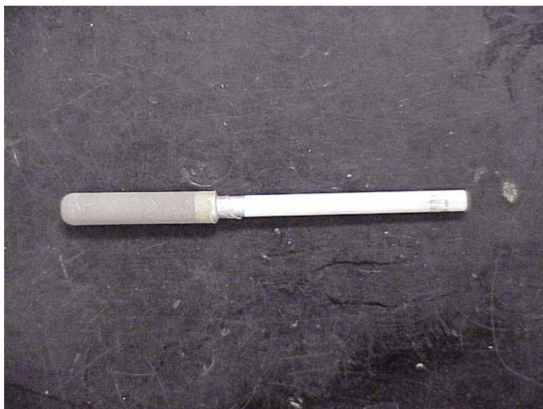
**Figure 4. Dense BCY/Ni thin film tube brazed onto a 1/4" alumina tube.**
