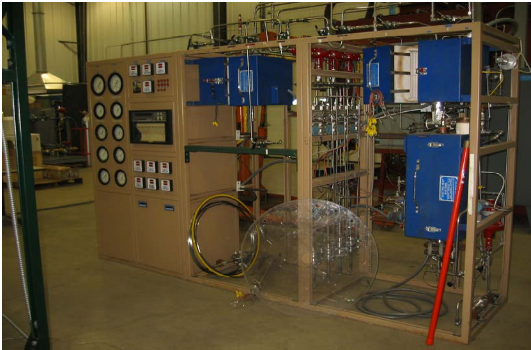
Figure 3-14. Picture of GTI Bench-Scale Catalyst Test Rig
