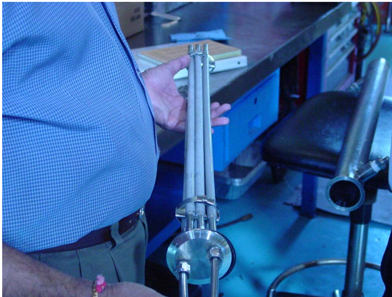
Figure 1. Typical single-pass Scepter® Micro filtration test module An all-welded module containing several filter tubes in parallel was used in the tests.
