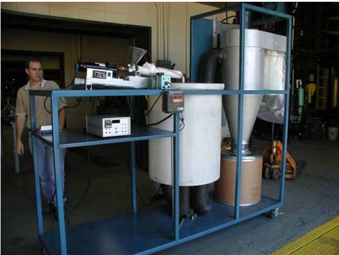
Figure 1 – Skid mounted CMS with cyclone collection system.
