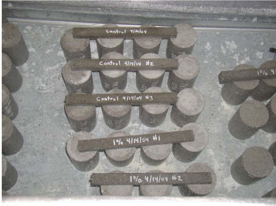
Figure 8 – Curing of CMS fiber composite mortar bars for shrinkage tests
