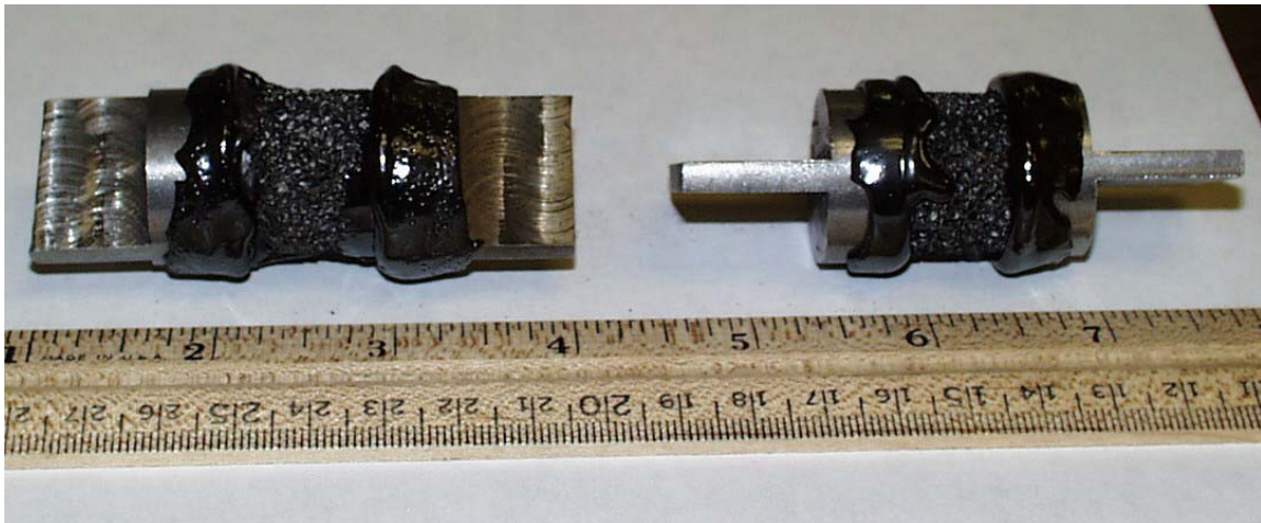
Figure 9. Foam-steel composite for tensile test.
