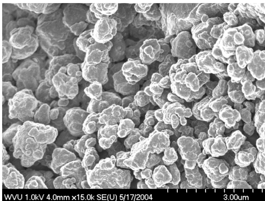
Figure 4. SEM image of ground SECO using a conventional ball mill
