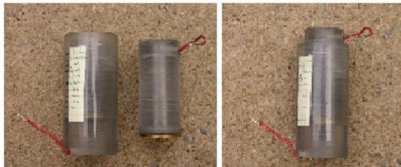
Figure 6. Electrical resistivity cell (WVU)
