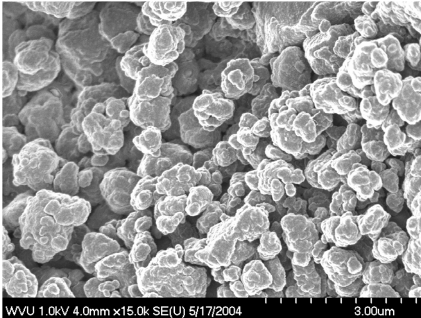
Figure 4. SEM image of ground SECO using a conventional ball mill
