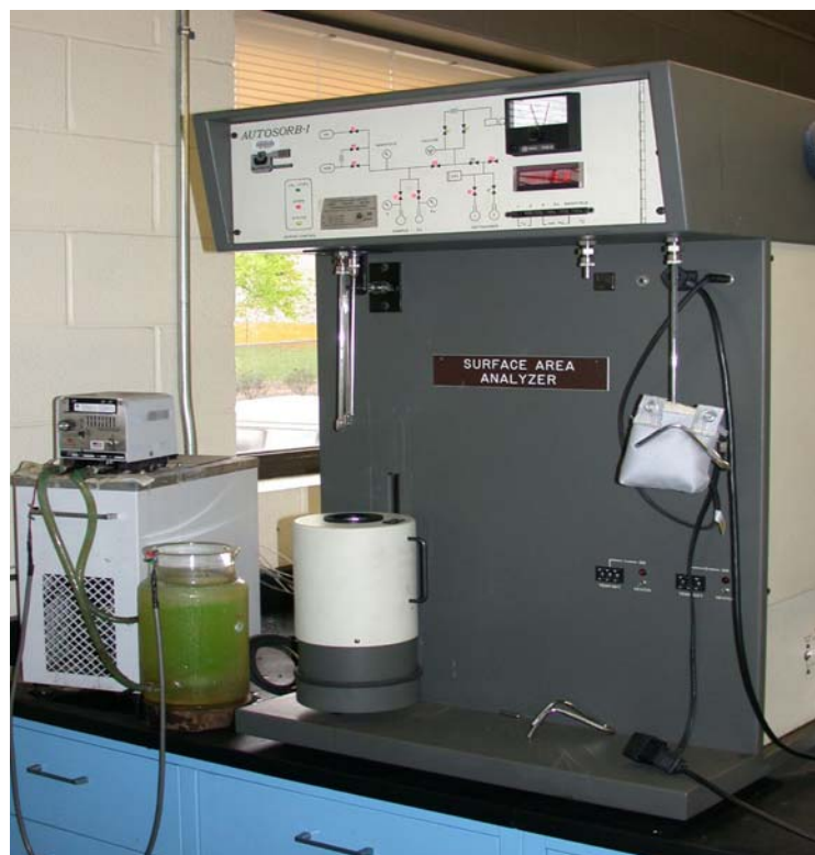
Figure 2. Quantachrome adsorption apparatus, Autosorb-1 Model ASIT.
