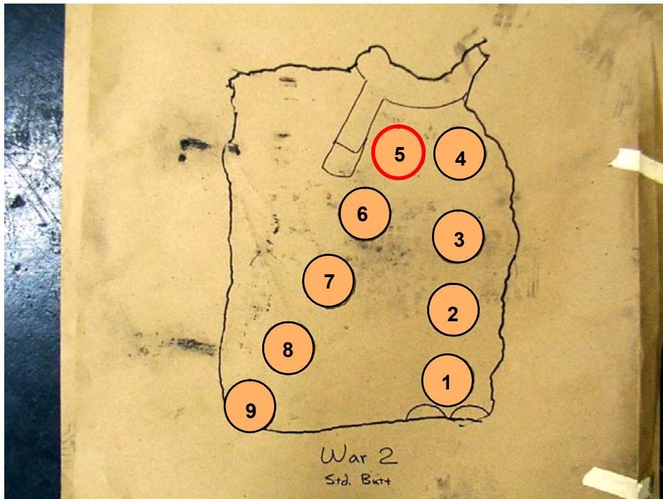
Figure 1 Position of the Core #5 in the anode butt.
