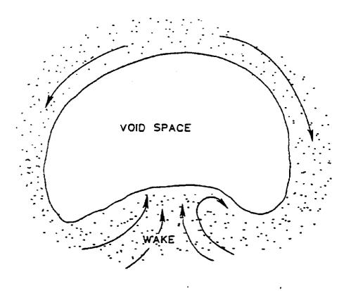
Figure 10. The pattern of solids movement in the vicinity of a void.
