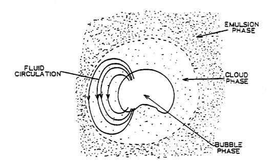
Figure 9. The gas flow pattern in the vicinity of a void.
