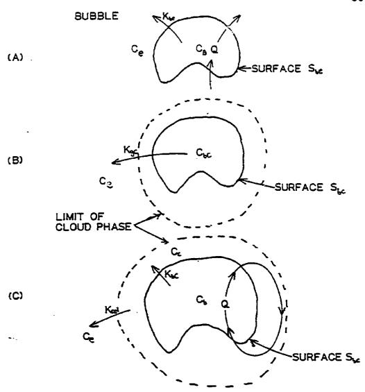
Figure 14. Three models used to represent the gas flow near a void. A. Davidson B. Partridge and Rowe C. Kunii and Levenspiel.
