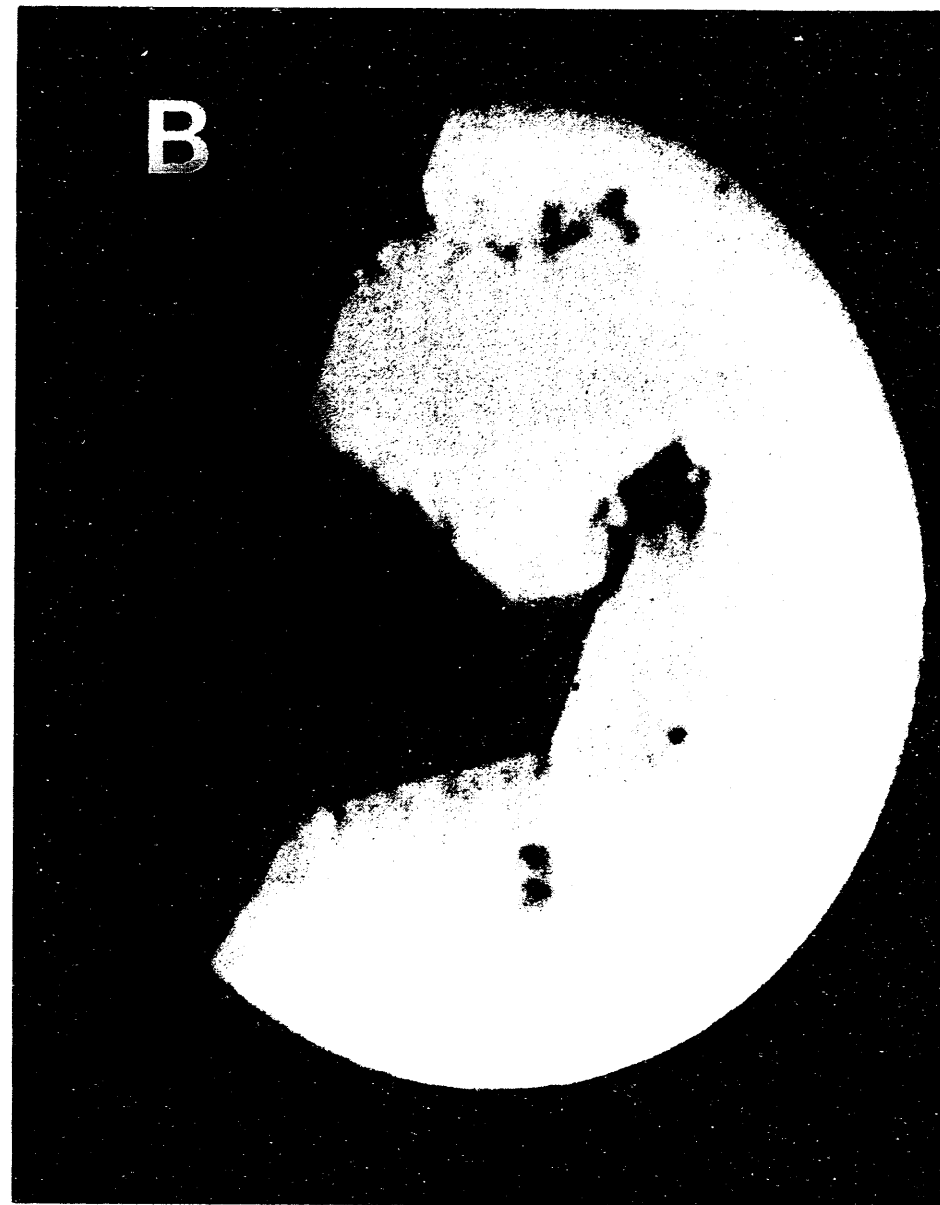
FIG. 14. Sequence of photographs taken from the CAEM video display, showing the edge recession attack of carbon in H 2 O vapor at 900 °C. The time between (a) and (b) is 3 sec. XBB 867-5379B
