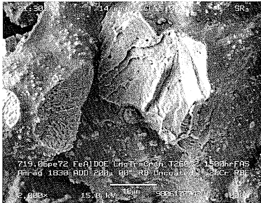
Figure 217: FAS fracture surface. Exposed for 1500 hours. Typical unexposed iron aluminide fracture surface with some porosity at sinter bond, zirconium/zirconia nodules on surface. Brittle transgranular fracture.
