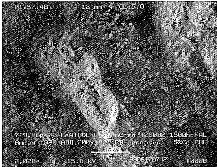
Figure 260: FAL fracture surface. Exposed for 1500 hours.
