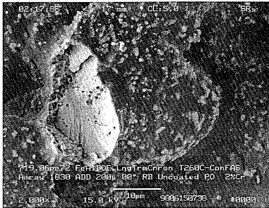
Figure 186: Fracture surface of FAS control sample. Preoxidized at 800°C. Brittle fracture of an iron aluminide sinter bond is shown. Sinter bond contains a small amount of porosity.
