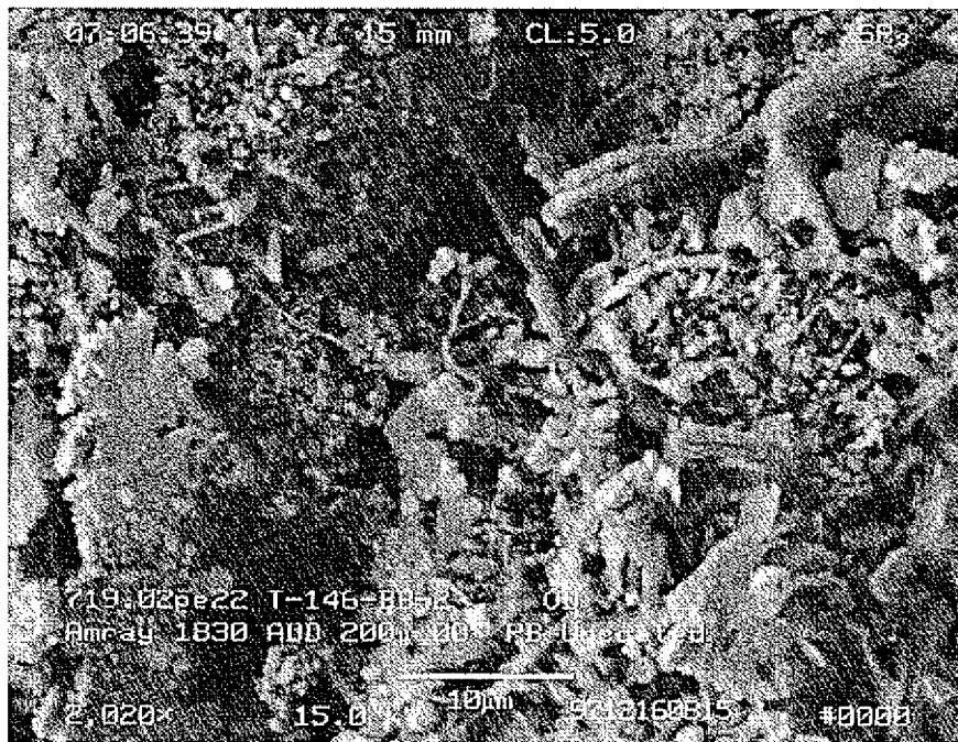
Figure 149: FAL 1000°C preoxidation, upstream surface of media. High sulfur detected using full screen spectrum. 2000X (T-146-BB-2)
