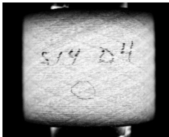
Figure 25 - Hole in membrane, detectable under transmitted light.
