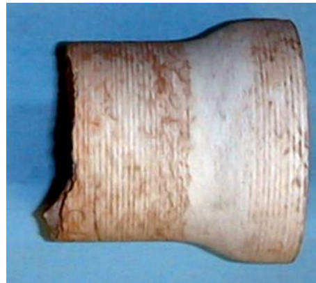
Figure 75 - C750 (B-49) with fine crack at base of tapered region of flange
