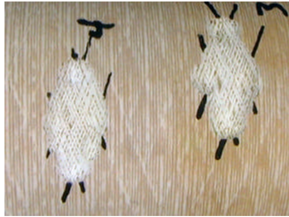
Figure 73 - Surface Damage Rating = 4
