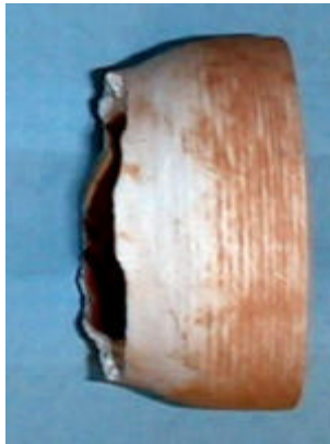
Figure 74 - C756 (T-31) broke during reinstallation
