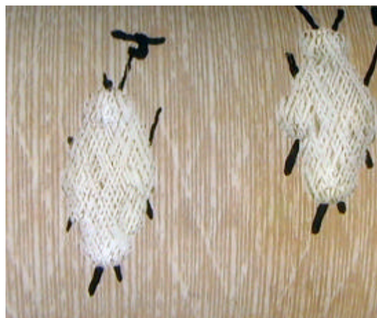
Figure 71 - Damage resulting from impact testing of Filter C740, Alumina Lot#2, 636 exposure hours
