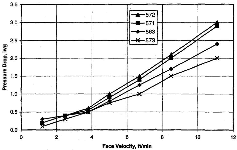
Figure 6 -- Room temperature gas flow resistance measurements of the course membrane PRD-66 candle filters.
