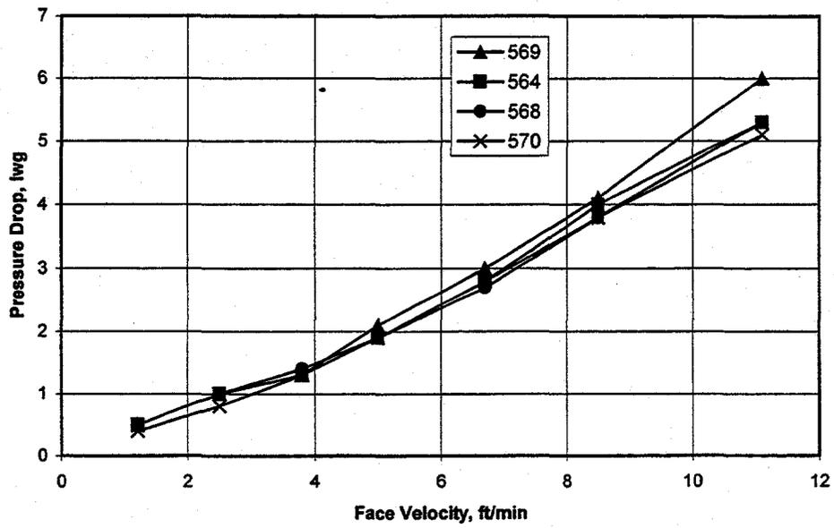
Figure 7 – Room temperature gas flow resistance measurements of the medium membrane PRD-66 candle filters.
