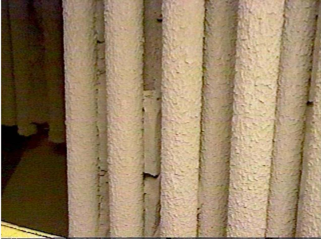
Figure 3-21. The bottom plenum was not entirely free of bridging between candles. This photograph shows a chunk of ash stuck between candles in the bottom plenum. This chunk is believed to have originated under the tubesheet in the bottom plenum.
