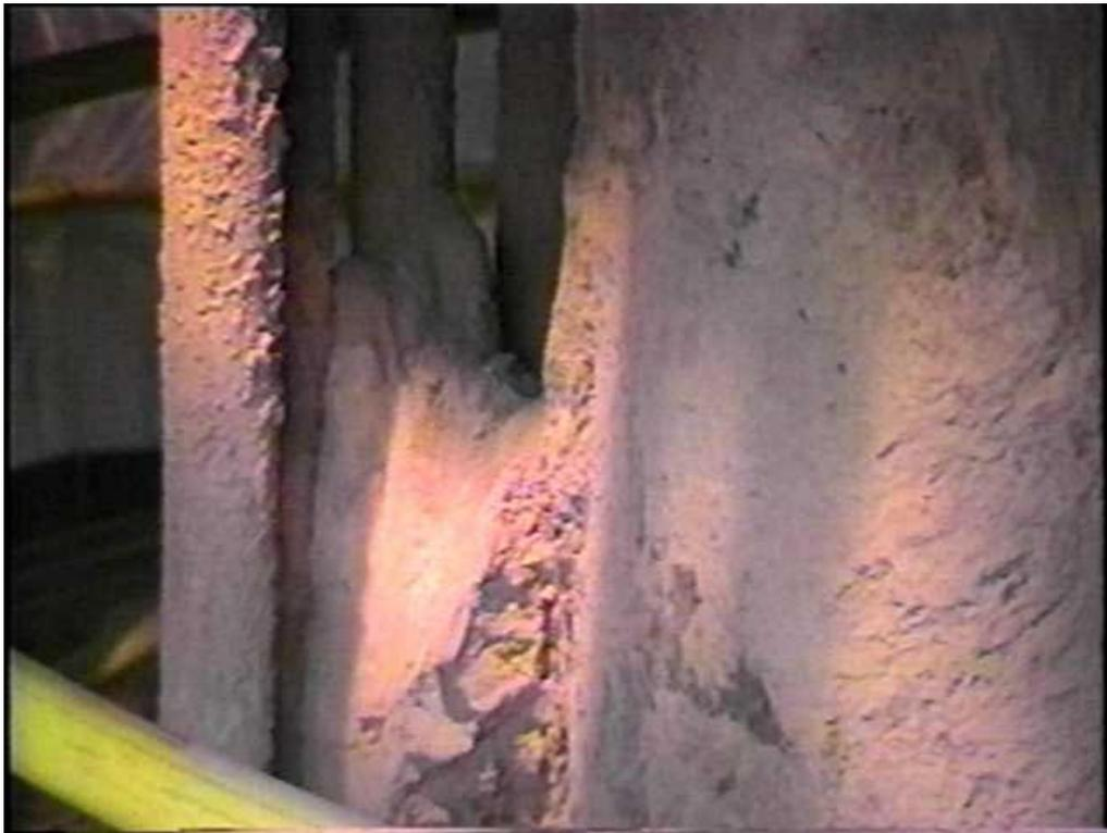
Figure 3-34. This morphology of this large ash bridge supports the conclusion that loose ash falling from above can be blocked and retained by chunks of ash previously lodged against the candles. This bridge was located near the lower end of the filter elements just above the conical surface of the ash shed.
