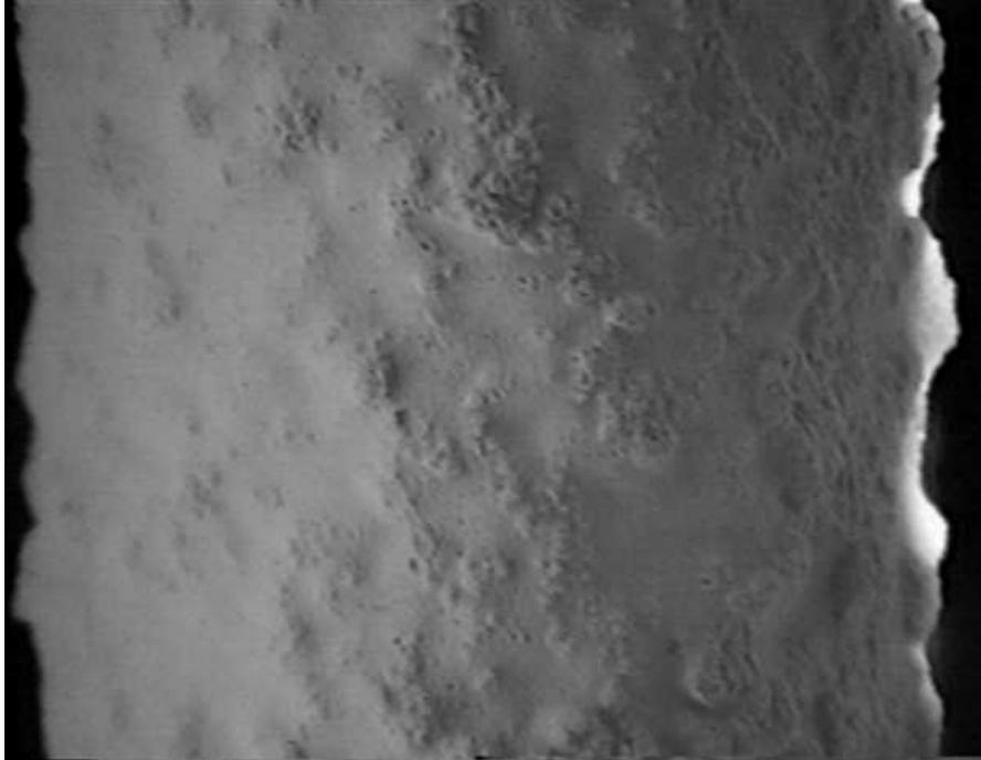
Figure 3-75. A representative photograph of the appearance of the smoothest filter cakes observed in the Siemens Westinghouse FL0301 filter at the PSDF on January 20, 1998. Small pinholes are distributed over the surface of the cake.
