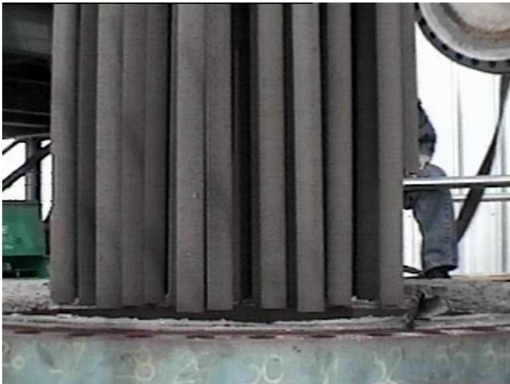
Figure 3-56. The lower plenum clearing the filtration vessel.
