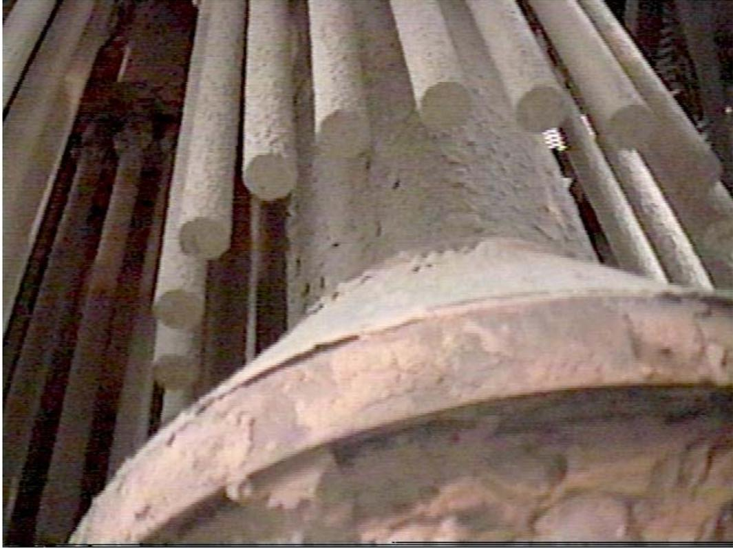
Figure 3-48. The ash sheds remained relatively clean during this run.
