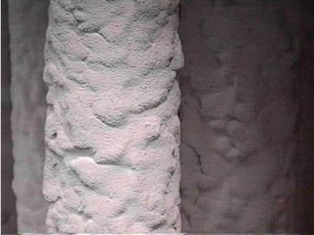
Figure 3-92. Another view of lumpy filter cakes observed in the top plenum on January 26, 1999.
