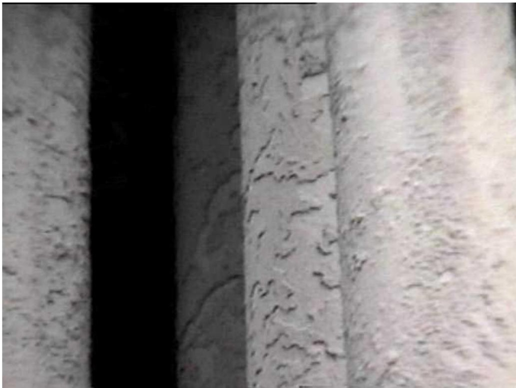
Figure 3-58. Typical patchy cakes observed on the filter elements.
