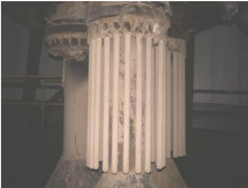
Figure 3-49. The intact elements in the top plenum remained clean.
