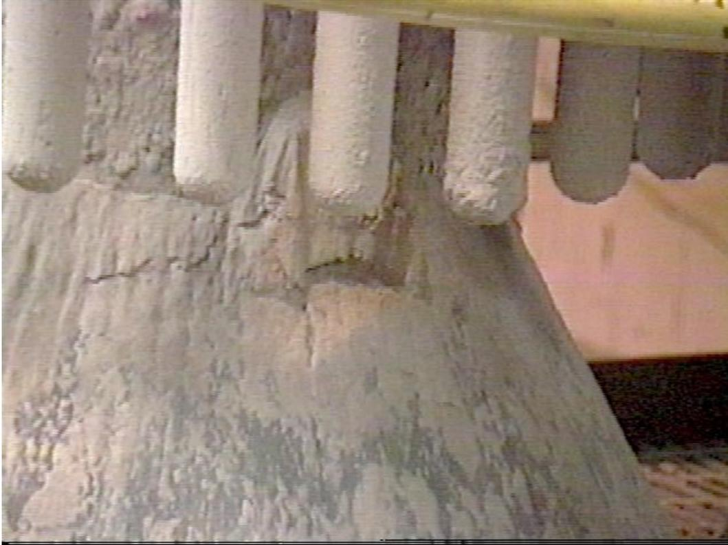
Figure 3-42. Only minor deposits were present on the ash shed below the top plenum.
