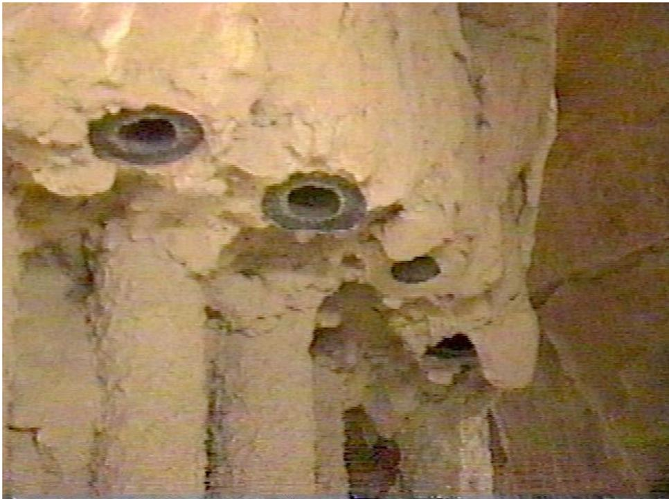
Figure 3-18. Two types of fracture surfaces are seen here. The relatively clean fracture surfaces on the two elements in the foreground indicate that these elements broke following operation. The ash-covered fracture surface of the element just to the right of the aforementioned elements indicates that this element broke before operation was discontinued.
