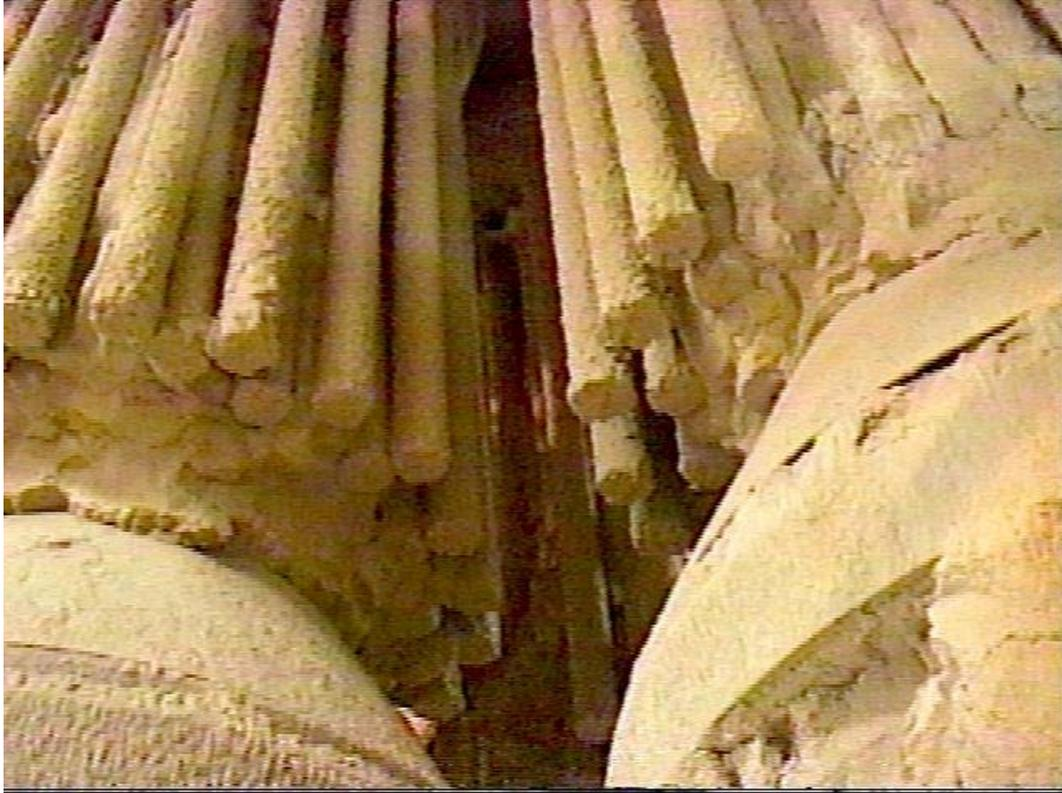
Figure 3-15. Bridging adjacent to the central support columns was pervasive.
