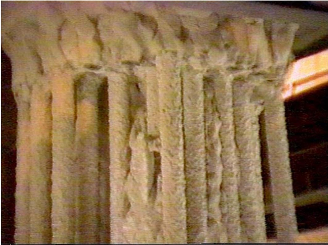
Figure 3-13. Close up of ash bridges and tubesheet deposits.
