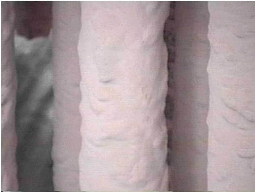
Figure 3-89. Close up of a filter cake in the top plenum (January 26, 1999).
