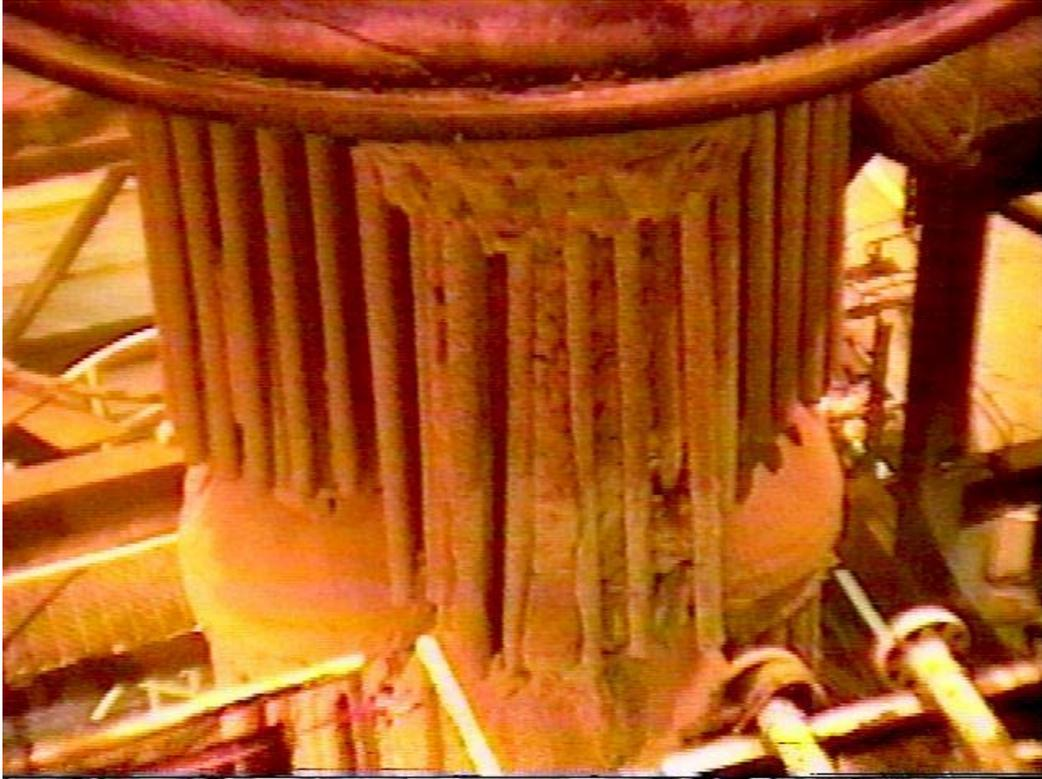
Figure 3-7. Severe bridging and candle deformation in the top plenum.
