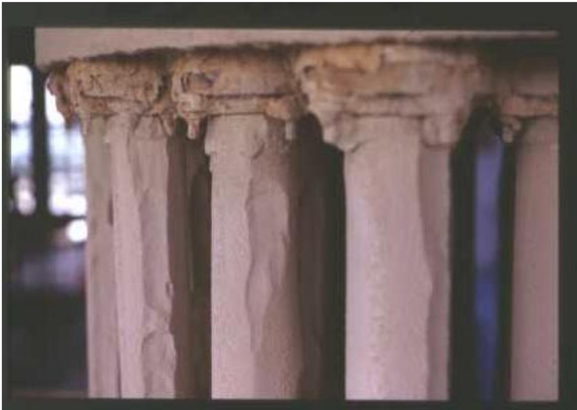
Figure 3-61. Upper portion of candles showing impaction ridges in the filter cakes.
