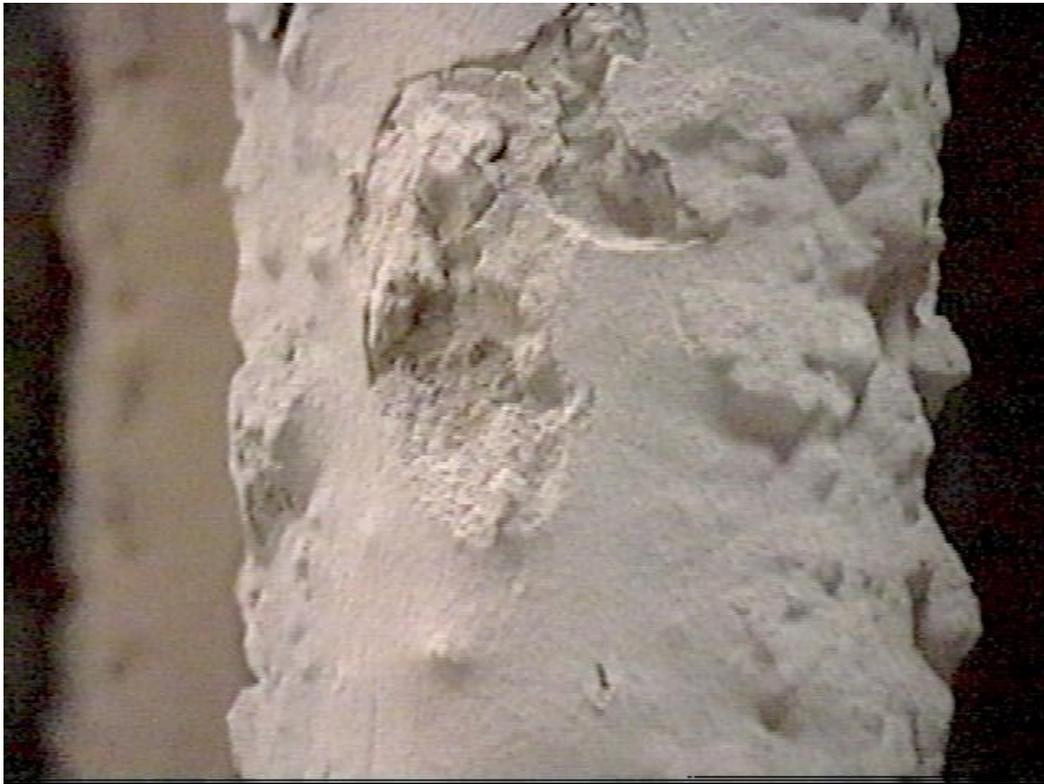
Figure 3-45. Many of the filter cakes were moderately thick and irregular in shape.
