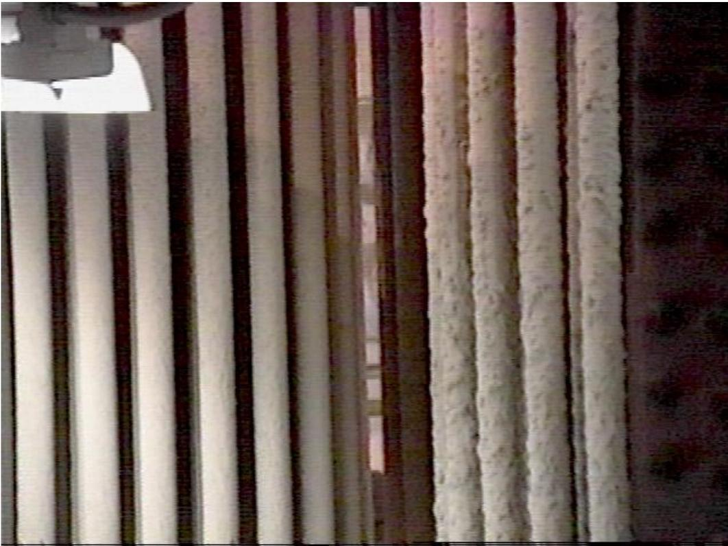
Figure 3-43. The distinctly different appearances of the filter cakes on these two filter arrays in the bottom plenum are believed to be a result of different element types.
