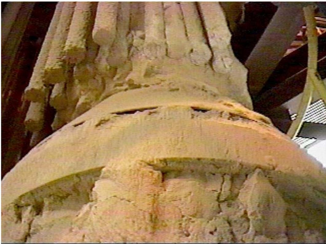
Figure 3-16. In addition to deposits adjacent to the support columns, large, strong agglomerates formed around the regions where the candles were attached to the tubesheet.
