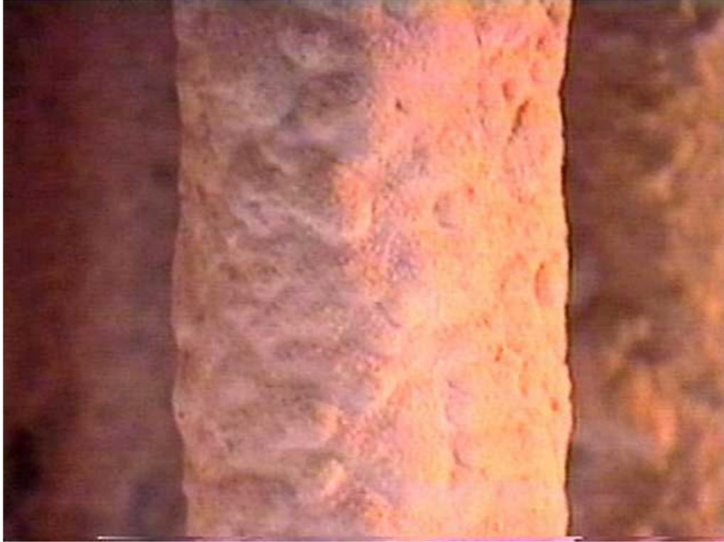
Figure 3-86. Close up of filter cake in the top plenum (January 26, 1999).
