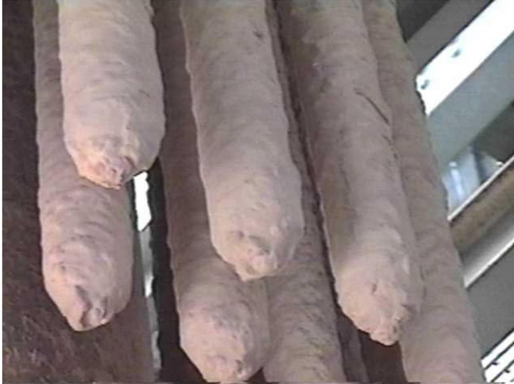
Figure 3-88. Lower portion of filter elements in the top plenum (January 26, 1999).
