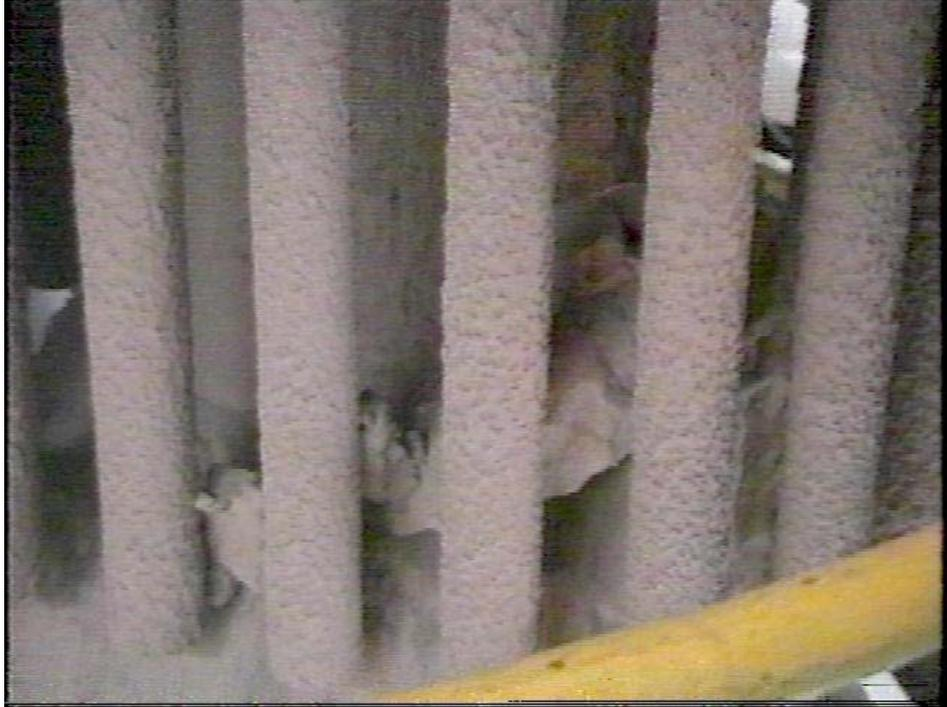
Figure 3-35. Chunks of ash that get trapped between candles (as shown here) appear to provide the initial conditions for development of bridges between adjacent filter elements. Ash removed during cleaning pulses piles on top of these trapped chunks instead of falling into the hopper for removal.
