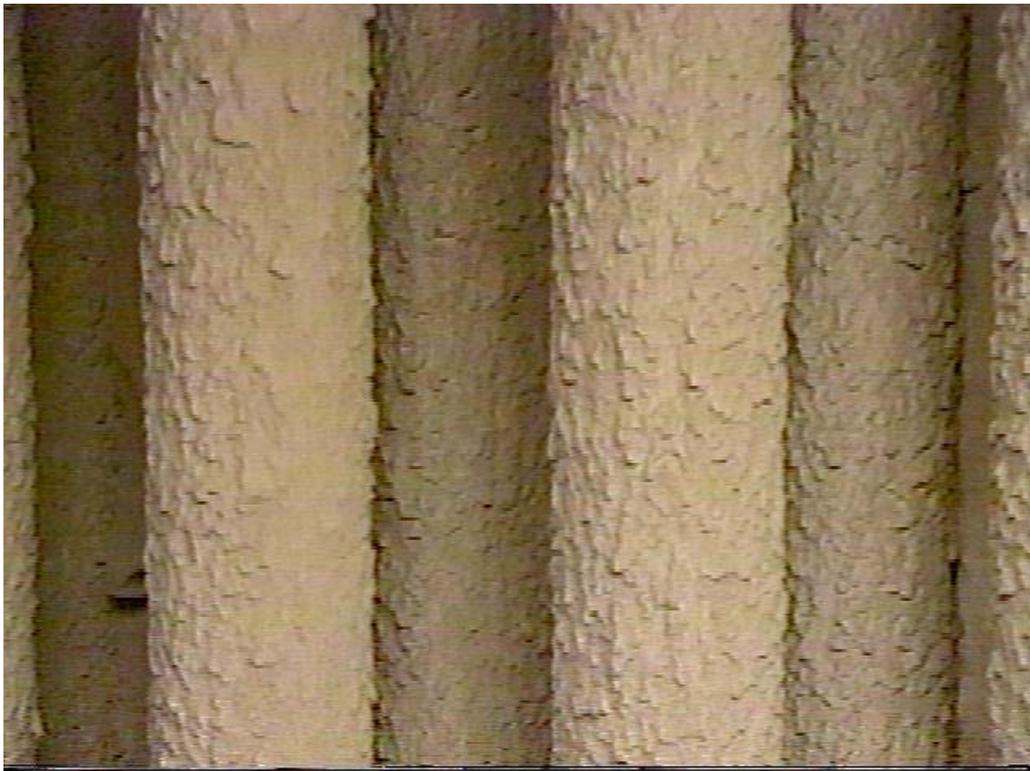
Figure 3-22. Close up of the filter cakes in the bottom plenum.
