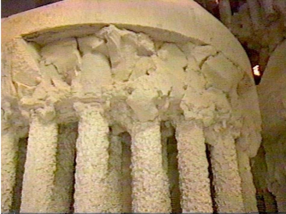
Figure 3-19. Large ash deposits were common under the tubesheet. This photograph also shows the general appearance of the filter cakes.
