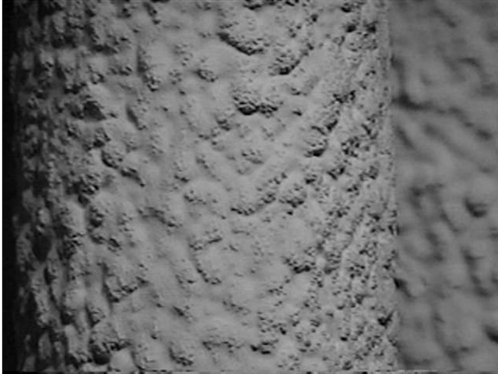
Figure 3-74. A representative photograph of the appearance of a relatively smooth filter cake observed in the Siemens Westinghouse FL0301 filter at the PSDF on January 20, 1998.
