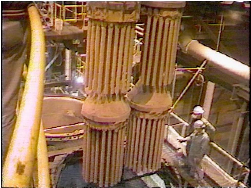
Figure 3-30. General condition of middle and bottom plenums as they were transported to the inspection platform.
