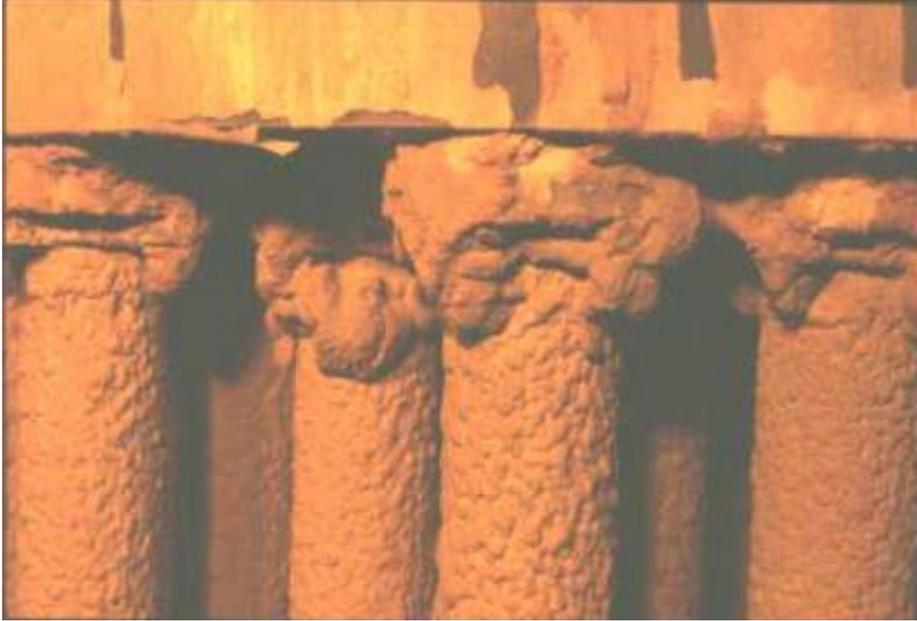
Figure 3-70. Deposits observed around the top of the filter elements.
