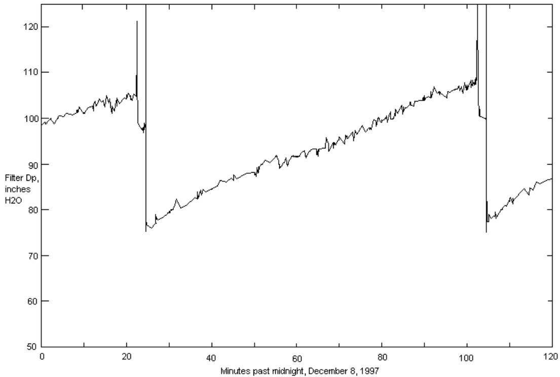
Figure 3-68. Pressure drop data from FL0301 operation early on December 8, 1997.
