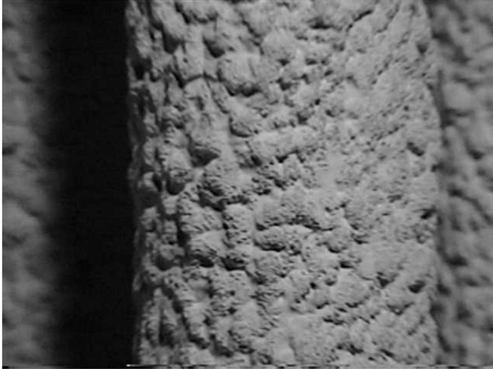
Figure 3-72. A representative photograph of the appearance of the majority of the filter cakes observed in the Siemens Westinghouse FL0301 filter at the PSDF on January 20, 1998.
