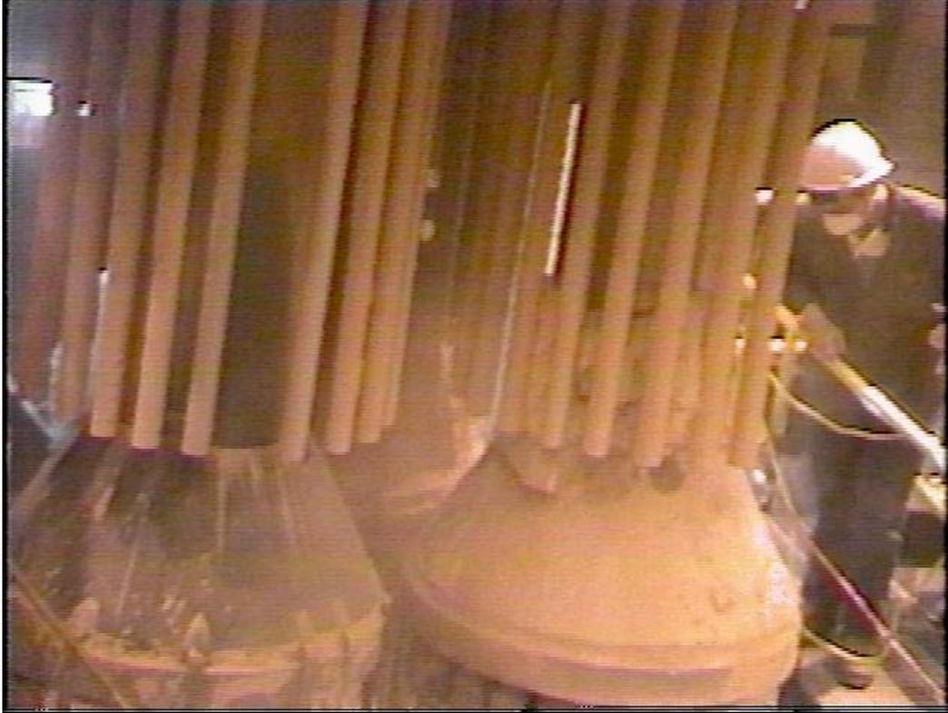
Figure 3-25. The top plenum experienced some bridging and broken elements.
