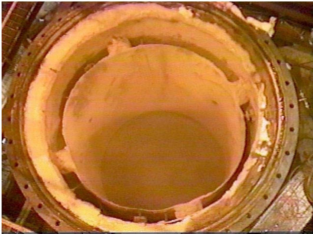
Figure 3-12. The interior of the filter vessel and the shroud after removal of the plenum assembly.
