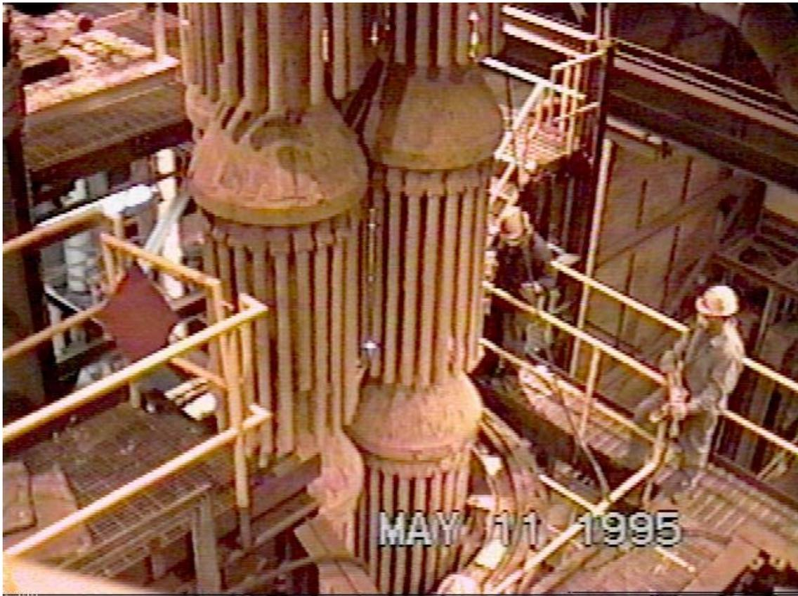
Figure 3-37. The filter assembly was basically free of bridges and most of the elements were intact when the assembly was removed from the filtration vessel.
