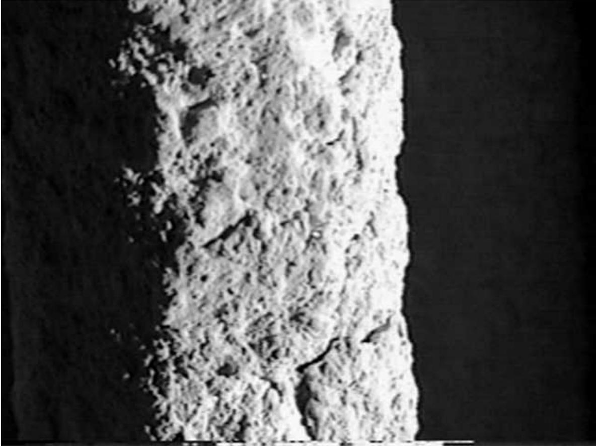
Figure 3-76. A representative photograph of the appearance of a passive ash deposit formed on a set of stacked samples of various filter element materials located within the array of candle filter elements. This deposit was observed in the Siemens Westinghouse FL0301 filter at the PSDF on January 20, 1998.
