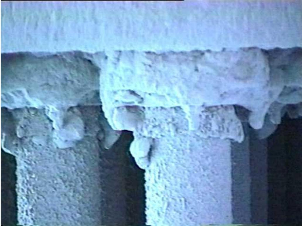
Figure 3-65. More deposits around the top of the filter elements. The blue color in this photograph was caused by blue tarps surrounding the inspection platform.
