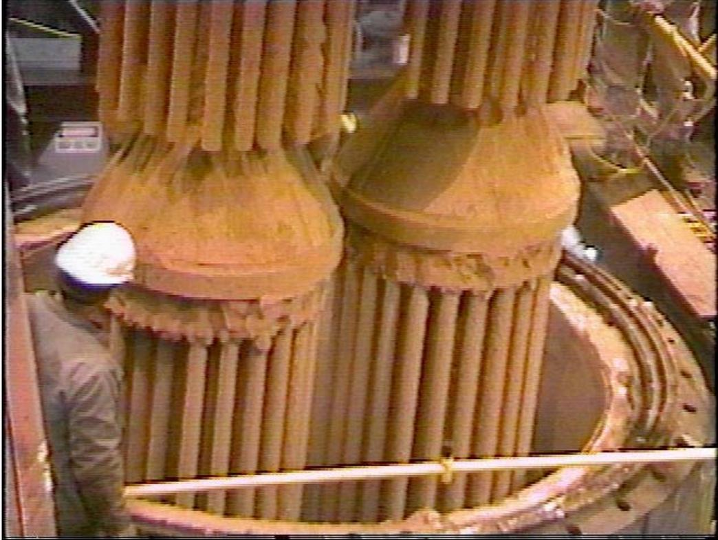
Figure 3-27. This photograph shows the general condition of the bottom and middle plenums as they were lifted from the filter vessel.
