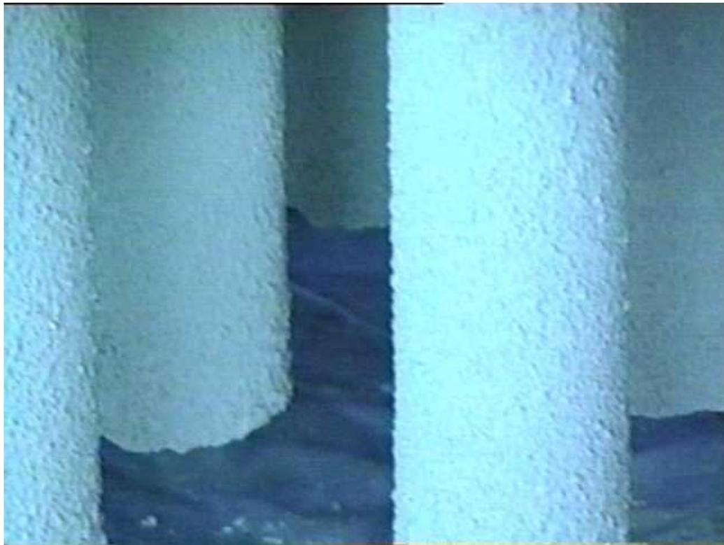
Figure 3-64. Lower portion of some of the candles on the lower plenum. The blue color in this photograph was caused by blue tarps surrounding the inspection platform.
