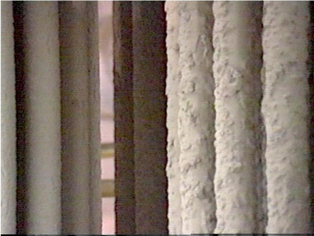
Figure 3-44. Close up of filter cakes in the bottom plenum.
