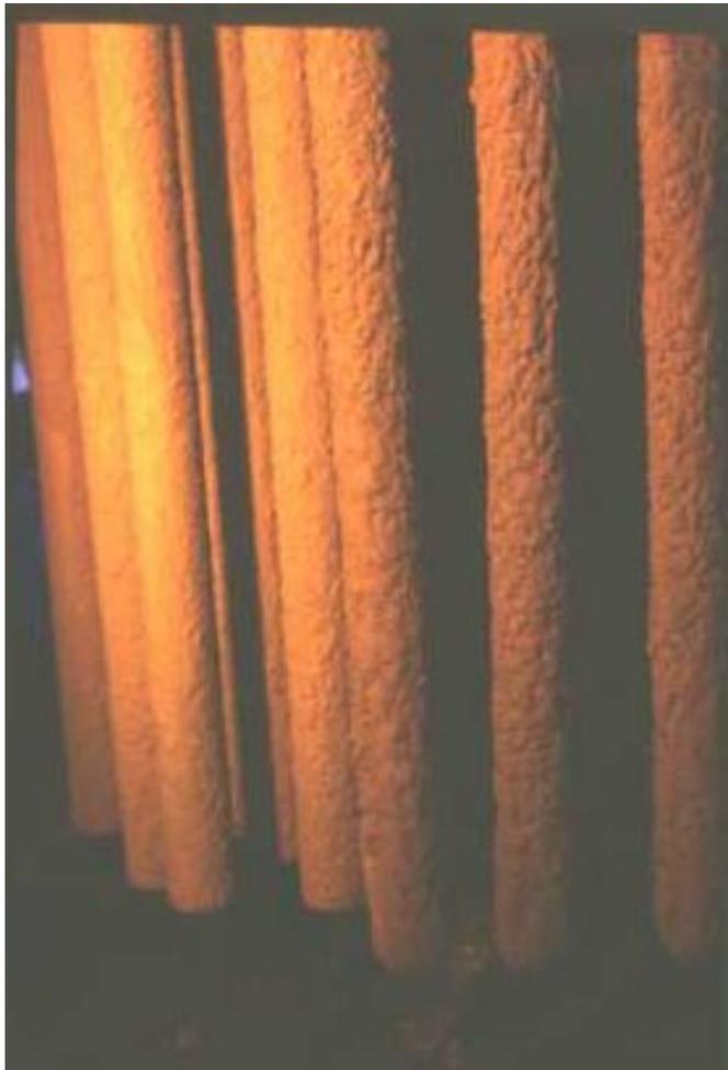
Figure 3-71. Typical appearance of the lower portion of the filter elements.
