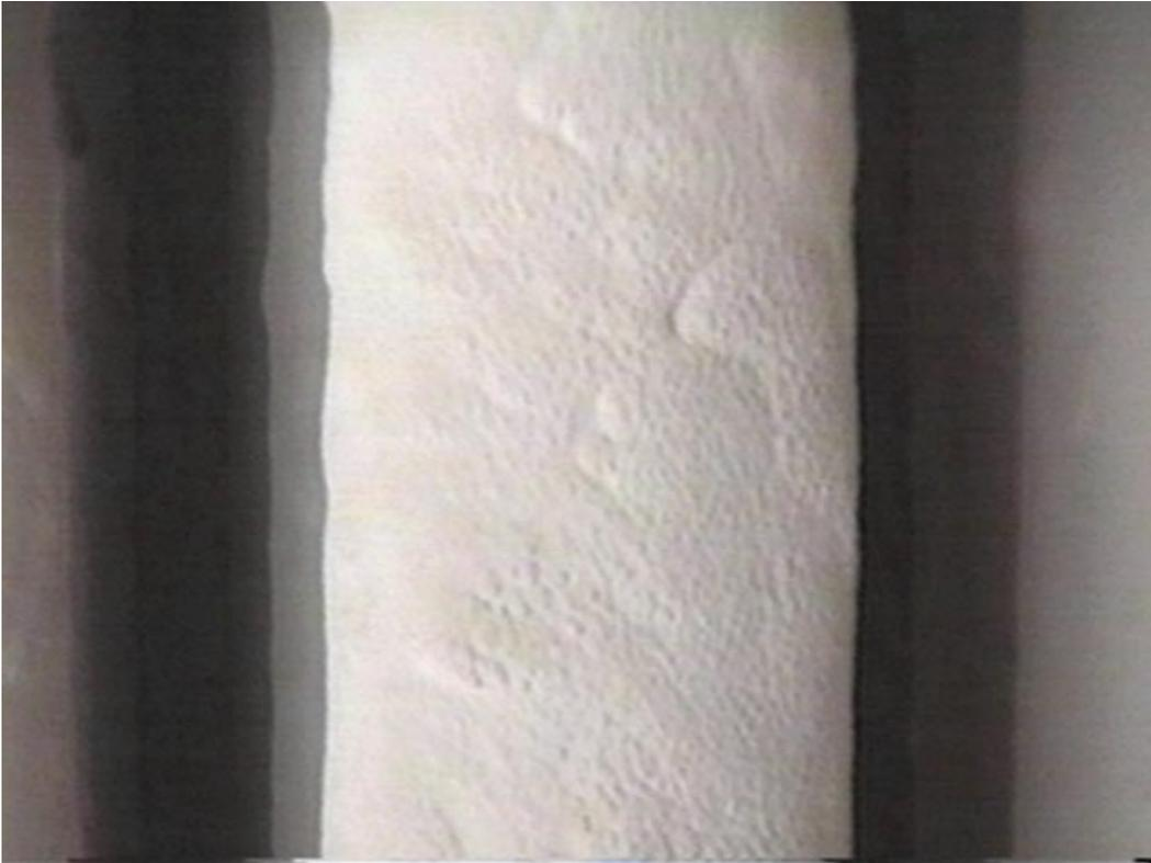
Figure 3-79. Typical smooth filter cakes observed on the bottom filter plenum at the PSDF on May 18, 1998.
