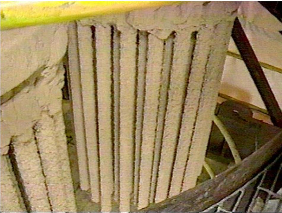
Figure 3-20. The candles in the bottom plenums were relatively free of bridges, presumably because these plenums had no support columns in the center of the arrays of elements. (Deposits formed by turbulent diffusion on the central columns in the upper plenums. These deposits grew unabated, and significantly contributed to the problems that were common in the upper plenums.)
