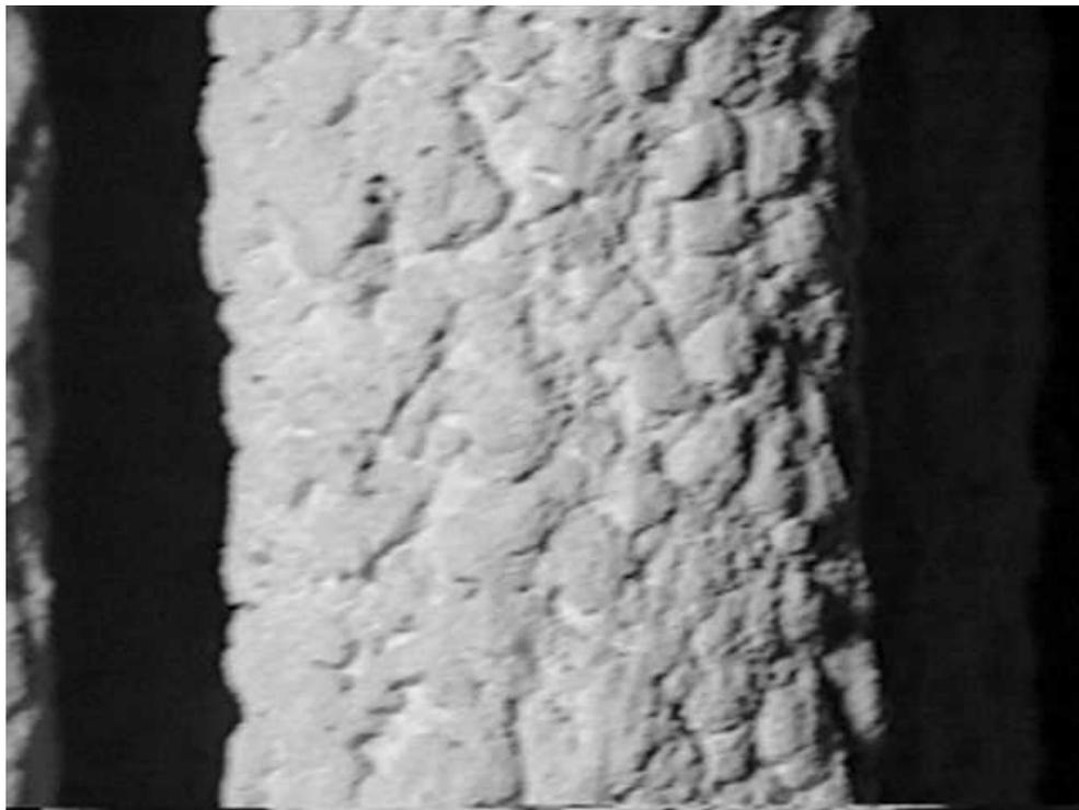
Figure 3-73. A representative photograph of the appearance of one of the lumpier filter cakes observed in the Siemens Westinghouse FL0301 filter at the PSDF on January 20, 1998.
