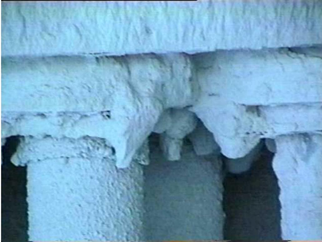
Figure 3-63. Filter cakes and deposits at the top of the filter elements. The blue color in this photograph was caused by blue tarps surrounding the inspection platform.
