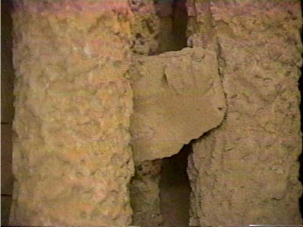
Figure 3-23. At various places large ash deposits were found lodged between filter elements.
