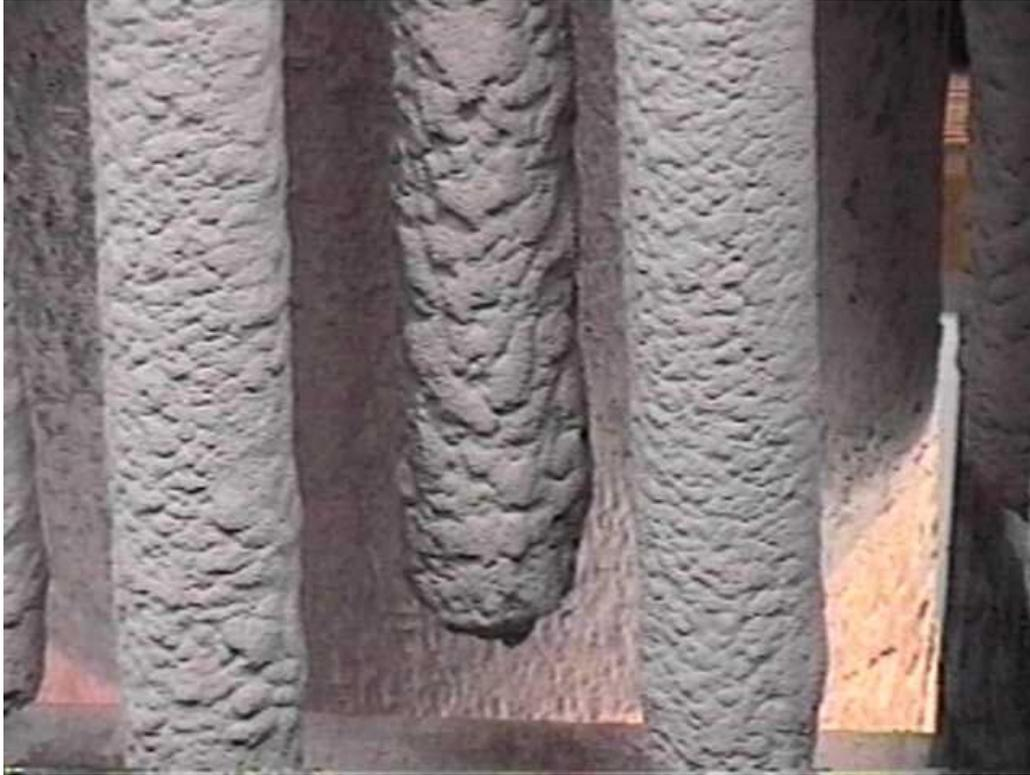
Figure 3-90. Lower portion of the filter elements in the top plenum (January 26, 1999).
