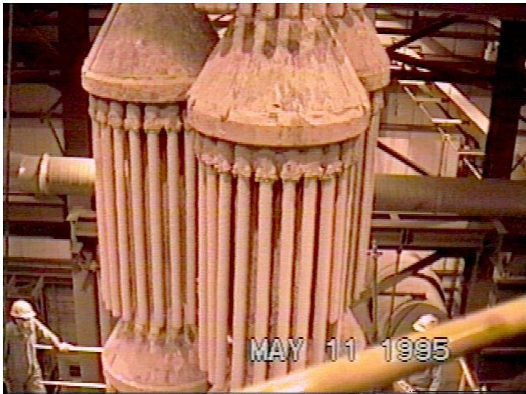
Figure 3-39. The middle plenum assembly was clean and the filter elements were intact.
