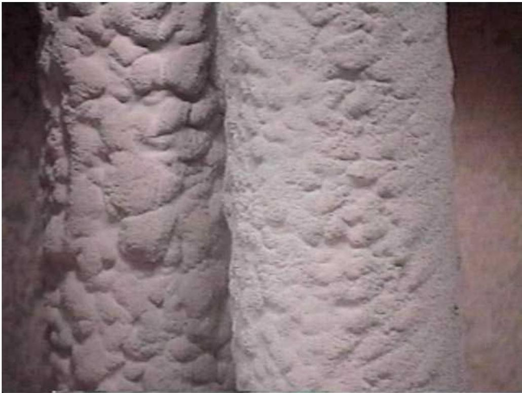
Figure 3-91. Many of the filter cakes observed in the top plenum on January 26, 1999 had a lumpy appearance.
