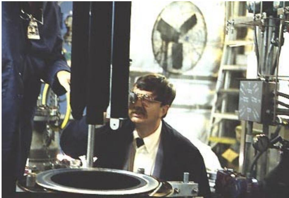
Figure 3-52. Microscopic examination of the filter cakes was used to determine their thickness.
