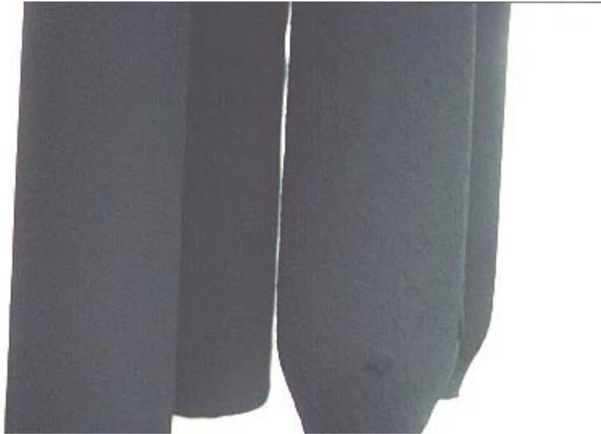
Figure 3-51. Lower portion of the four candles removed from the MGCR filter vessel. Each element was covered with a thin, black filter cake that was smooth and fluffy.
