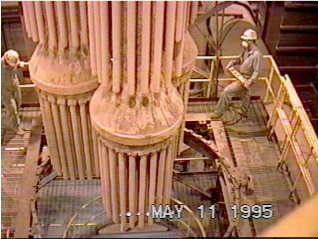
Figure 3-40. The bottom plenum was clean and the filter elements were intact. The filter assembly is being lowered onto the inspection platform.
