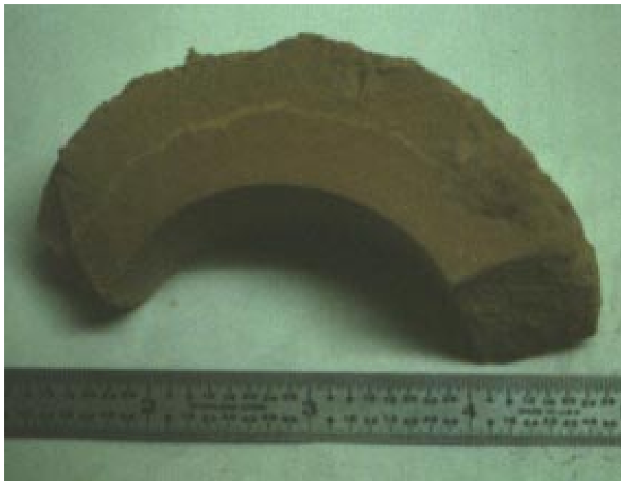
Figure 3-6. A number of laboratory analyses were performed on this thick filter cake deposit (ID # 4012). The deposition layers formed during filtration are clearly visible in this specimen.
