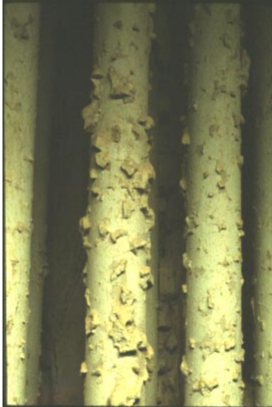
Figure 3-5. The appearance of these candles is believed to be the result of patchy cleaning and the loss of cake during cooling down of the filter vessel.
