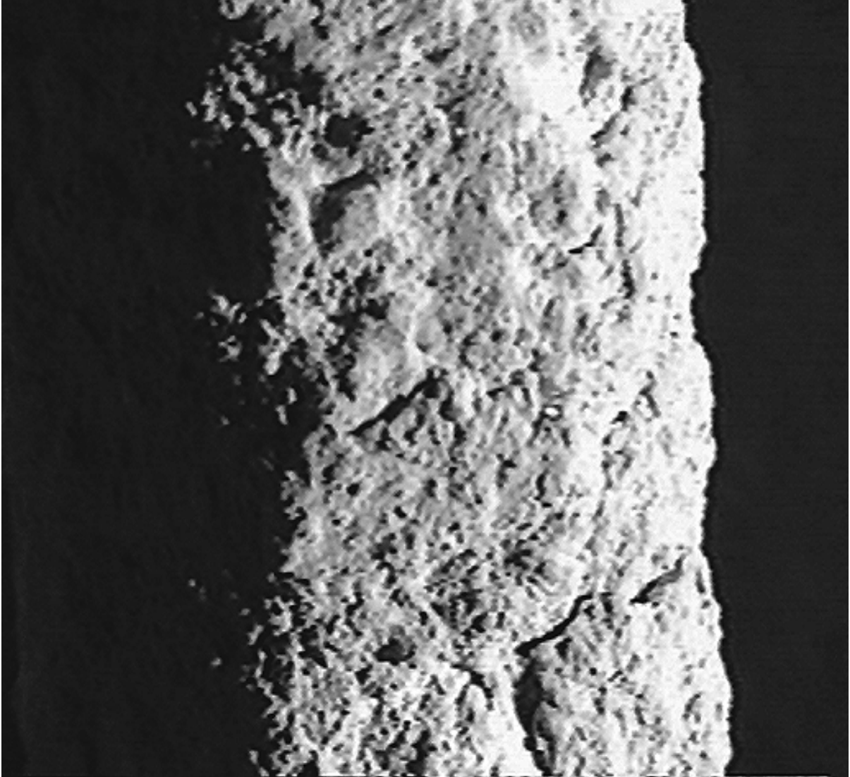
Figure 5. A representative photograph of the appearance of a passive ash deposit formed on a set of stacked samples of various filter element materials located within the array of candle filter elements. This deposit was observed in the Westinghouse FL0301 filter at the PSDF on January 20, 1998.
