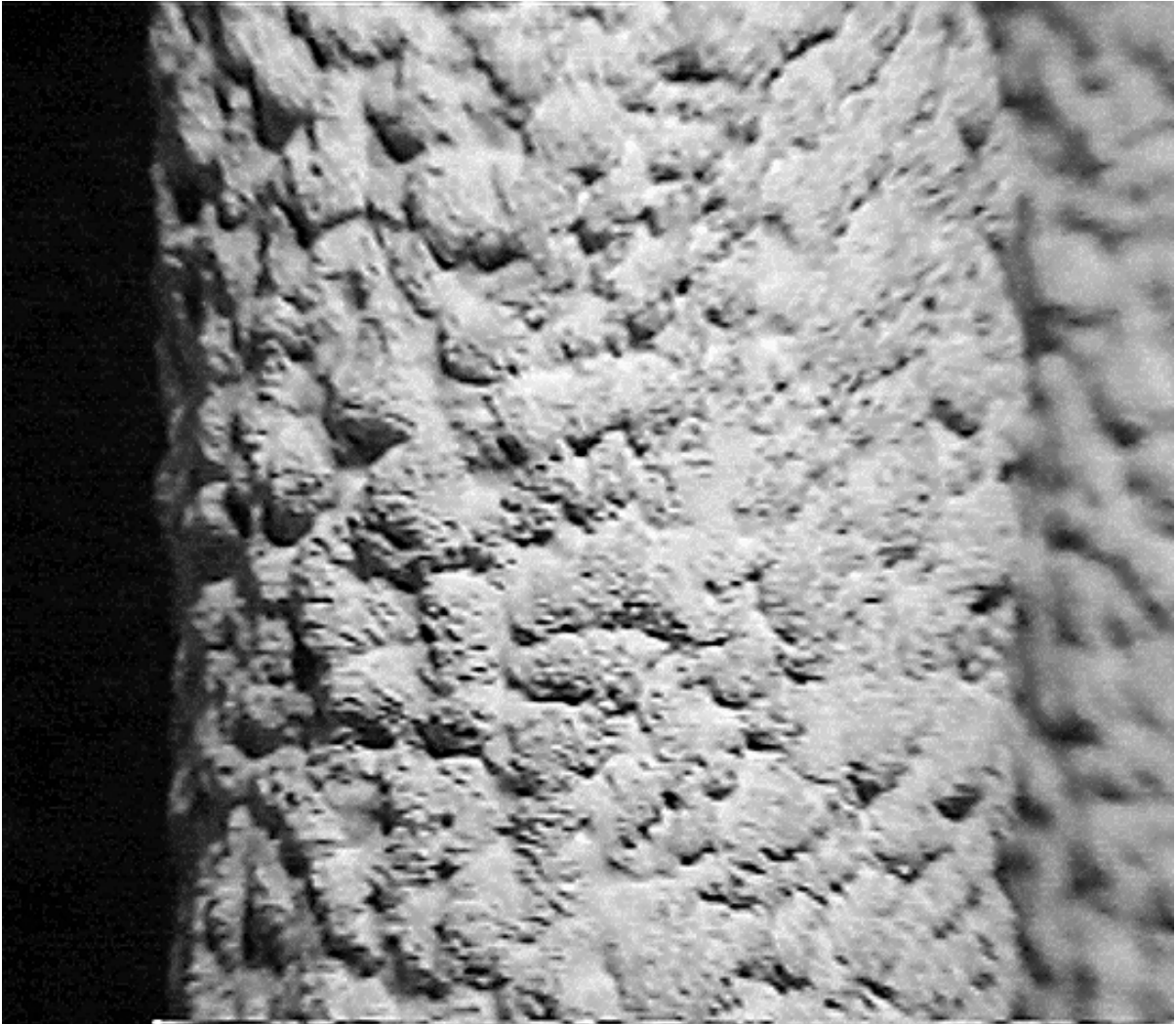
Figure 1. A representative photograph of the appearance of the majority of the filter cakes observed in the Westinghouse FL0301 filter at the PSDF on January 20, 1998.
