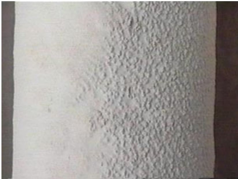
Figure 7. Typical smooth filter cakes observed on the bottom filter plenum on May 18, 1998.
