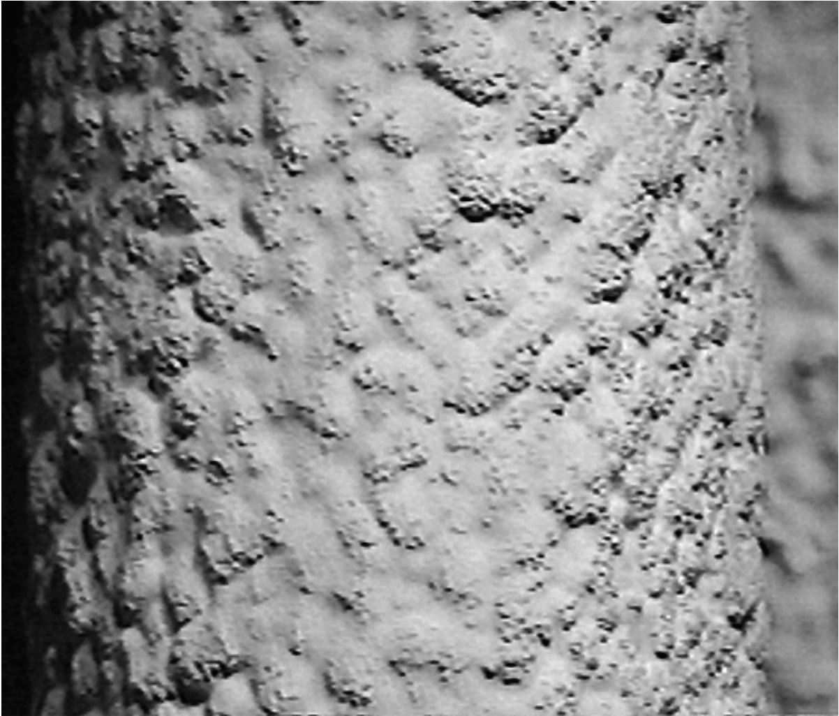
Figure 3. A representative photograph of the appearance of a relatively smooth filter cake observed in the Westinghouse FL0301 filter at the PSDF on January 20, 1998.
