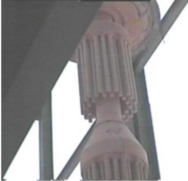
Figure 6. Appearance of the entire filter assembly on May 18, 1998 during removal from the filter vessel.
