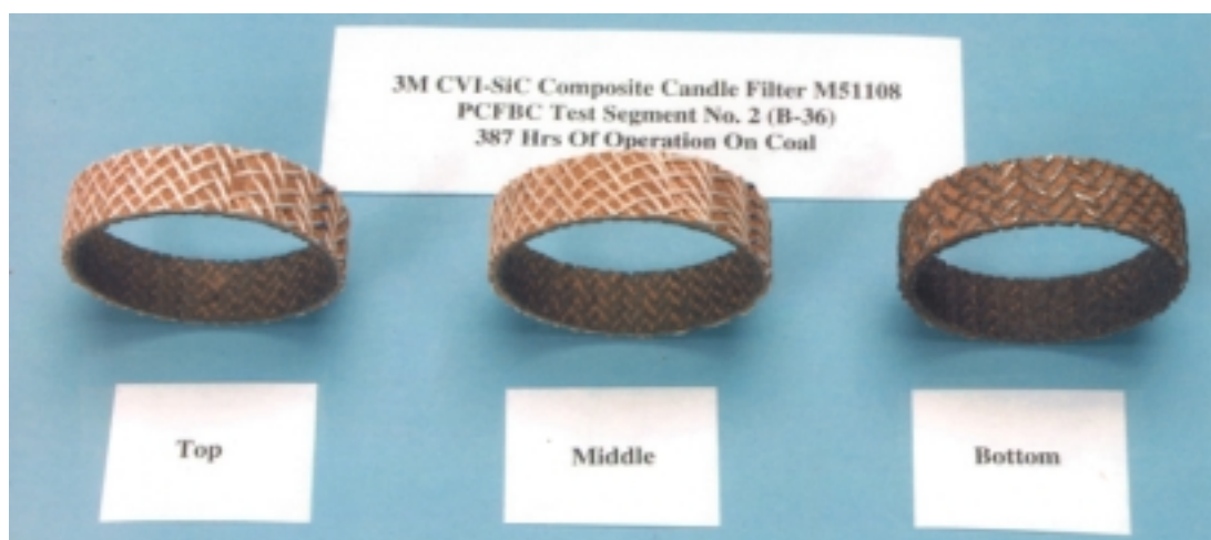
Figure 3.8 — Removal of the CVI-SiC coating along the outer confinement layer of the 3M CVI-SiC composite filter element after 387 hours of operation at AEP.
