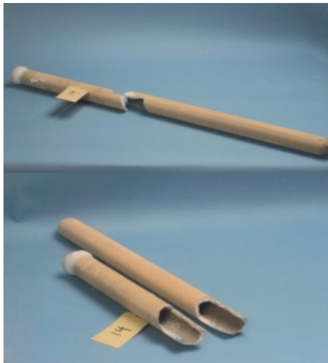
Figure 4.7 — Failure of the Scapa Cerafil™ filter element during Siemens Westinghouse simulated PFBC qualification testing.
