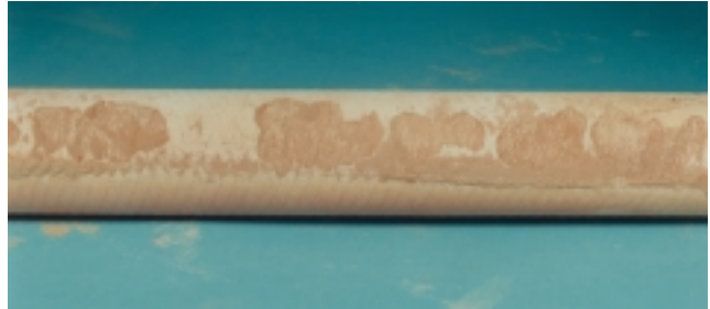
Figure 3.10 — Divot formations along the length of the DuPont PRD-66 filter elements after testing at AEP.
