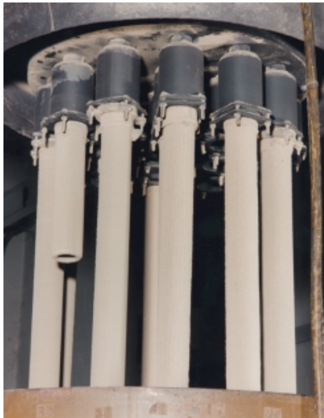
Figure 4.2 — Filter array at the conclusion of Siemens Westinghouse qualification testing.
