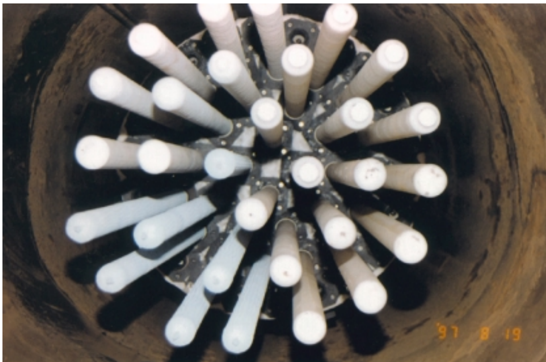
Figure 4.9 — Advanced composite filter element testing at the Foster Wheeler test facility in Karhula, Finland.
