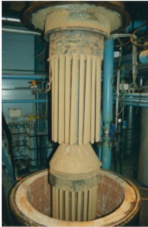
Figure 4.11 — Siemens Westinghouse Advanced Particulate Filtration system at the conclusion of testing at the Foster Wheeler PCFBC test facility in 1997.
