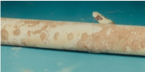
Figure 3.10 — Divot formations along the length of the DuPont PRD-66 filter elements after testing at AEP.
