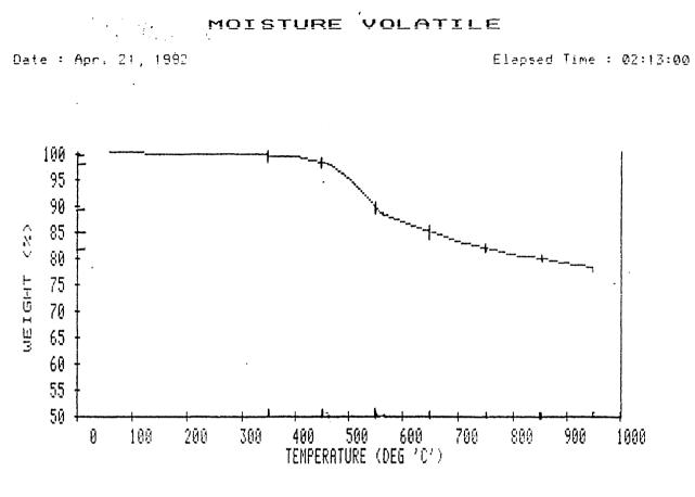
Frn.#1 Cr.# 6 Type:Classification. ID:KNOX CRK- Weight: 0.730 Gram(s) Title : MOISTURE VOLATILE Zero Dev : 10 Max Dev : 5 Mode/ Step End ATM Node. Nec Cyn Ramp Rate Final Timeout or % Deviation Mode Temp. 106 °C - B/N2 950 °C - B/N2 99 D/M Cnst Wgt Timeout 0,05 % 7 Nin 11 <u>-</u> t QFF Vol. ON 10 D/M
